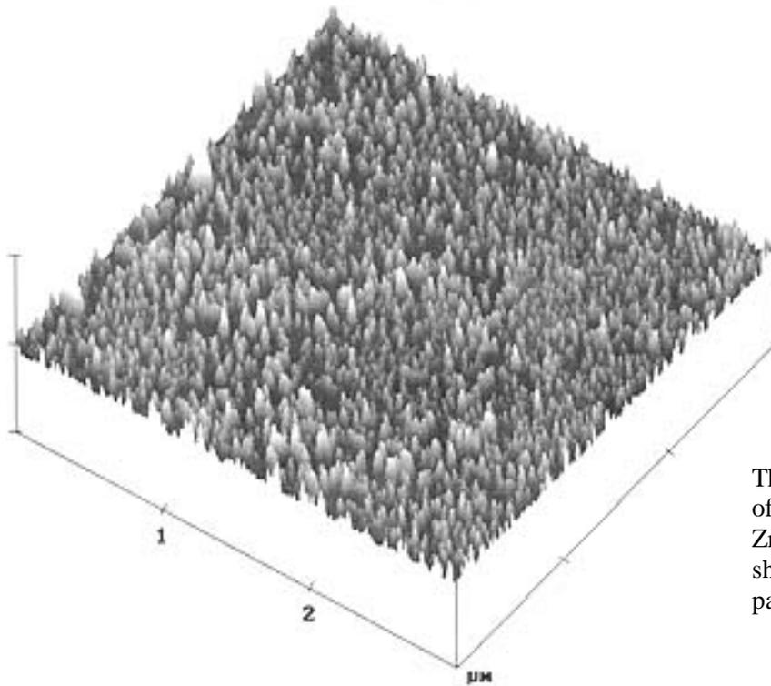
Three-dimensional image of 2 bilayers of ZrO<sub>2</sub>/polymer films, showing more closely packed layers of particles
