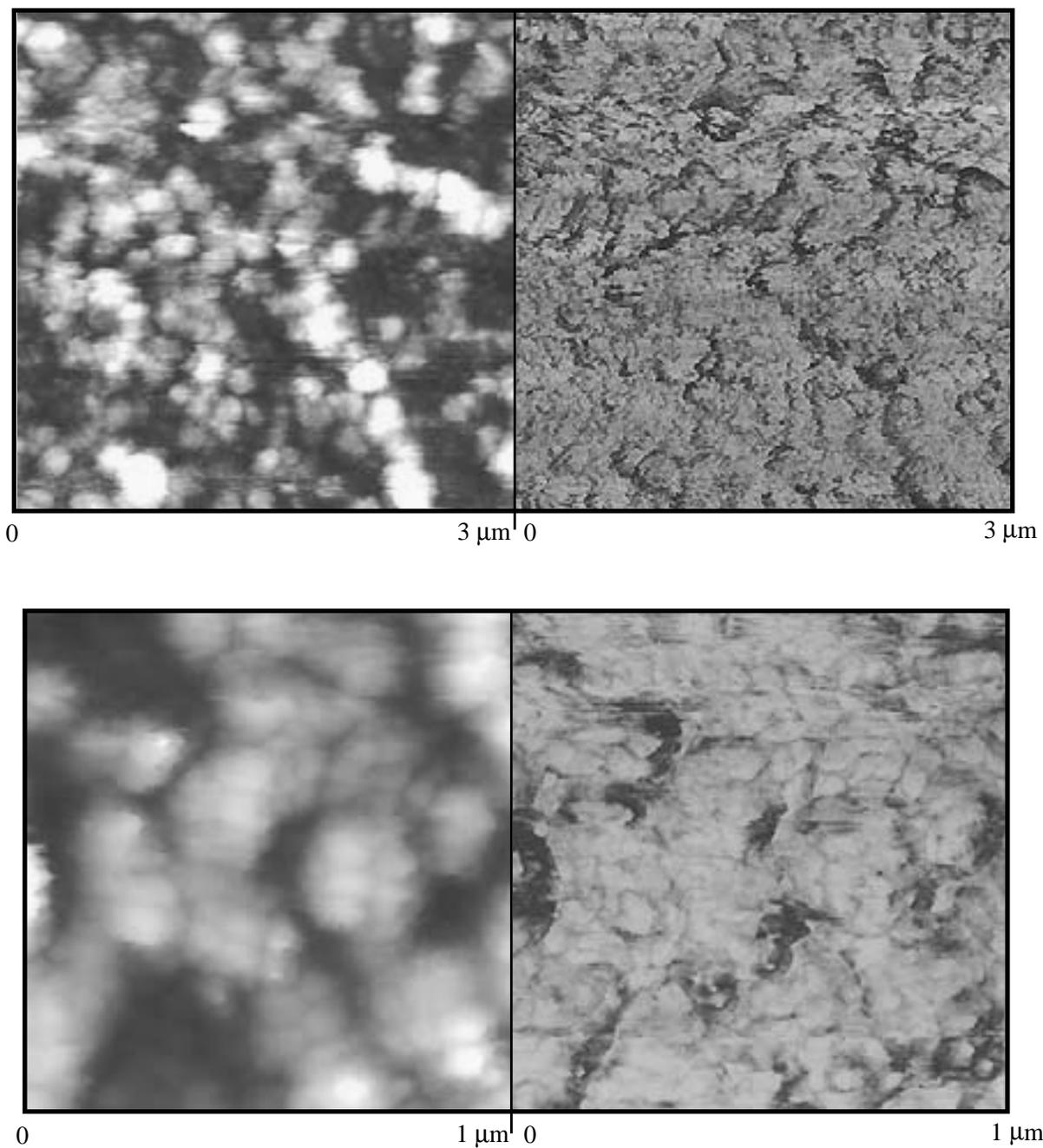
**Figure 4.21. AFM images after the adhesion test showing distorted particles on the coating surface.**
