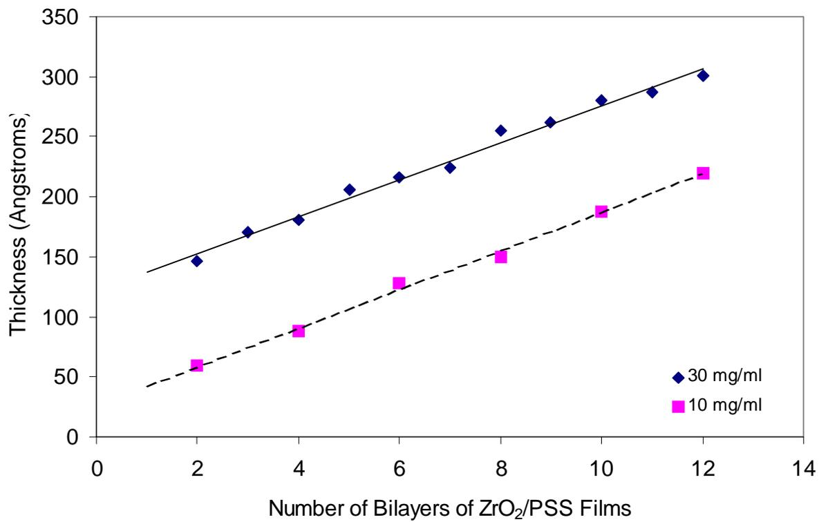
Figure 4.18. Thickness dependence of the ZrO<sub>2</sub> concentrations.
