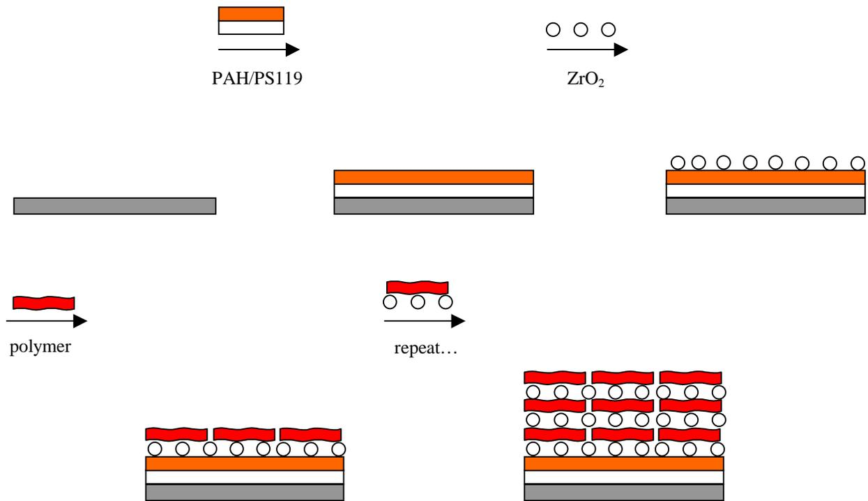
**Figure 4.3. Schematic representation of multilayer fabrication of ZrO<sub>2</sub>/polymer nanocomposite thin-film coatings.**
