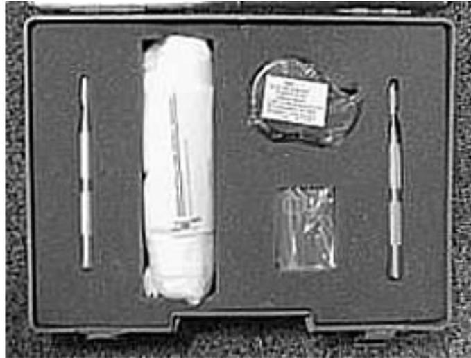
**Figure 4.4. Adhesion and abrasion testing apparatus.**
