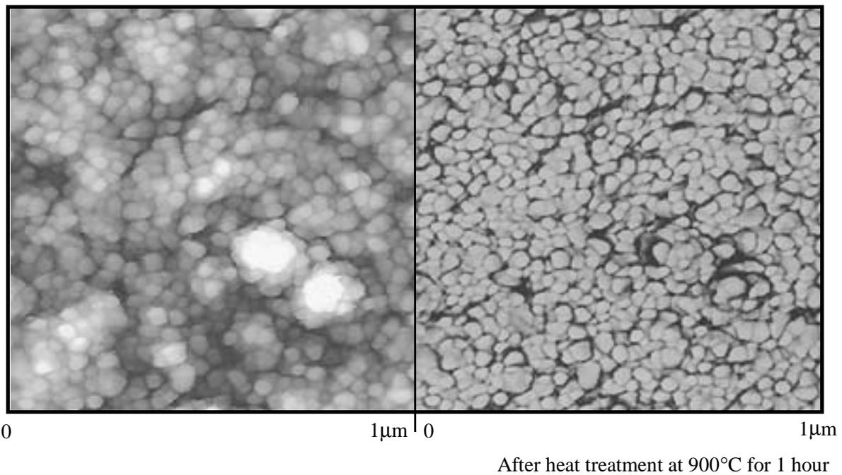
**Figure 4.16. AFM images of ZrO<sub>2</sub>/polymer coating surface. The structure consists of 200 bilayers of films; ZrO<sub>2</sub> = 10 mg/ml.**
