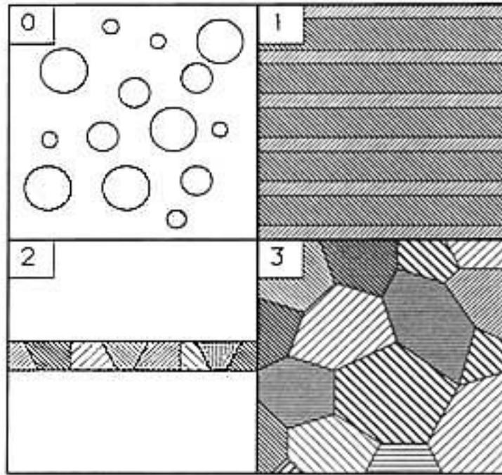
**Figure 2.1.** The schematic diagrams of the four types of nanophase materials, classified according to integral modulation dimensionality, from zero, in a, to three, in d. a: Clusters of any aspect ratio from 1 to infinity. b: Multilayers. c: Ultrafine-grained overlayers, coatings, or buried layers. d: Nanophase materials [10].
