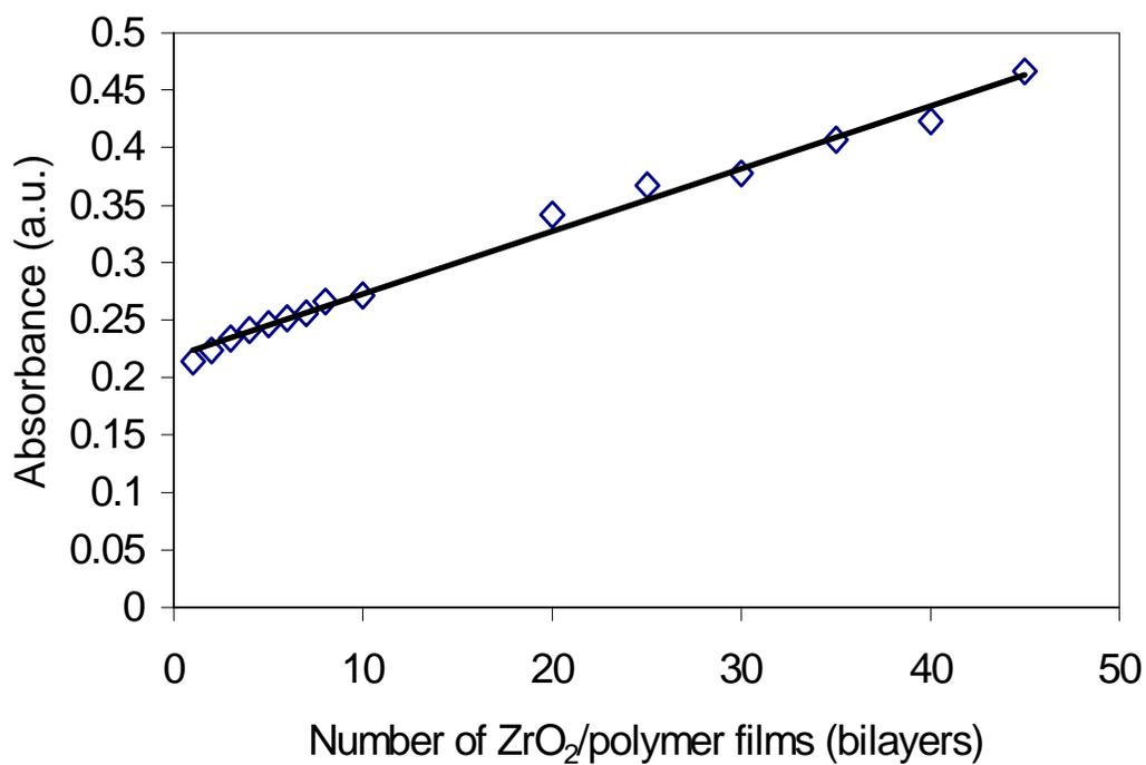
**Figure 4.7.** Dependence of optical absorbance of the ZrO<sub>2</sub>/polymer multilayer film on the number of deposited bilayers (at 225 nm).
