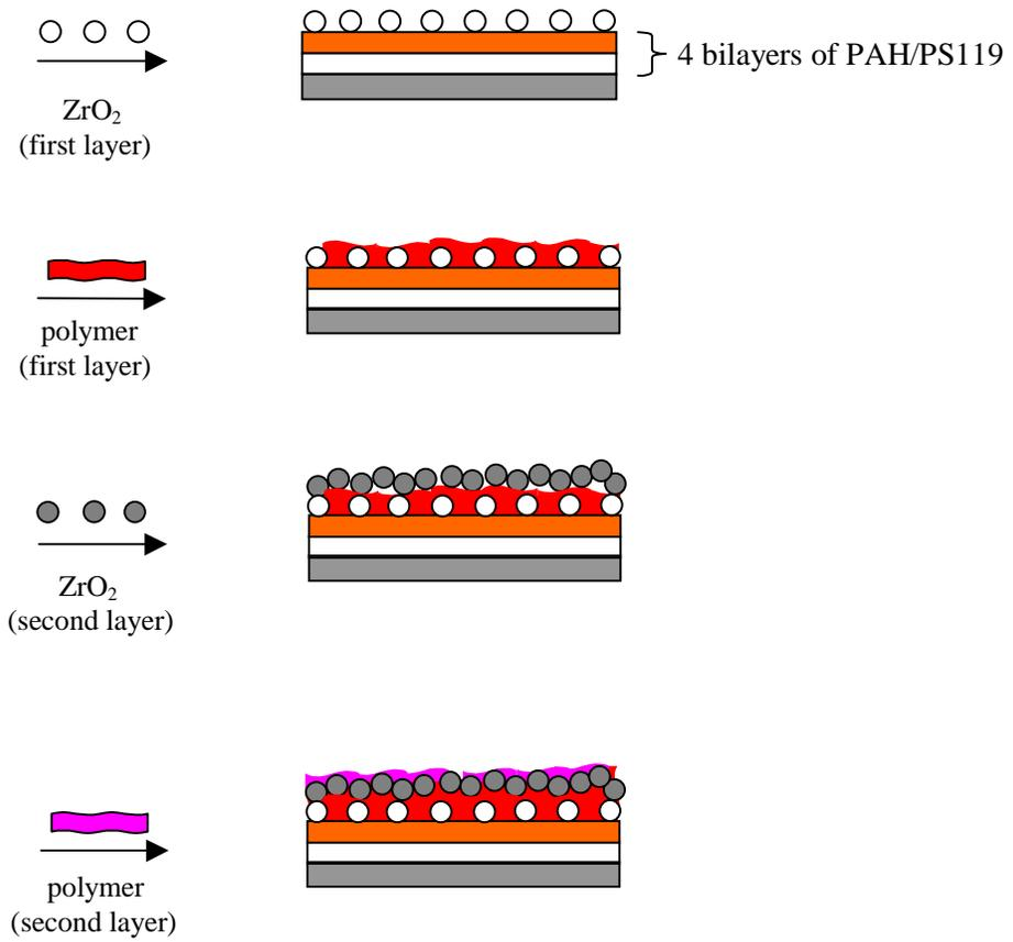
**Figure 4. 14. The ISAM fabrication method of  $ZrO_2$ /polymer nanocomposites showing the formation of bumpy surfaces.**
