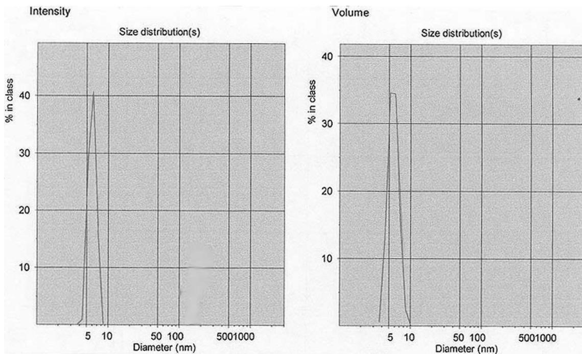
**Figure 4.13. Particle size distributions of ZrO<sub>2</sub> colloidal system.**
