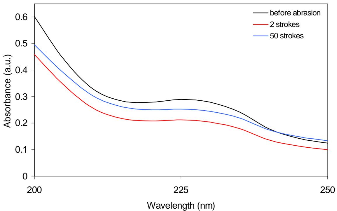
**Figure 4.22.** UV/Vis spectrum after the abrasion tests showing a decrease in optical absorption.
