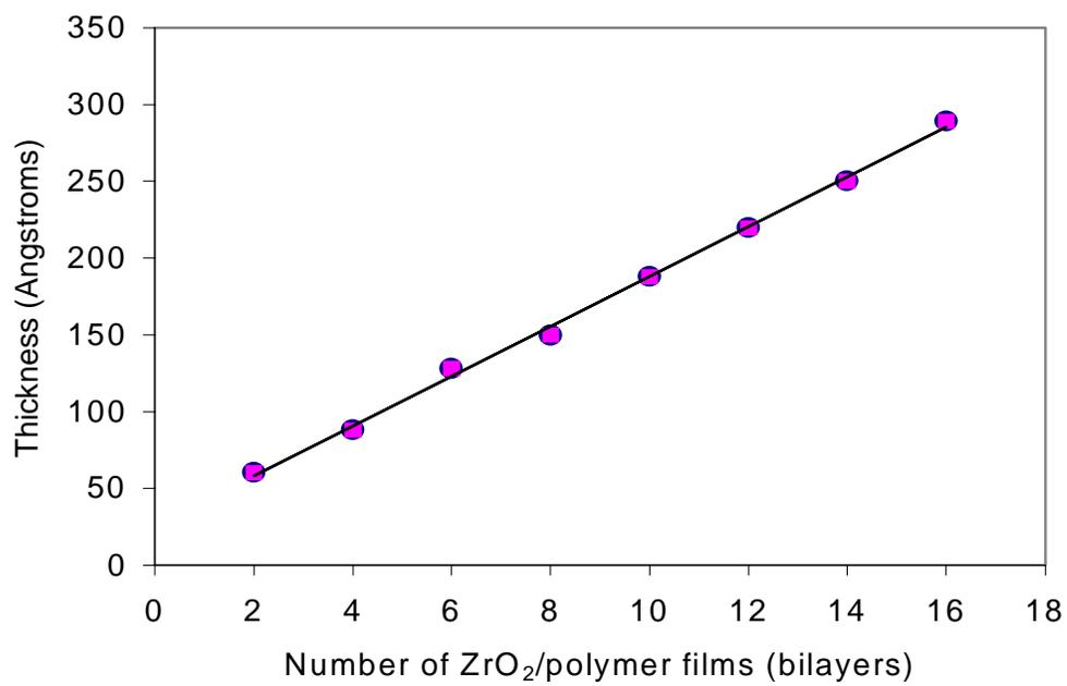
**Figure 4.8.** Dependence of ellipsometric thickness of ZrO<sub>2</sub>/polymer multilayer films on the number of deposited bilayers.
