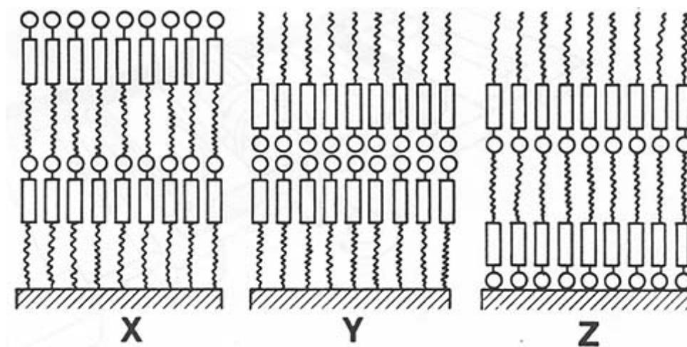
**Figure 3.1.** The common deposition mode for classical LB films is Y-type, where the molecules stack vertically with a head to head and tail to tail configuration. However, X and Z-type depositions are also observed [20].
