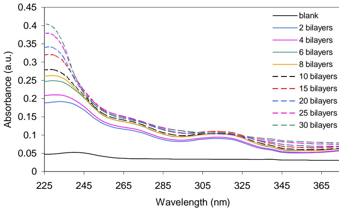
**Figure 4.6.** UV/Vis Spectrum of ZrO<sub>2</sub>/PSS multilayer structure showing an increasing number of bilayers.
