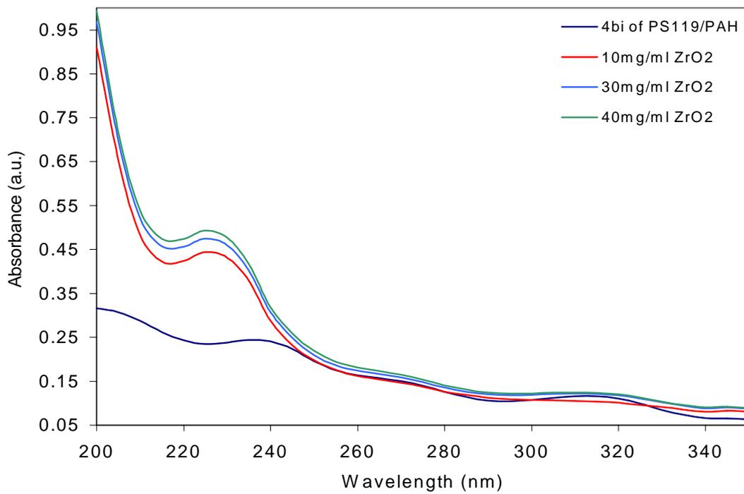
**Figure 4.17. UV/Vis spectra showing increasing optical absorption for different concentrations of ZrO<sub>2</sub> solutions.**
