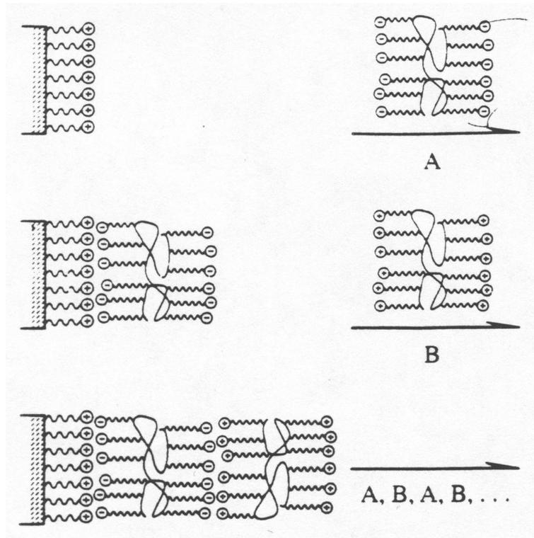
Figure 3.2. Schematic for the buildup of multilayer assemblies by ISAM [4].
