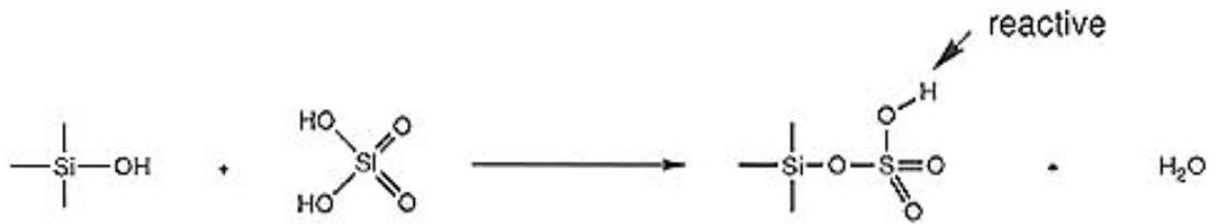
**Figure 4.2. Pre-treatment reaction to modify the surface charge of quartz or silicon substrates.**
