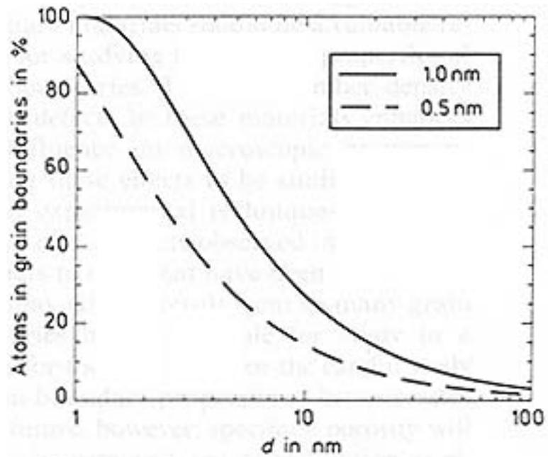
**Figure 2.2.** Range of percentage of atoms in grain boundaries of a nanophase material as a function of grain diameter, assuming that the average grain boundary thickness ranges from 0.5 to 1.0 nm (ca 2 to 4 atomic planes wide) [10].
