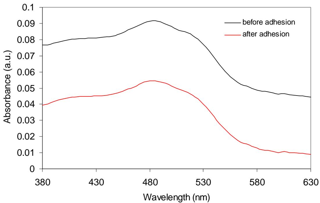
**Figure 4.20. UV/Vis spectrum after the adhesion test showing a decrease of optical absorption.**
