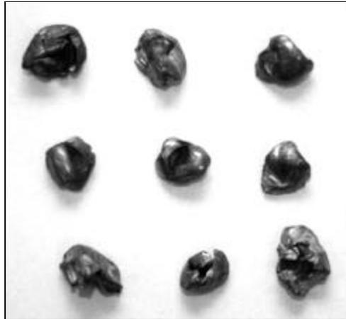
**Figure 4.6: Various deformed projectiles after specimen penetration.**
