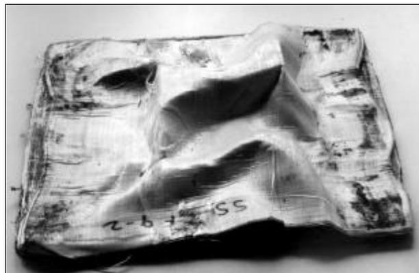
Figure 4.19: The post impact inspection of a specimen containing nine ECPE layers showed large deformation in the ECPE, which contributed to the significant improvement in energy absorption capabilities.
