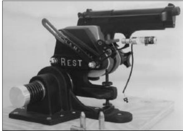
**Figure 3.6: The 9mm handgun was mounted and a laser sight was used to provide maximum accuracy.**
