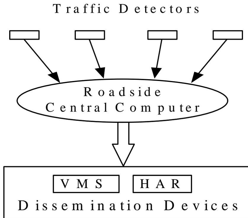
**Figure 8. Typical system architecture for a real-time advanced warning and traffic control system**
