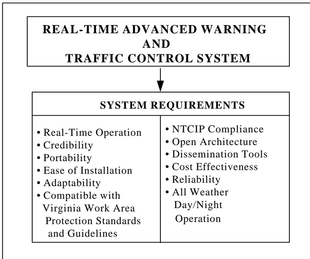
**Figure 12. System Requirements for the Real-Time Work Zone System**
