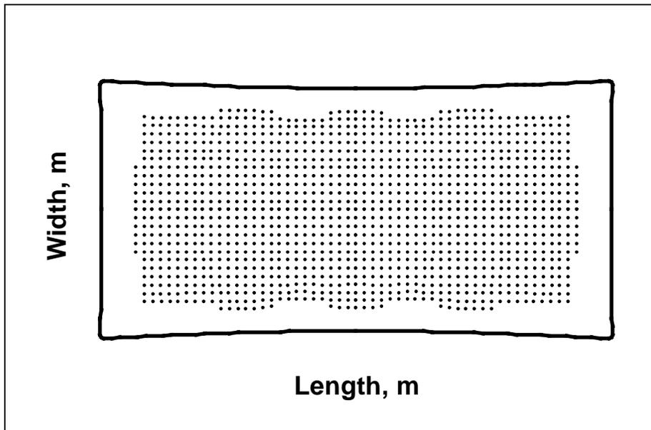
Figure 3.3.2.2: Whole Contact Region at a Pressure Head of 0.69m for  $K_d = 8.40 \times 10^4$   $\text{N/m}^3$  and  $L_f:W_f$  of 2:1
