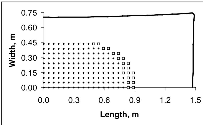
Figure 3.2.2.1: Quarter Contact Region at Pressure Heads of 0.5m and 0.79m for  $K_d = 4.20 \times 10^6 \text{ N/m}^3$  and  $L_f:W_f$  of 2:1; circle: 0.5m and 0.79m, square: 0.5m
