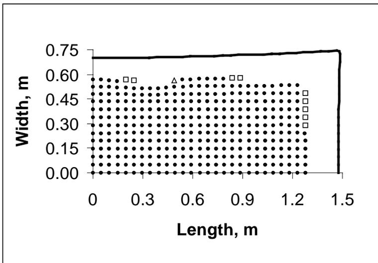
Figure 3.3.2.1: Quarter Contact Region at Pressure Heads of 0.5m and 0.69m for  $K_d = 8.40 \times 10^4 \text{ N/m}^3$  and  $L_f:W_f$  of 2:1; circle: 0.5m and 0.69m, square: 0.5m, triangle: 0.69m
