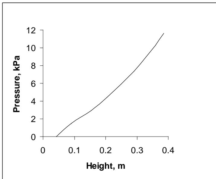
Figure 3.2.4.1: Pressure vs. Height for  $K_d = 4.20 \times 10^6 \text{ N/m}^3$  and  $L_f:W_f$  of 2:1
