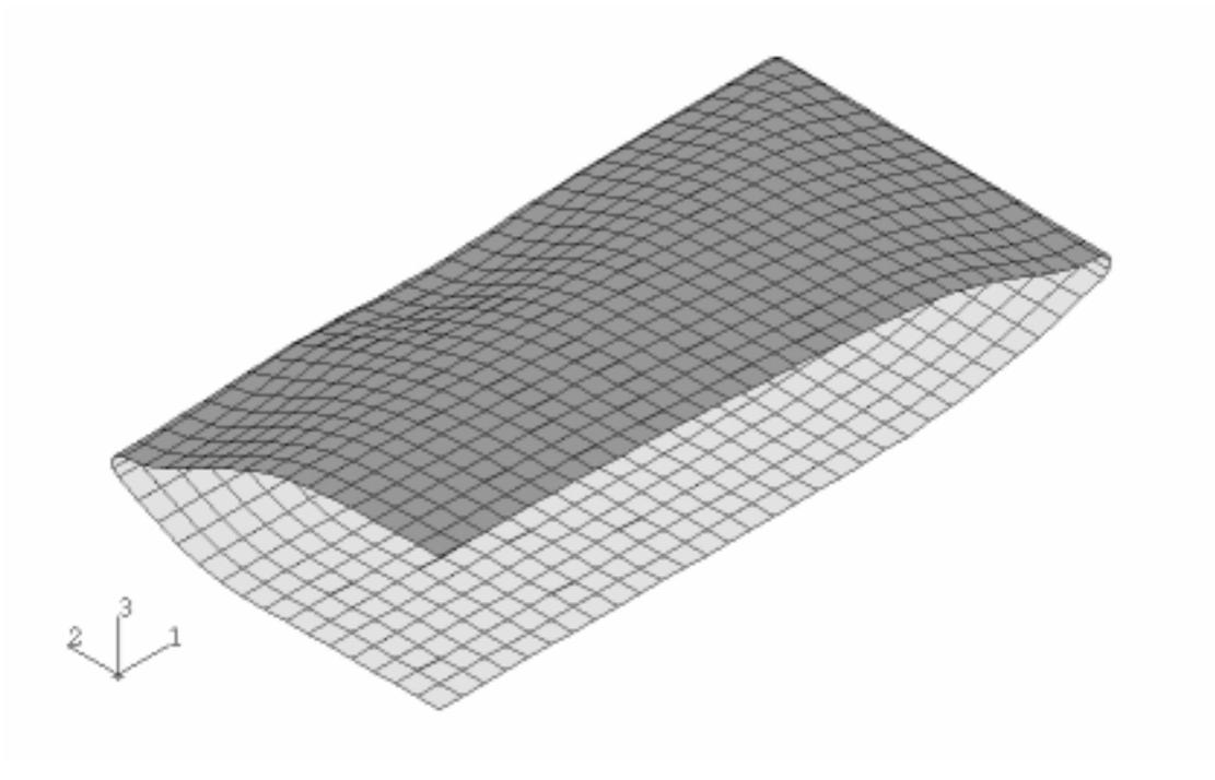
Figure 3.2.1.1: Pressure Head of 0.5m for  $K_d = 4.20 \times 10^6 \text{ N/m}^3$  and  $L_f:W_f$  of 2:1
