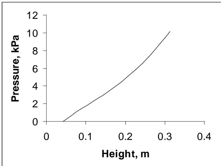
Figure 3.3.4.1: Pressure vs. Height for  $K_d = 8.40 \times 10^4 \text{ N/m}^3$  and  $L_f:W_f$  of 2:1
