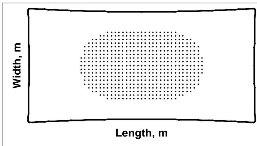
Figure 3.2.2.2: Whole Contact Region at a Pressure Head of 0.79m for  $K_d = 4.20 \times 10^6 \text{ N/m}^3$  and  $L_f:W_f$  of 2:1
