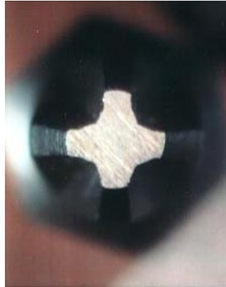
Figure 4.9 New Bit, Sectioned to 30-Thousandths
