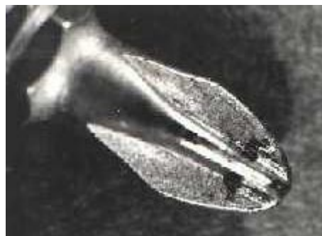
Figure 4.2 Bit B Black & Decker Scorpion Bit after 5000 Cycles on Dixon Rig
