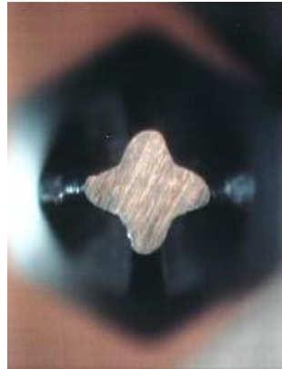
Figure 4.10 Fully Worn Bit, Sectioned to 30-Thousandths
