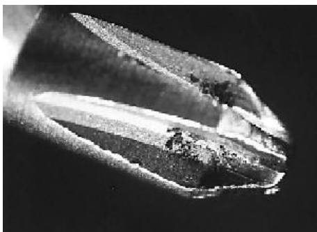
Figure 4.1 Bit A Grabber #2 Reduced Bit after 2500 Cycles on Dixon Rig
