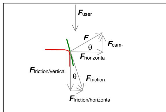
**Figure 5.12 Complete Force Balance**
