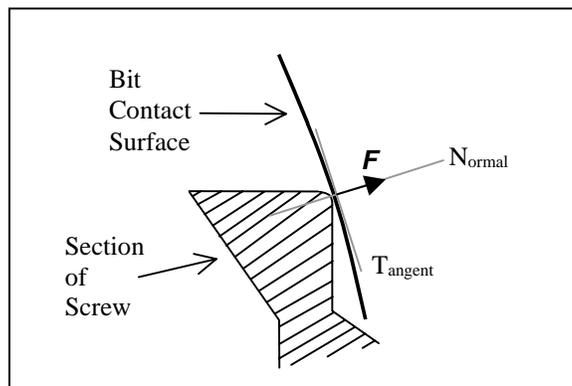
**Figure 6.1 Bit/Screw Interaction for Current Bit**
