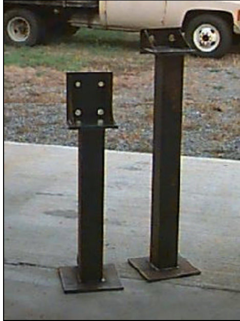
Figure 4.15 Stands for Supporting the Cab During the Installation of the Base Mounts
