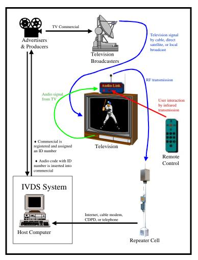
Figure 1.1 IVDS System Diagram
