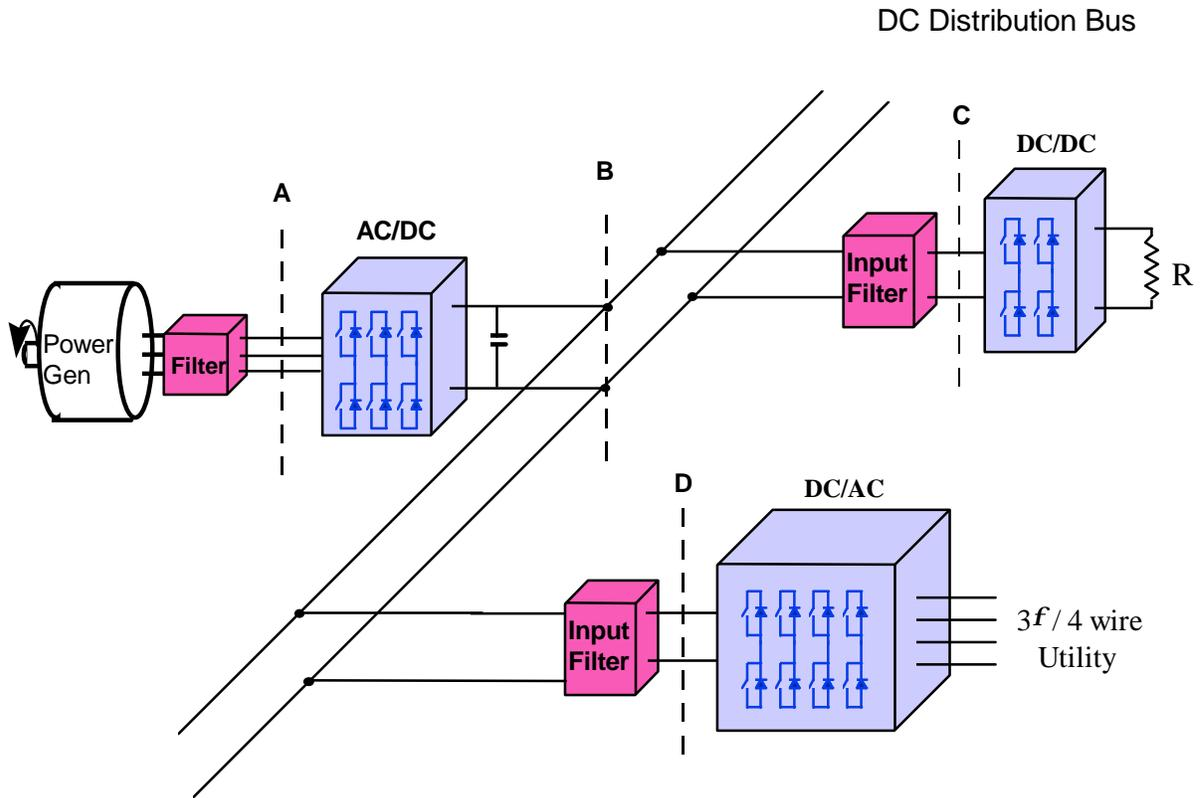
**Figure 1.2 : PEBB based DC Distribution Power System (DPS) :** *The DPS comprises of a front-end Boost Rectifier feeding the DC link. Various loads connected to the DC link include a three phase Four Leg Inverter and a DC-DC Converter.*
