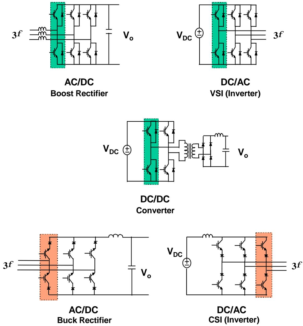
**Figure 1.1 : Identification of a PEBB Switching Cell :** *The commonality in the power converters is represented as the shaded block. In this thesis, the darkly shaded block is chosen as a PEBB.*
