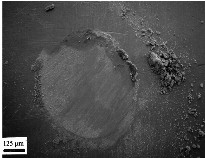
Figure 4.29 SEM micrograph of wear scar on steel ball developed after sliding against glaze A coated \text{Si}_3\text{N}_4 flat
