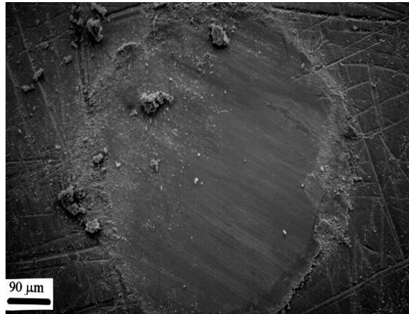
Figure 4.36 SEM micrograph of wear scar on steel ball developed after sliding against glaze B coated \text{Si}_3\text{N}_4 flat
