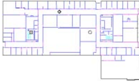
Figure 4.4: Building layout with a base station antenna, represented by a circle, and an interference source antenna, represented by a diamond, having been placed on the current floor. Another base station antenna, represented by a circle that has been crossed out, has been positioned on some other floor of the building.
