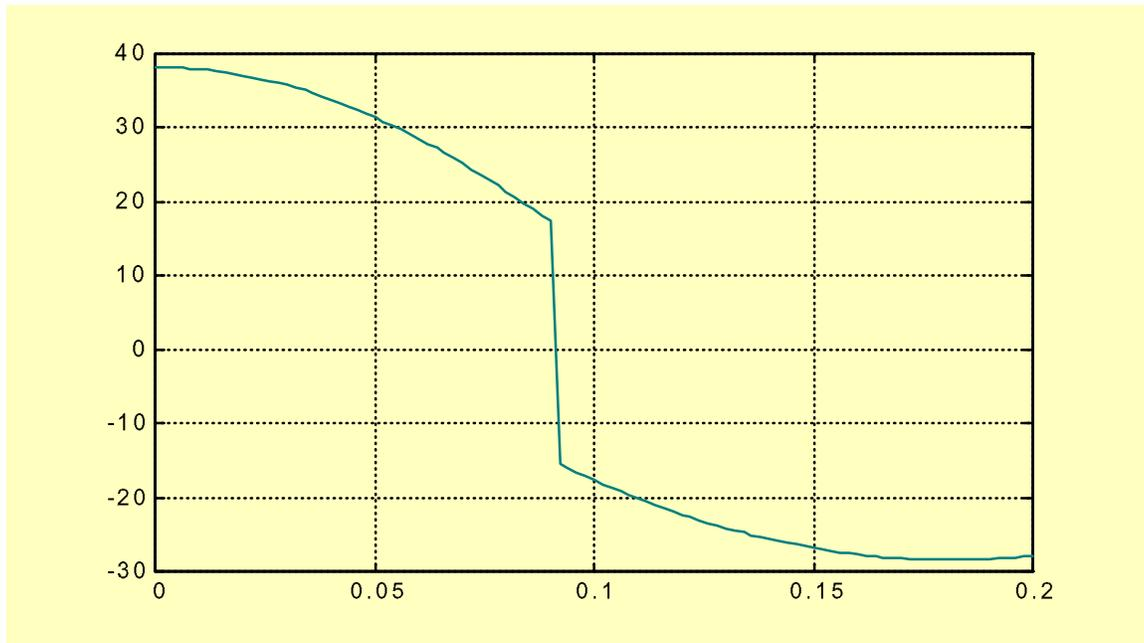
**Figure 3.3:** Acceleration of generator 1 ( $\text{rad.s}^{-2}$ ) versus time:  $t_{cl}=0.09\text{sec}$
