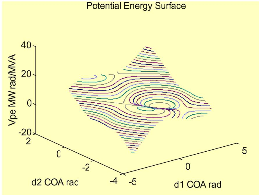
**Figure 3.1:** 3-Machine Potential Energy Surface
