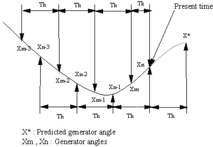
**Figure 4.8 :** Y. Ohura's method of predicting generator angle
