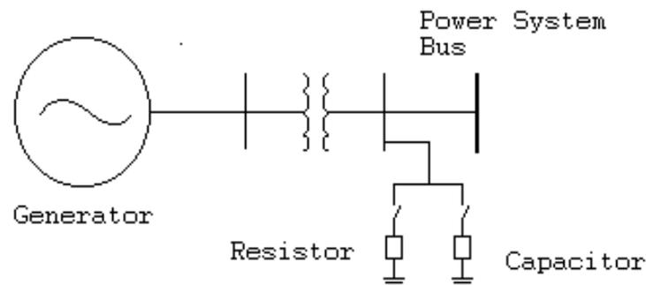
**Figure 6.1:** Braking resistor-capacitor location for a generator
