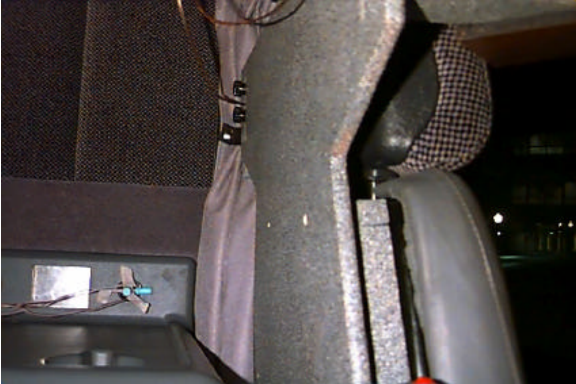
Figure 5.3. Cab Triaxial Mount Accelerometers.
