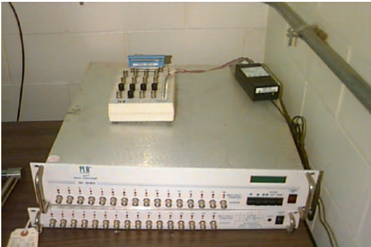
Figure 4.5. PCB Signal Conditioner.
