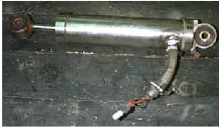
Figure 3.3. A Prototype Twin-Tube Magneto-Rheological Damper.
