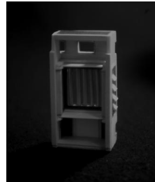
louvers adjusted to receive indirect light
