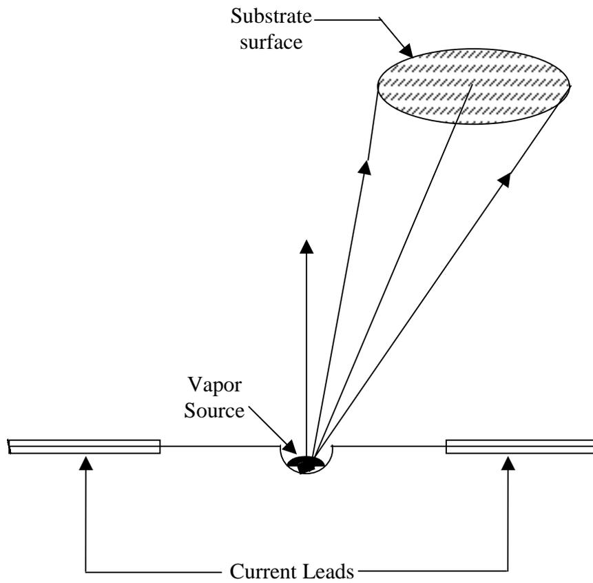
**Figure 4.6 Schematic illustrating vapor deposition.**
