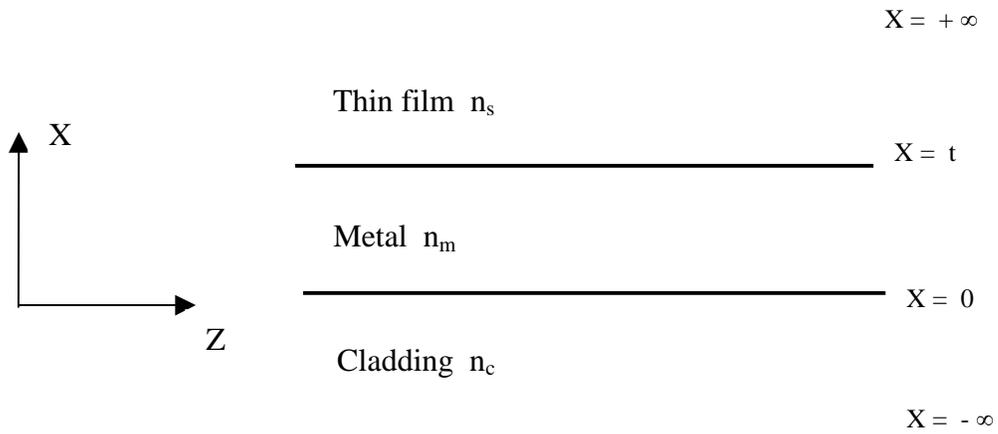
**Figure 3.4 the three-layer fiber surface plasmon configuration<sup>22</sup>.**
