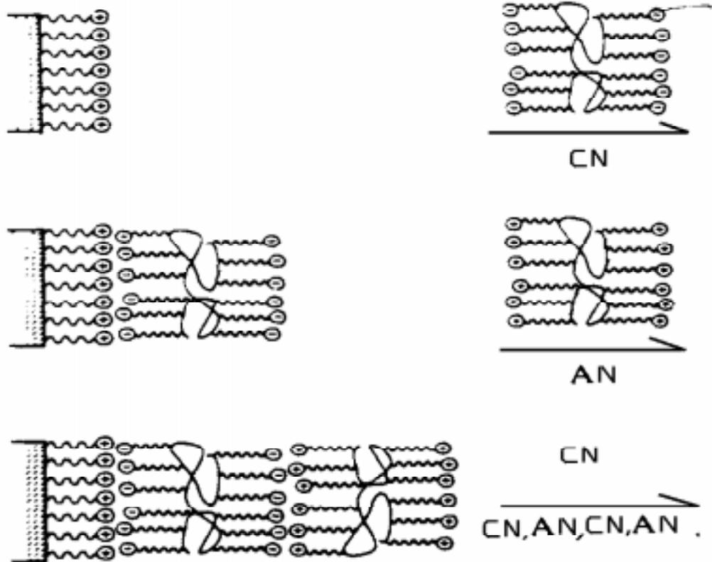
**Figure 3.7 Ionic Self-Assembled Monolayer Method (ISAM), buildup of multilayer assemblies, (AN-anion, CN-cation).**
