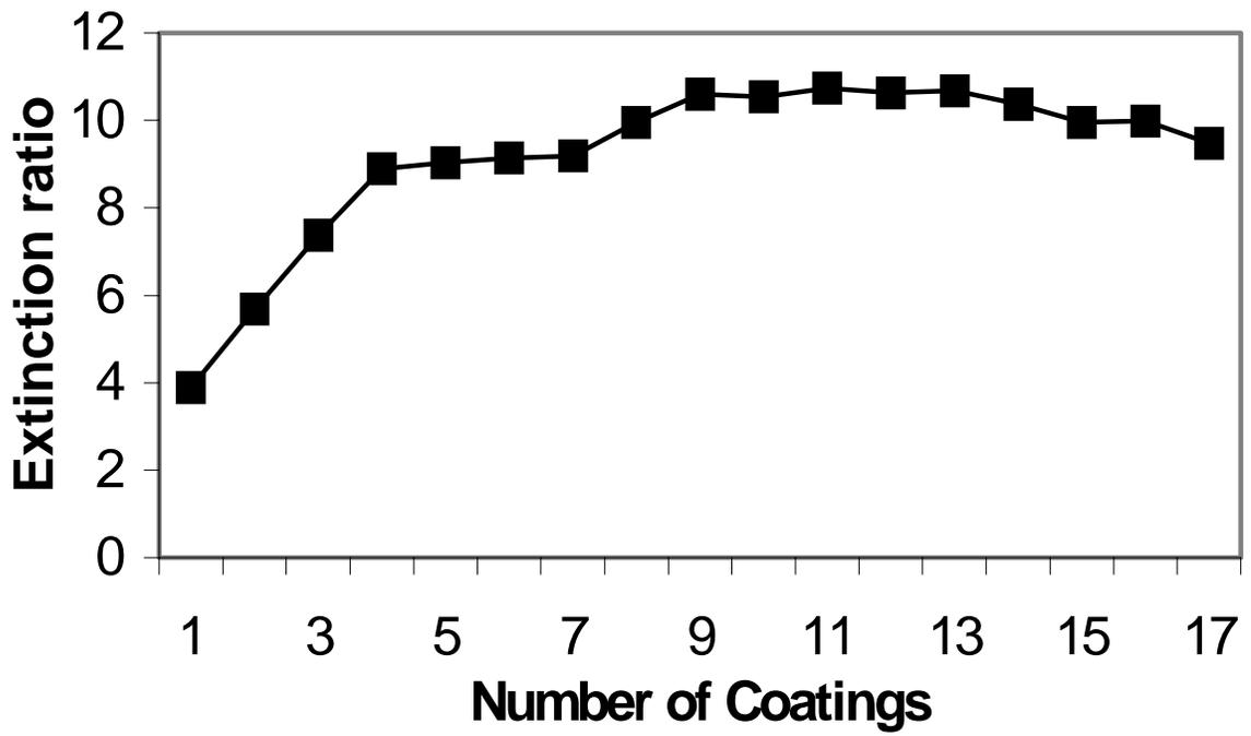
**Figure 4.14.** Extinction ratio of the fiber polarizer.
