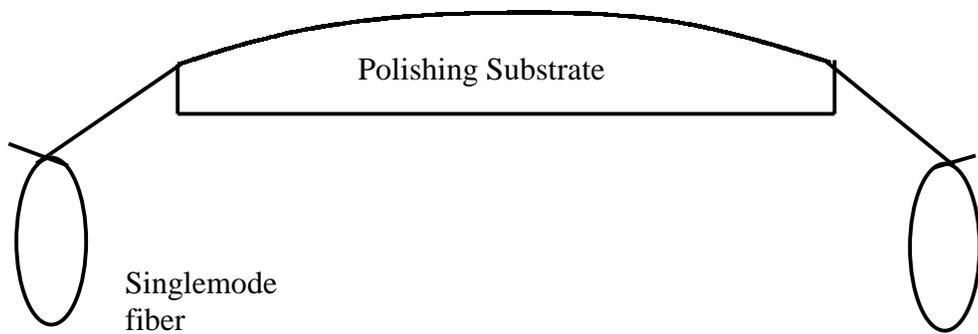
**Figure 4.1 Polishing substrate and configuration of the single mode fiber polarizer.**
