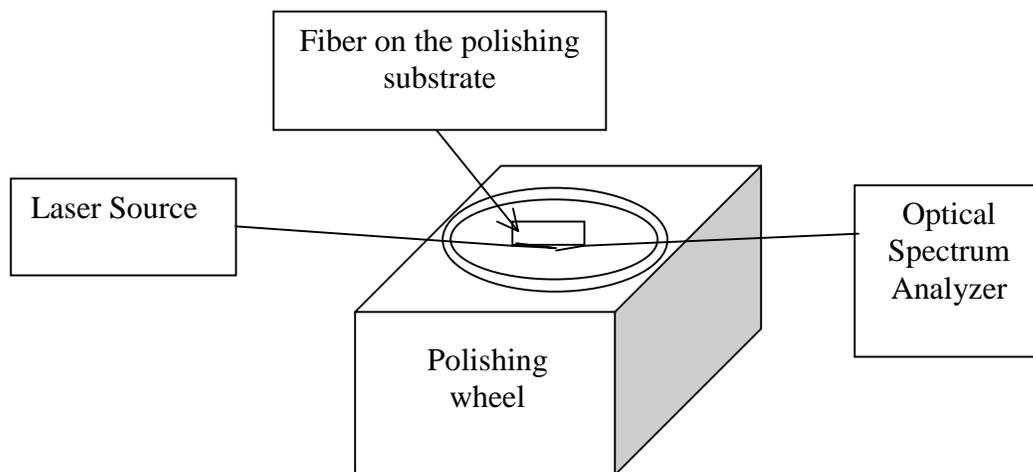
**Figure 4.3 Experimental setup for polishing.**
