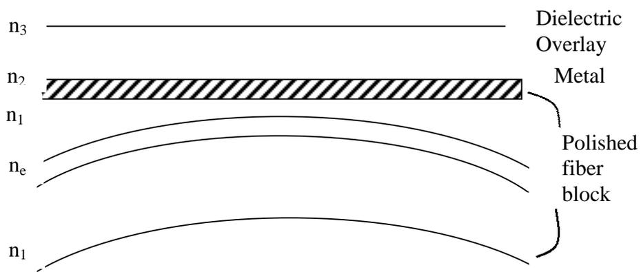
**Figure 3.5 Schematic diagram of the thin metal film plasmon polarizing structure<sup>10</sup>.**
