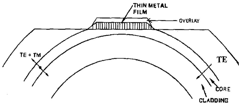
Figure 2.1 Schematic of the fiber polarizer<sup>3</sup>.
