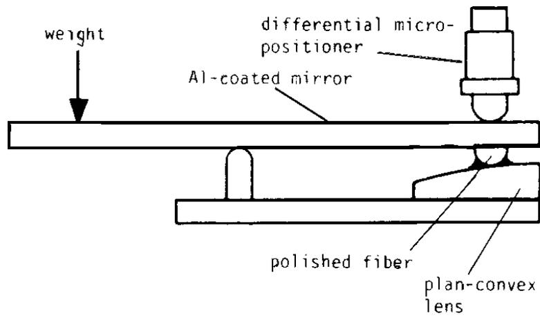
**Figure 2.2 Fiber polarizer with metal-coated mirror and the experimental setup<sup>4</sup>.**
