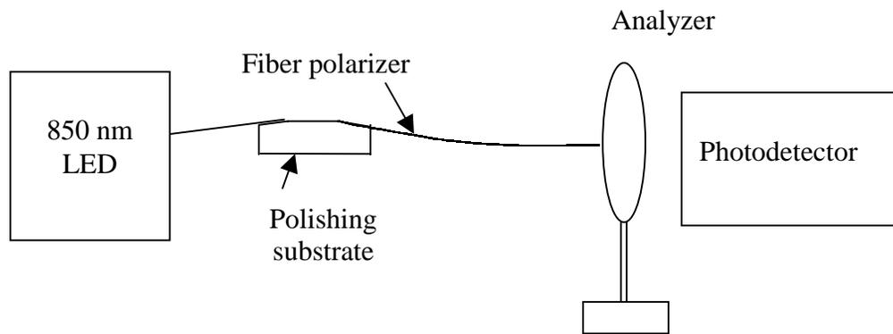
**Figure 4.7** Experimental setup to observe the polarization of light.
