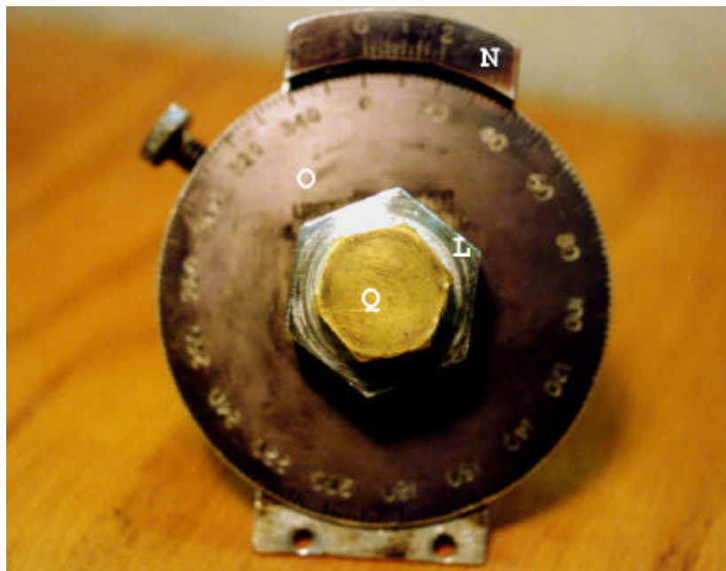
Figure 4.3: Plasma Torch Angle Indicator
