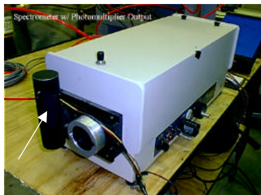
Figure 5.5: Ebert Spectrometer with Burle PMT
