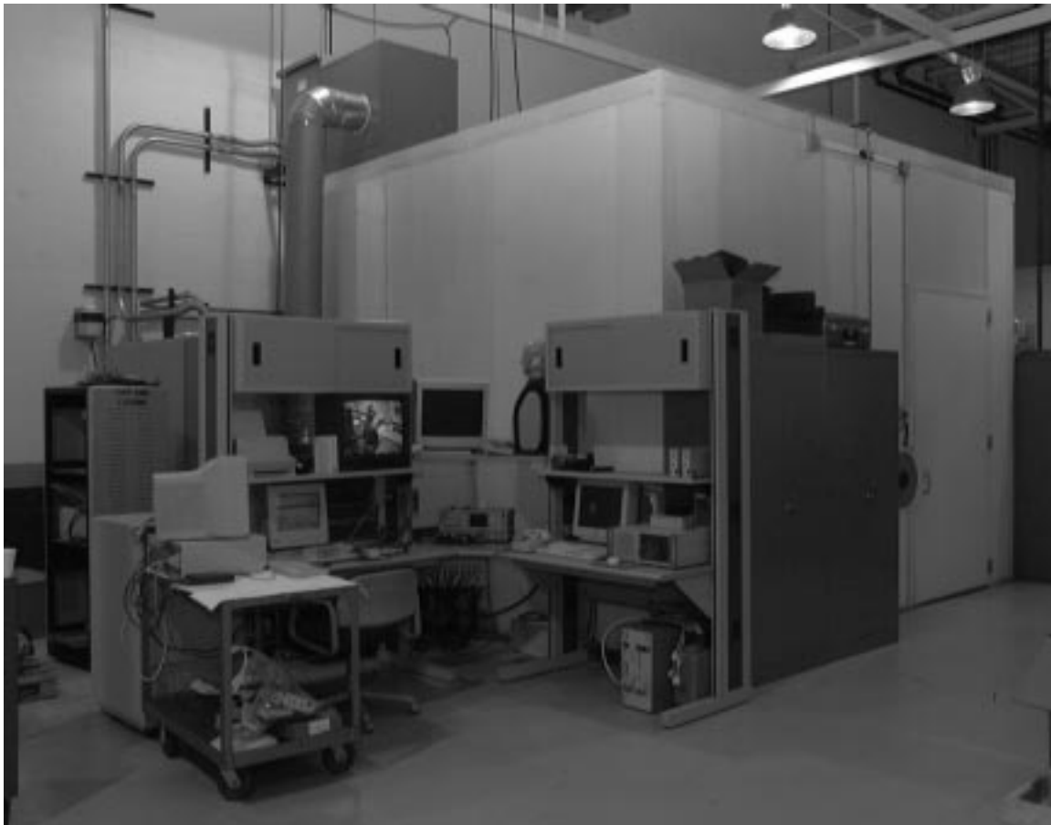
Figure 4.1.1. Hemi-Anechoic Chamber – Exterior
