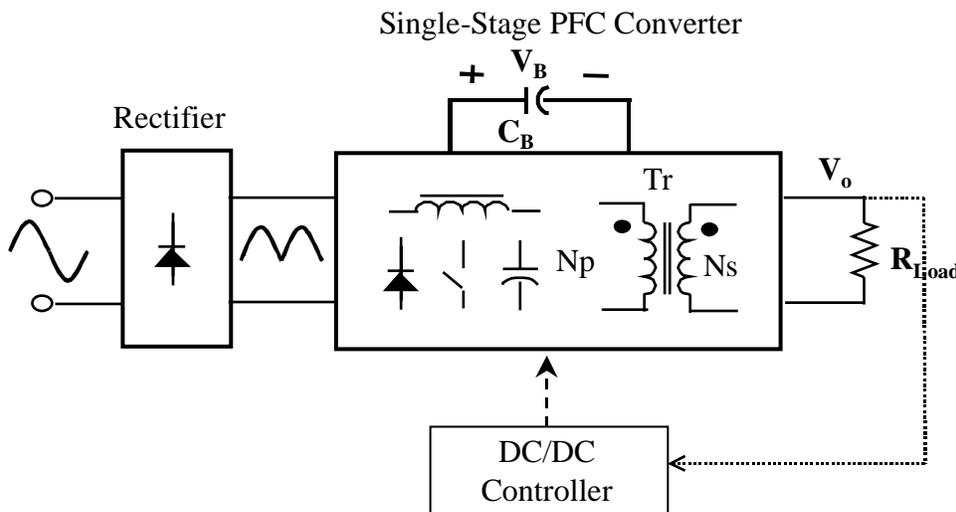
**Figure 4.4 Active Single-Stage PFC Converter**
