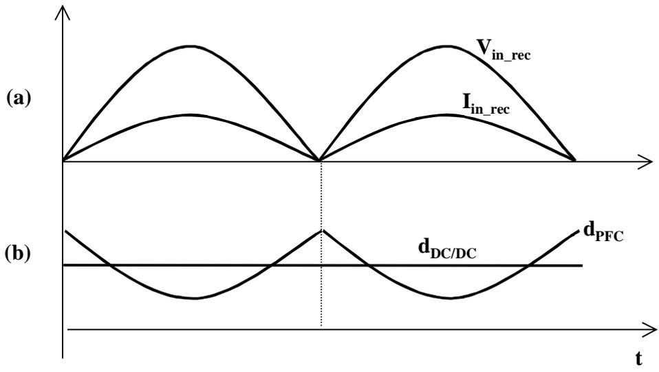
**Fig 4.2 Waveforms of Two-Stage PFC Converter**
