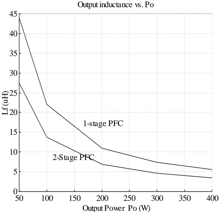
**Figure 4.13 Output filter inductance vs.  $P_o$**
