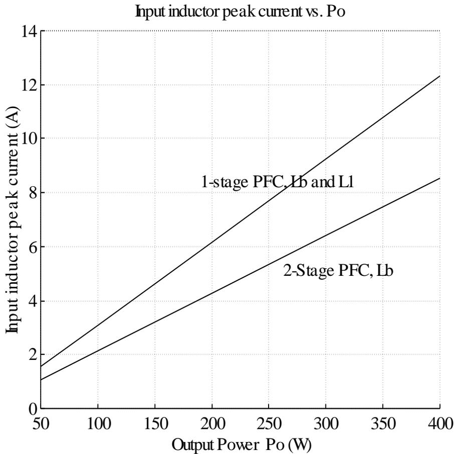
**Figure 4.12 Input inductor peak current vs.  $P_o$**
