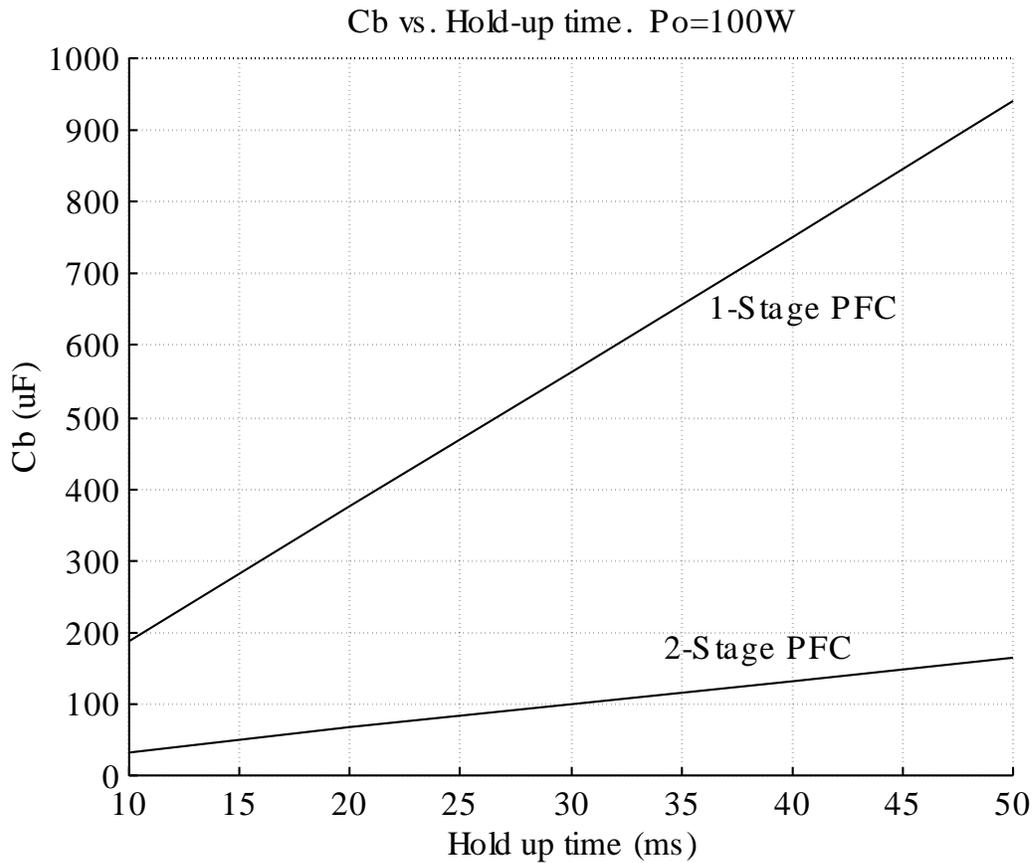
**Figure 4.7  $C_B$  vs. Hold-up time @  $P_o=100$  W**
