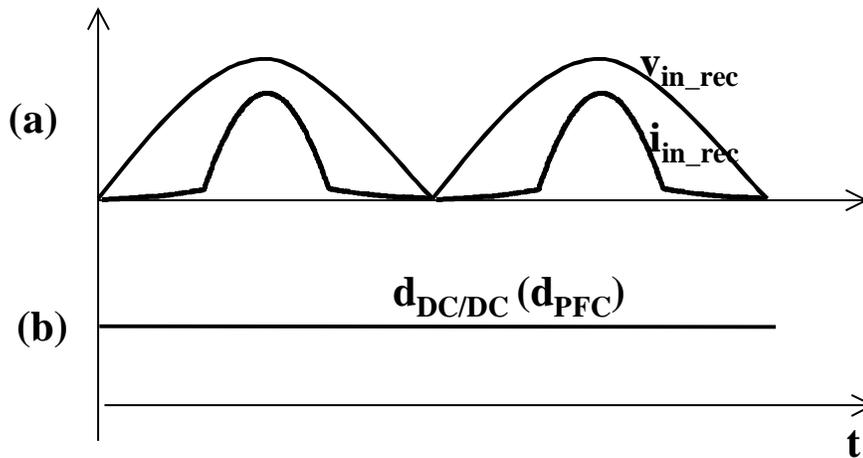
**Fig. 4.6 Waveforms of the Single-Stage PFC Converter**
