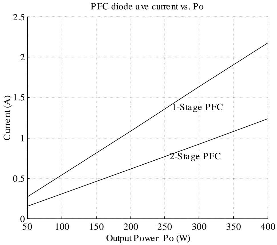
**Figure 4.10 PFC diode average current vs. output power**
