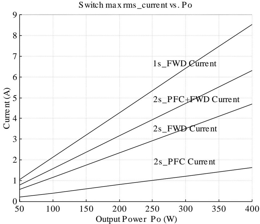
**Figure 4.9 Switch rms current vs. output power**
