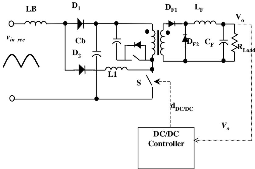
**Fig. 4.5 CCM Single-Stage PFC Converter with ACL Forward Output Stage**
