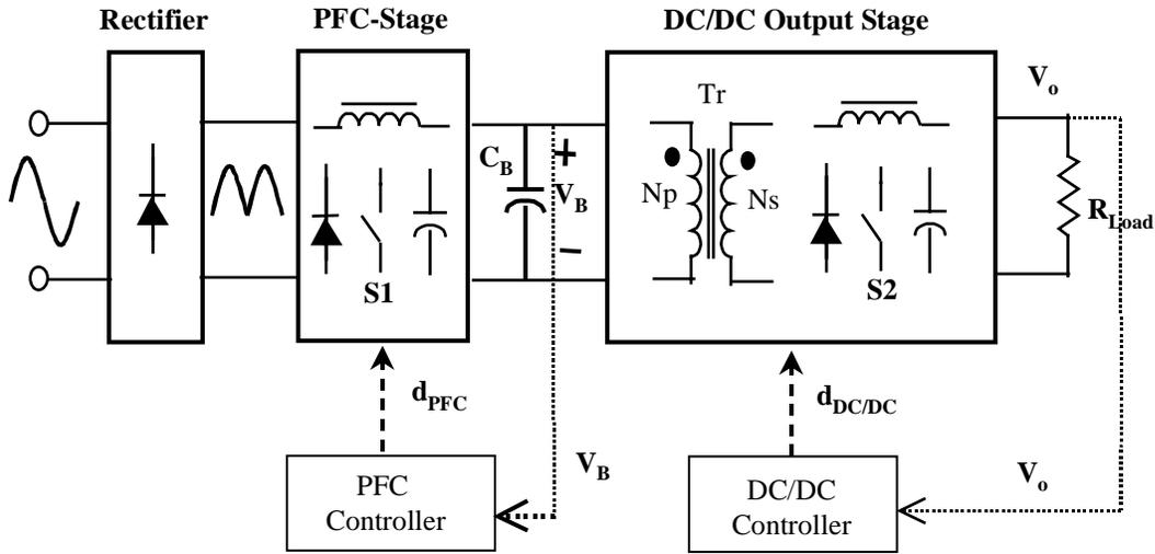
**Figure 4.1 Active Two-Stage PFC Converter**
