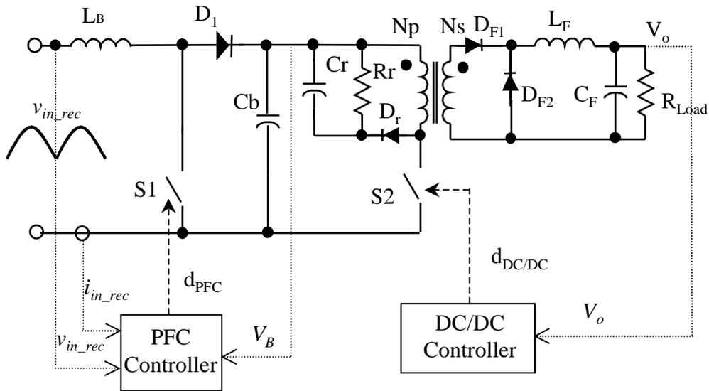
**Figure 4.3 CCM Boost PFC Front-End and RCD Clamped Forward Output Stage**
