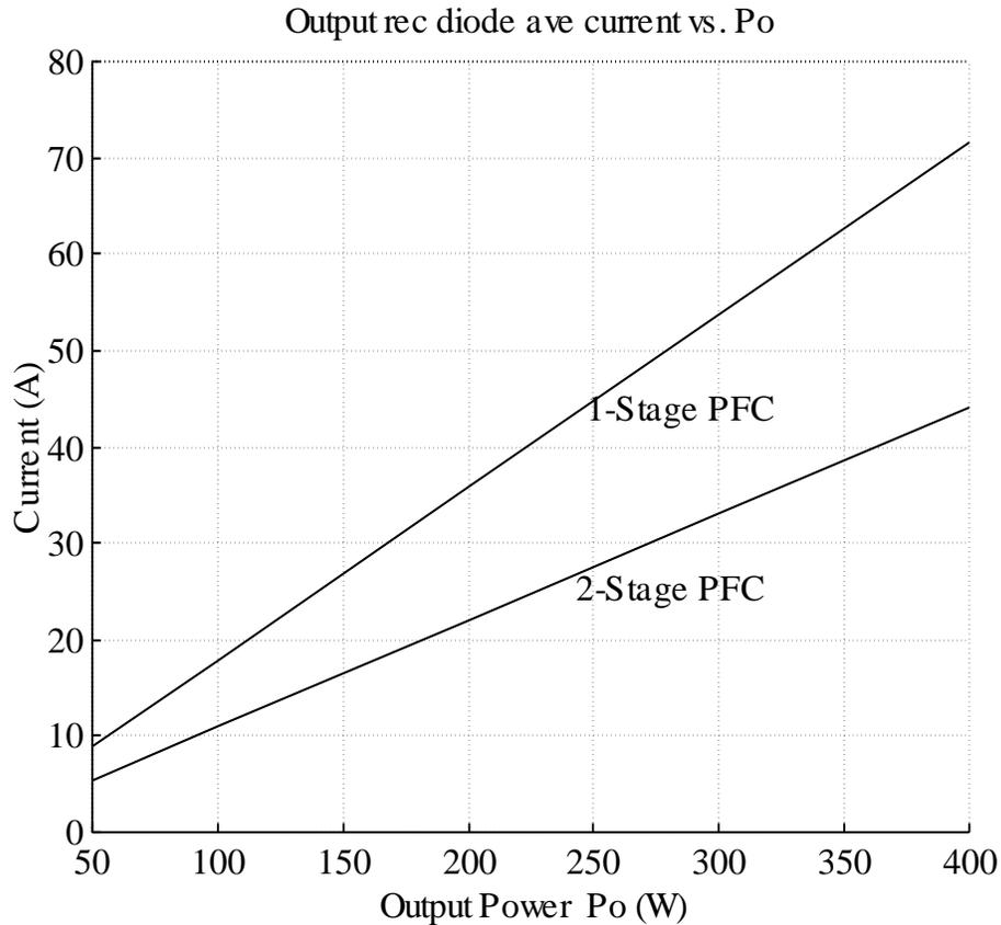
**Figure 4.11 Output rectifier diode current vs.  $P_o$**
