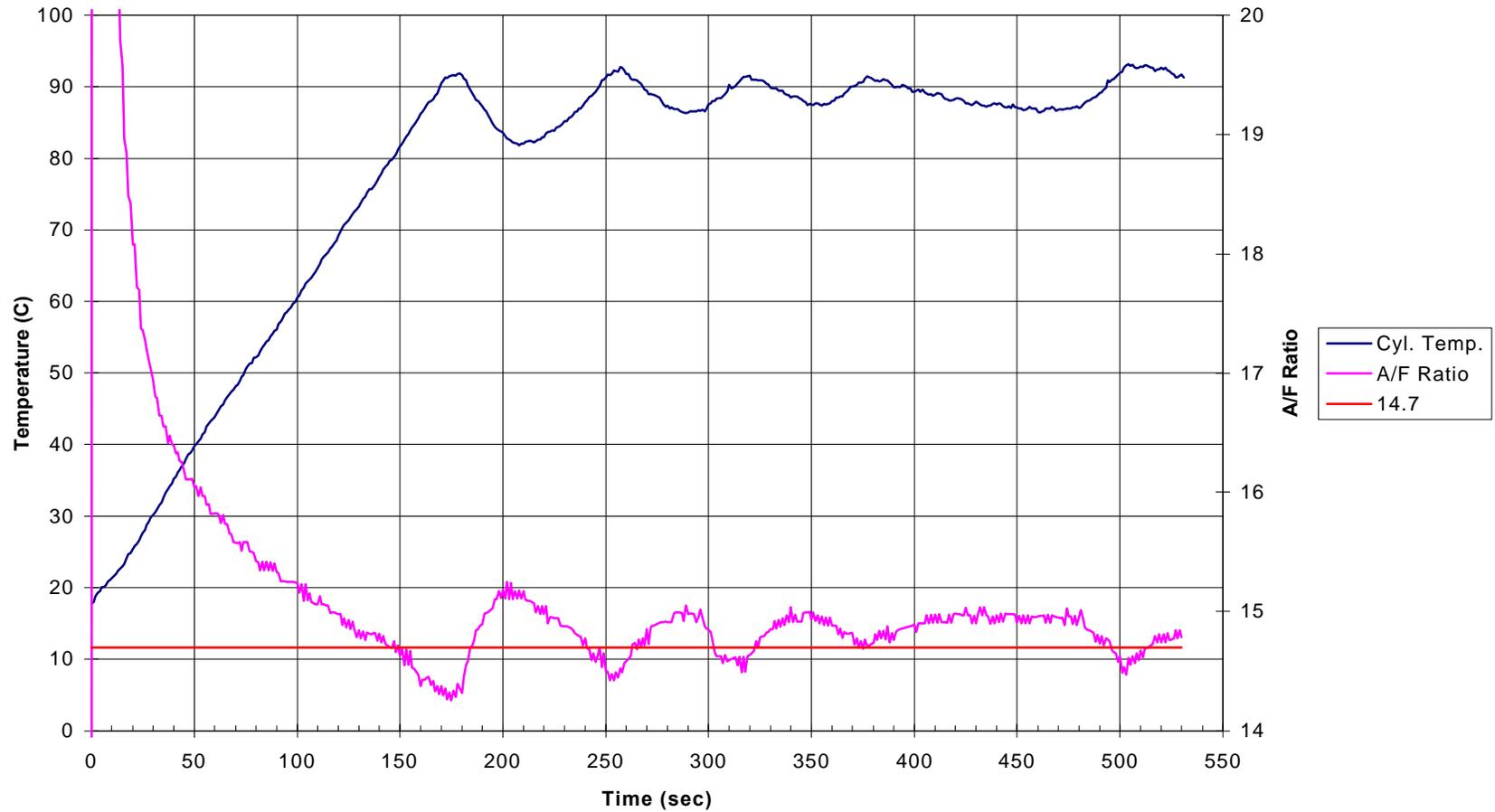
**Figure 4.13 - Cylinder Temperature and Calculated A/F Ratio Versus Time**
