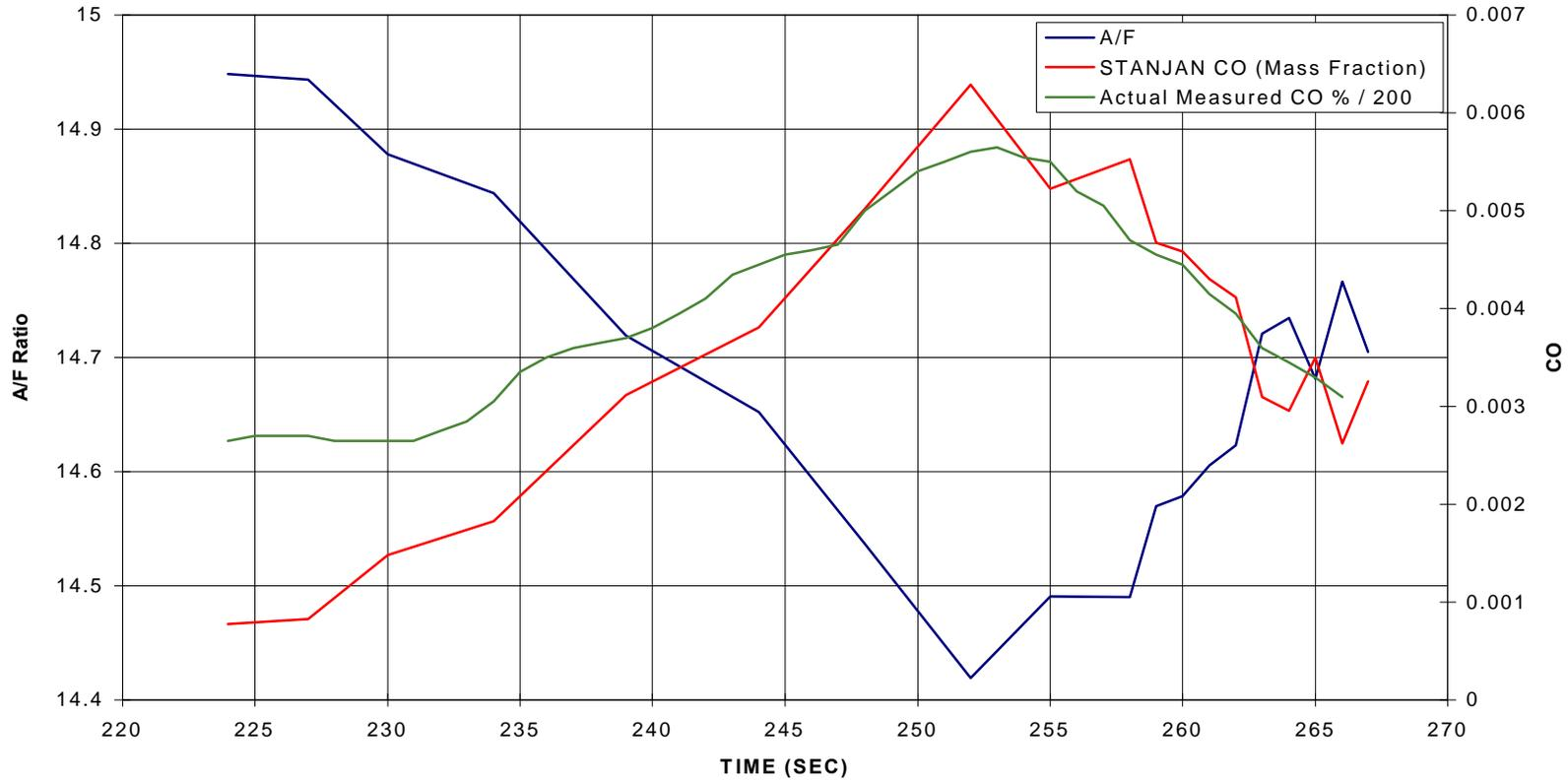
**Figure 4.14 - Comparison of Estimated CO Concentration Changes and Measured CO Concentration Changes For A/F Ratio Fluctuations**
