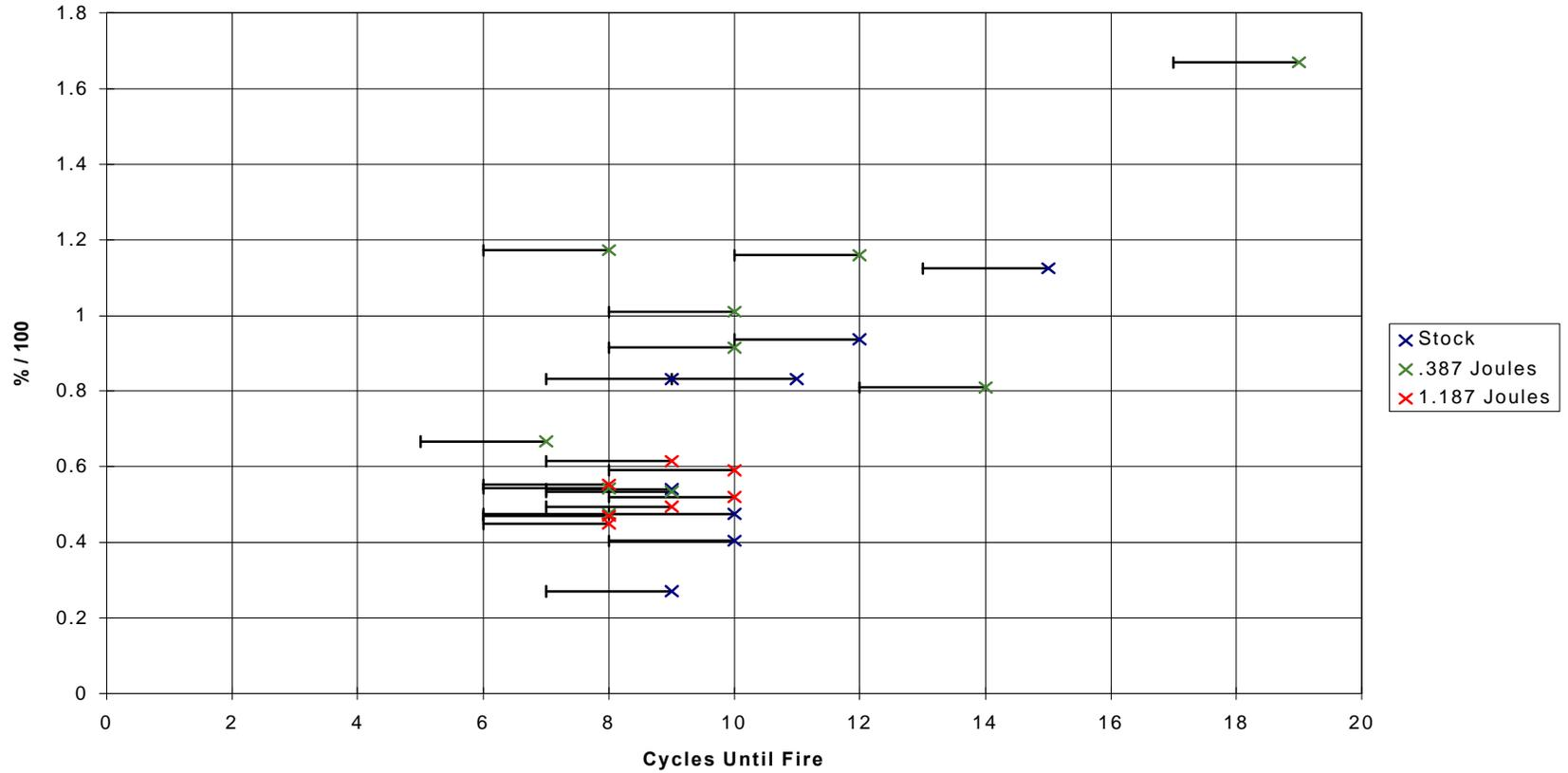
**Figure 4.8 - % Increase in Contribution to Total HCs Produced by Cold Start Vs. Cycles Until Start**
