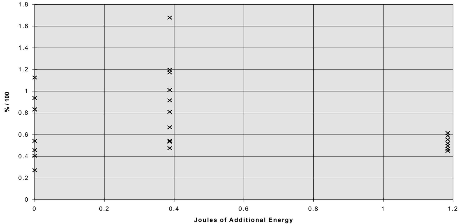
**Figure 4.7 - % Increase in Contribution to Total HCs Produced by Cold Start Vs. Additional Ignition Energy Over Stock**
