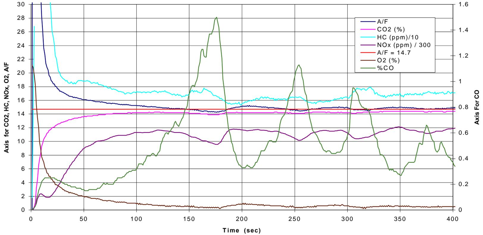
Figure 4.12 - Example Graph of All the Measured Emissions and Calculated A/F Ratio Versus Time
