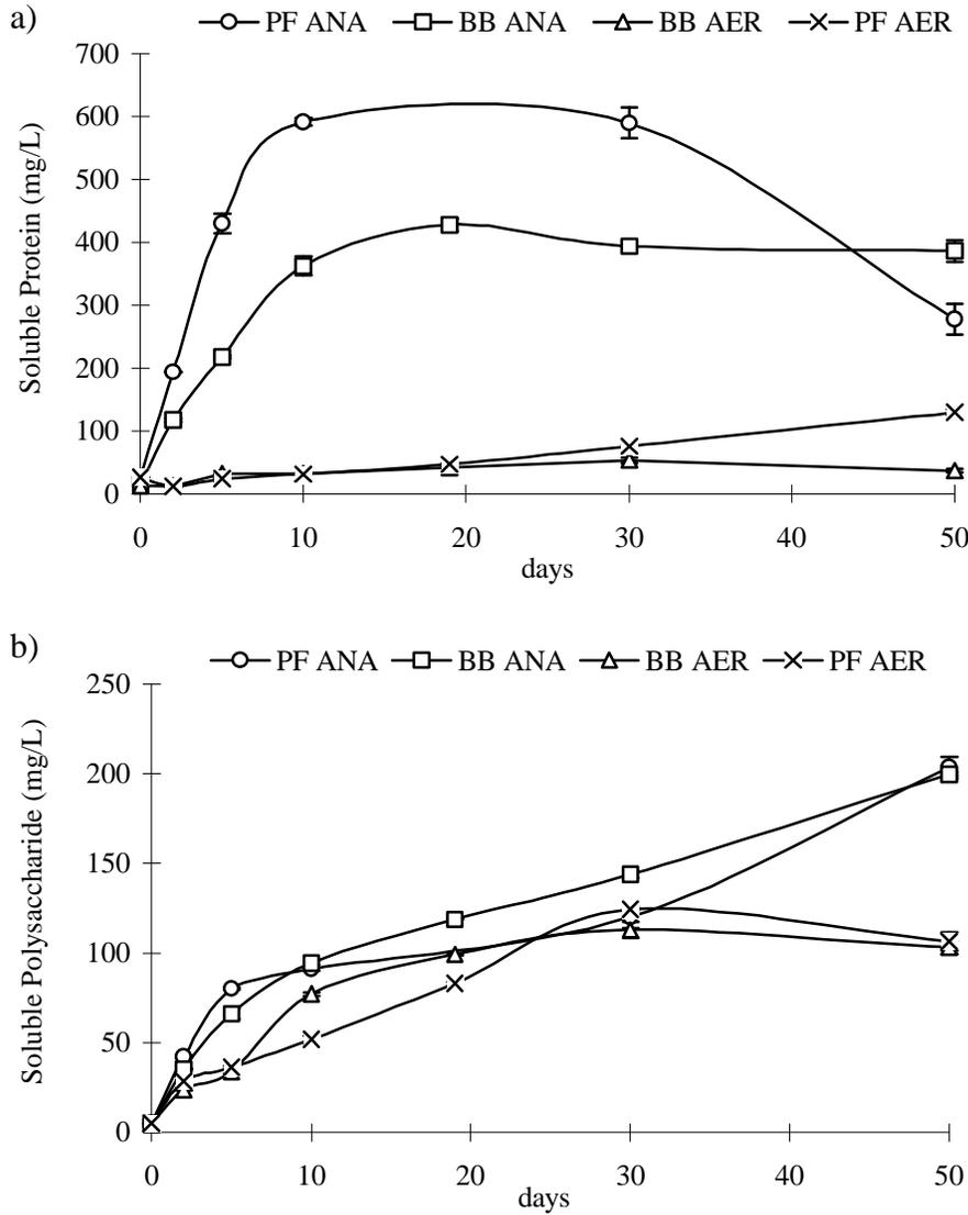
Figure 2: a) Soluble Protein, and b) Soluble Polysaccharide for Blacksburg (BB) and Pepper s Ferry (PF) Aerobic (AER) and Anaerobic (ANA) Digestion, 20°C
