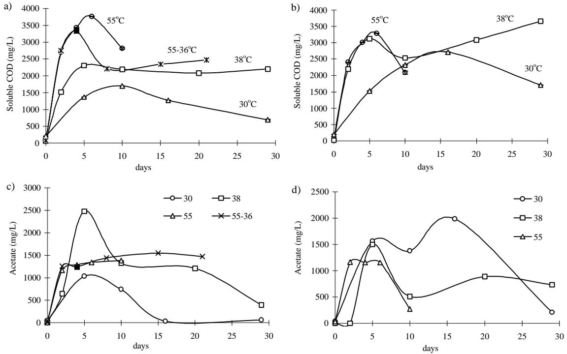
**Figure A5: a) Soluble COD, and c) Acetate for Pepper s Ferry Anaerobic Digestion Studies; and b) Soluble COD, and d) Acetate for Blacksburg Anaerobic Digestion Studies at Temperatures of 30, 38, 55, and 55-36°C. The black square in a) and c) represents the change from thermophilic to mesophilic conditions.**
