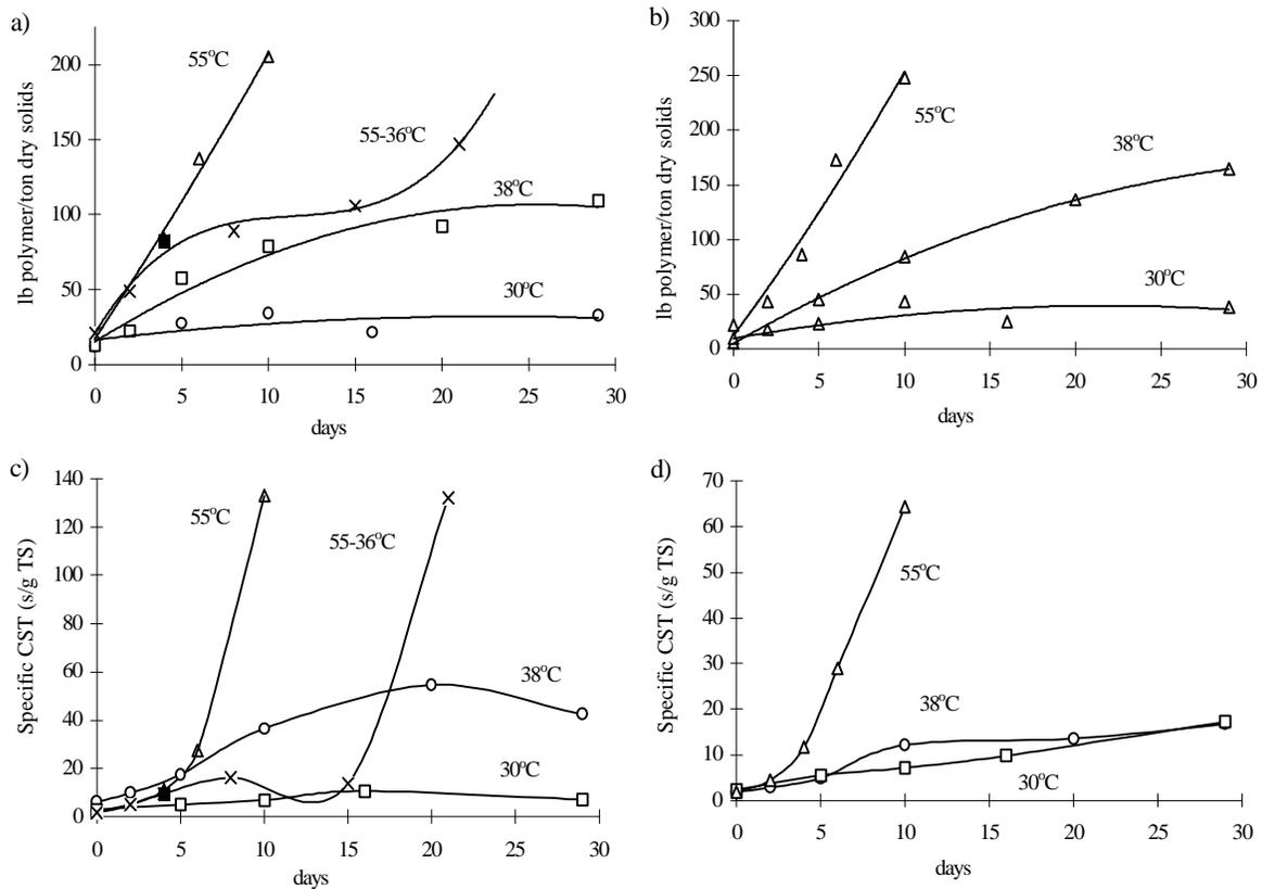
**Figure A2: a) Polymer Demand, and c) CST for Pepper s Ferry Anaerobic Digestion Studies; and b) Polymer Demand, and d) CST for Blacksburg Anaerobic Digestion Studies at Temperatures of 30, 38, 55, and 55-36°C. The black square in a) and c) represents the change from thermophilic to mesophilic conditions.**
