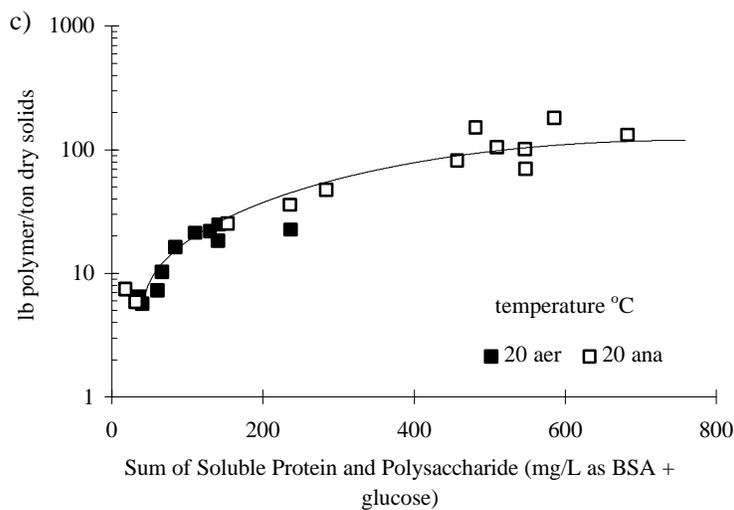
**Figure 3: Polymer Demand versus a) Soluble Protein, b) Soluble Polysaccharide, and c) Sum of Soluble Proteins and Polysaccharides for Blacksburg and Pepper s Ferry Aerobic (aer) and Anaerobic (ana) Digestion Studies, 20°C**
