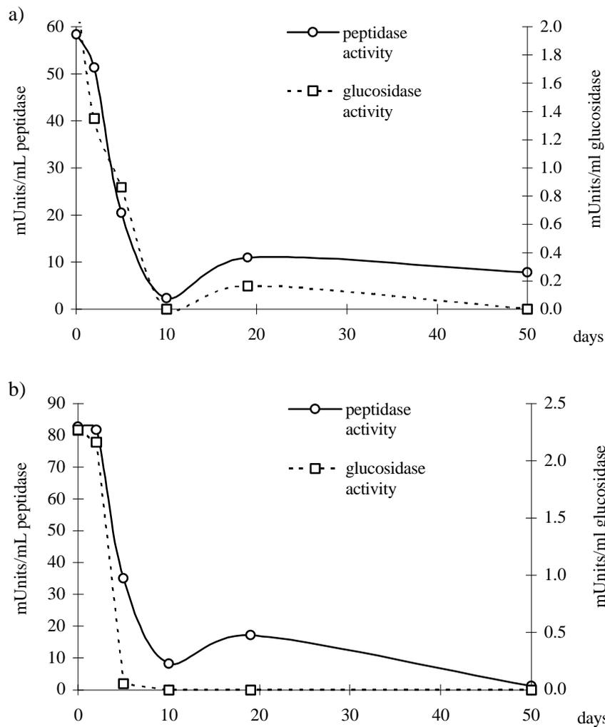
**Figure 9: Peptidase and Glucosidase Activities for a) Blacksburg, and b) Pepper s Ferry Aerobically Digested Biosolids, 20°C**
