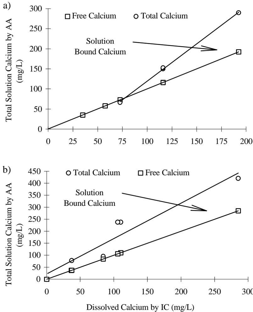
**Figure 6: Partitioning of Free and Colloidal Calcium Released to the Supernatant for a) Blacksburg, and b) Pepper's Ferry Aerobic Digestion Study, 20°C**
