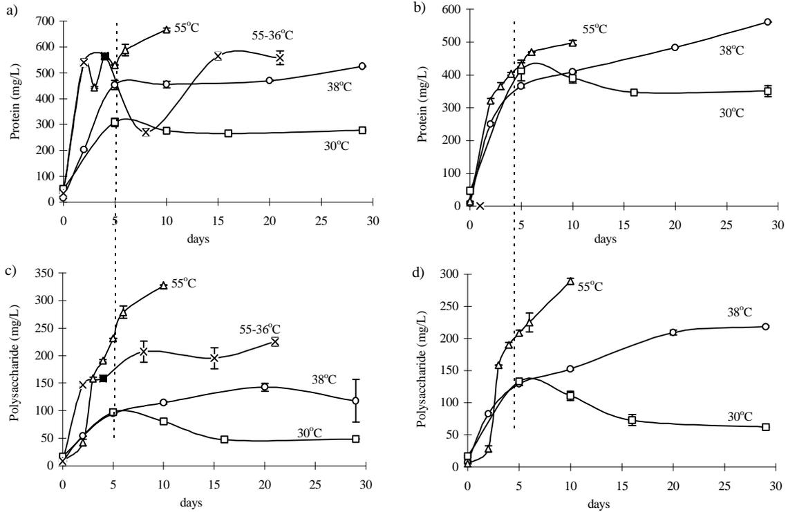
**Figure A3: a) Protein, and b) Polysaccharide for Pepper's Ferry Anaerobic Digestion Studies; and c) Protein, and d) Polysaccharide for Blacksburg Anaerobic Digestion Studies at Temperatures of 30, 38, 55, and 55-36°C. The black square in a) and b) represents the change from thermophilic to mesophilic conditions.**
