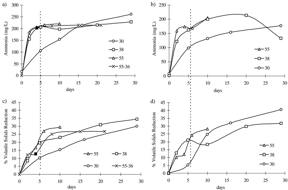
**Figure A4: a) Ammonia, and c) % Volatile Solids Reduction for Pepper's Ferry Anaerobic Digestion Studies; and b) Ammonia, and d) % Volatile Solids Reduction for Blacksburg Anaerobic Digestion Studies at Temperatures of 30, 38, 55, and 55-36°C. The black square in a) and c) represents the change from thermophilic to mesophilic conditions.**
