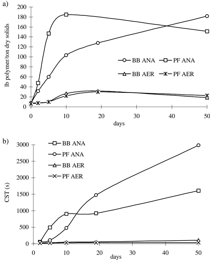
**Figure 1: a) Polymer Demand, and b) CST for Blacksburg (BB) and Pepper s Ferry (PF) Aerobic (AER) and Anaerobic (ANA) Digestion Study, 20°C**
