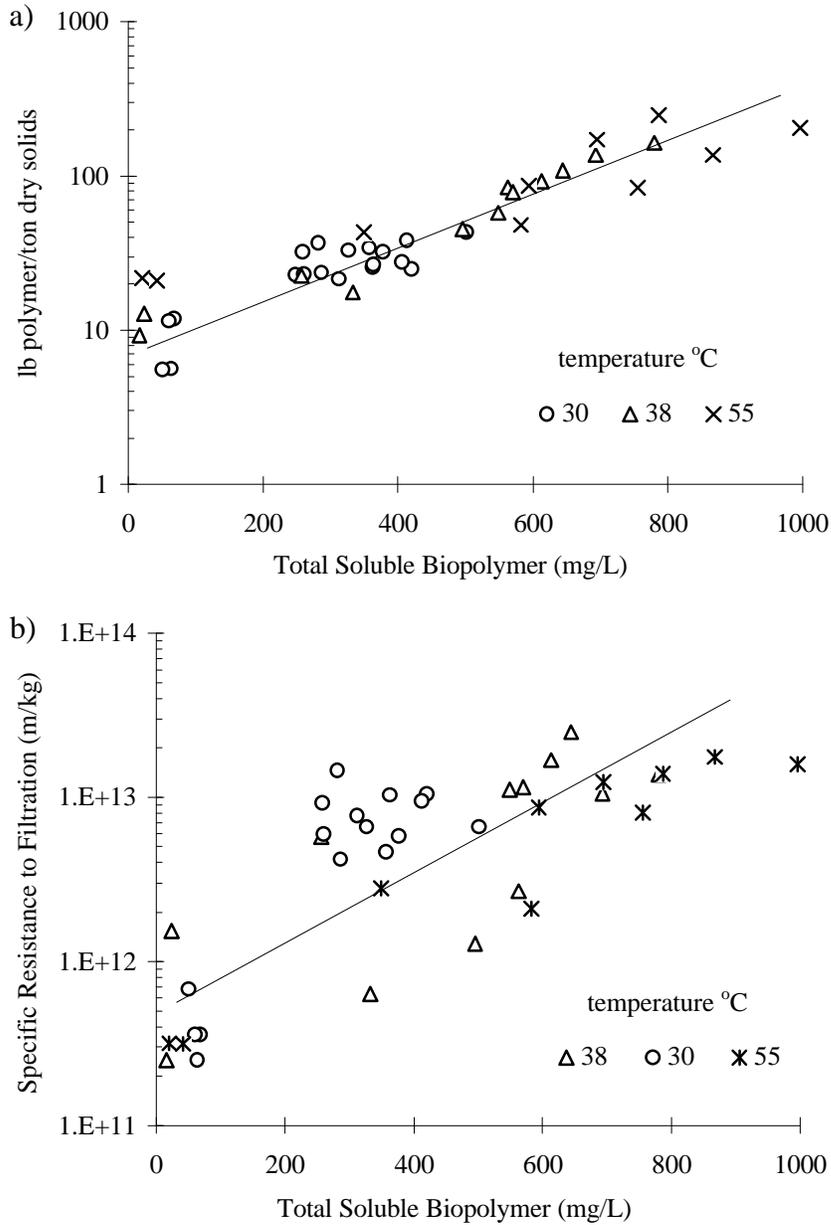
**Figure A1: a) Polymer Demand, and b) Specific Resistance to Filtration versus Total Soluble Biopolymer Concentration for Blacksburg and Pepper s Ferry Anaerobic Digestion Studies at 30, 38, and 55°C**
