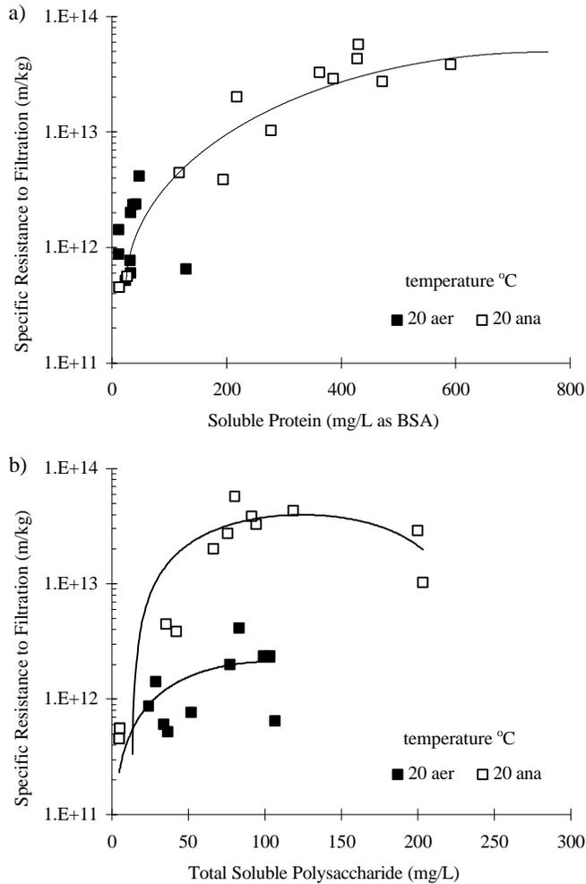
**Figure 4: Specific Resistance to Filtration versus a) Soluble Protein, and b) Soluble Polysaccharide for Blacksburg and Pepper's Ferry Aerobic (aer) and Anaerobic (ana) Digestion Studies, 20°C**
