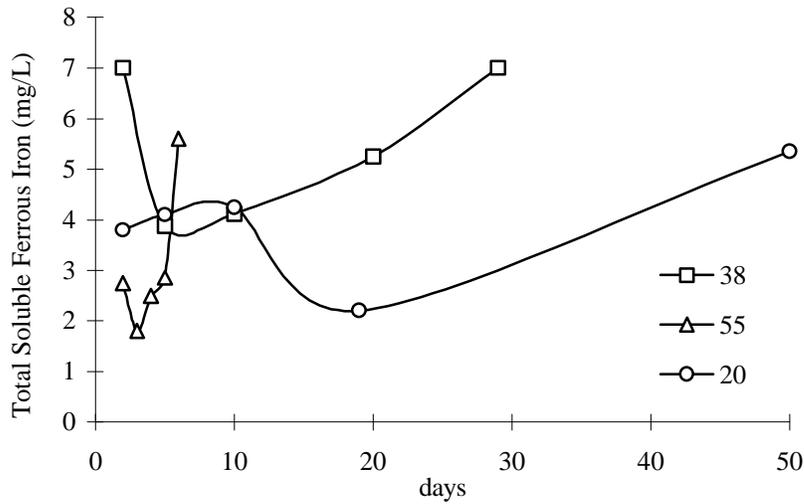
**Figure A6: Total Soluble Ferrous Iron Released for Pepper s Ferry Anaerobic Digestion Studies at Temperatures of 20, 38, and 55°C.**
