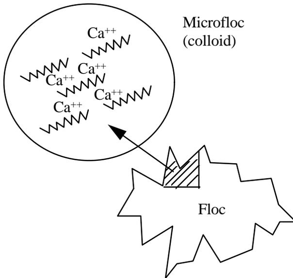
**Figure 8: An illustration of floc deterioration during digestion. Proteins and polysaccharides bound by calcium are released into solution as colloids (or microflocs) and not as discrete units.**
