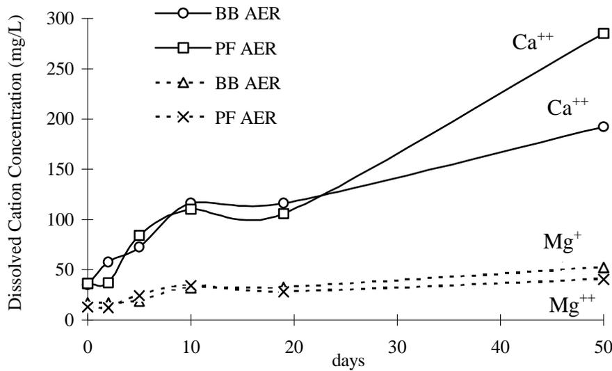
**Figure 5: Dissolved Calcium and Magnesium Concentrations for Blacksburg (BB) and Pepper s Ferry (PF) Aerobic (AER) Digestion Studies, 20°C**
