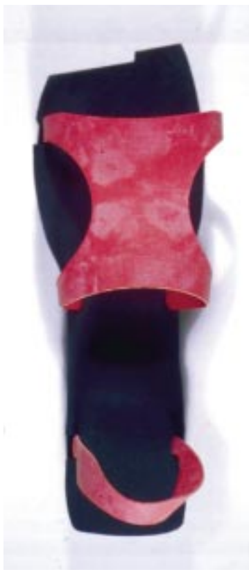
fig 3.7 – first iteration of lasercut foam prototype – all parts cut on LaserCMM
