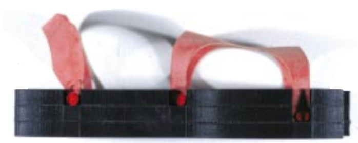
fig 3.7 – first iteration of lasercut foam prototype – all parts cut on LaserCMM
