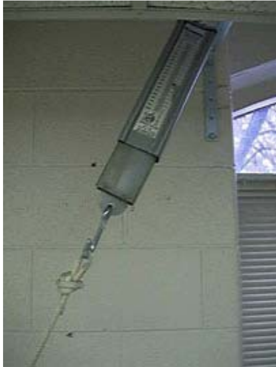
Lab 1, Exercise 1.2: detail of farm scale used to hang weights.
