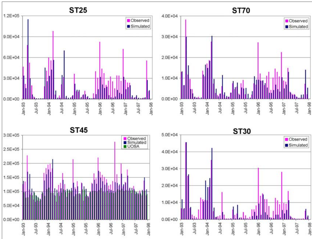
Figure 5-13: Comparisons of Monthly Oxidized Nitrogen Loads (lbs) at Four Principal Stream Stations in the Occoquan Watershed for Model Calibration (1993-1995) and Validation (1996-1997)
