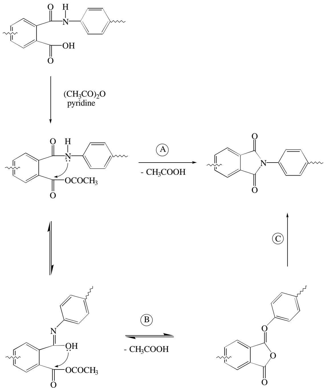
Figure 2.2.1.4.1: Proposed Mechanism for the Chemical Imidization Process<sup>78-80</sup>
