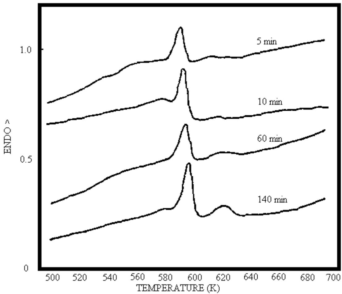
Figure 2.5.3: DSC Thermograms of LARC-TPI After Exposure to NMP at  $160\pm 10^\circ\text{C}$  as a Function of Time <sup>143</sup>
