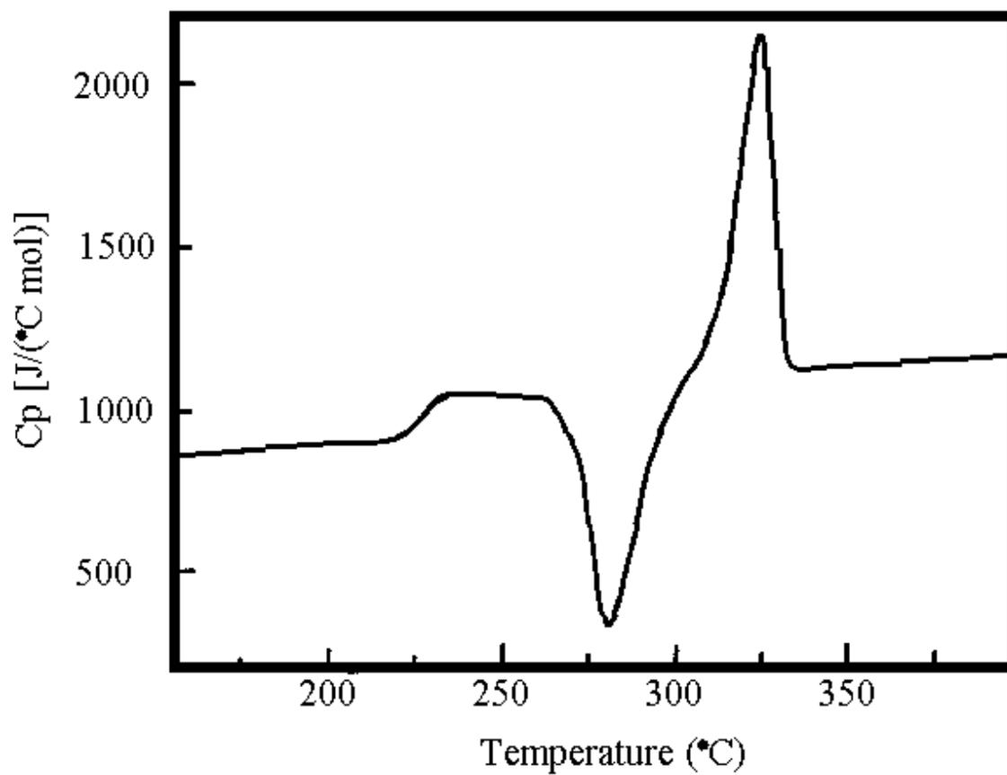
Figure 2.5.17: DSC Thermogram of BTDA-DMDA After Quenching from 400°C <sup>173</sup>
