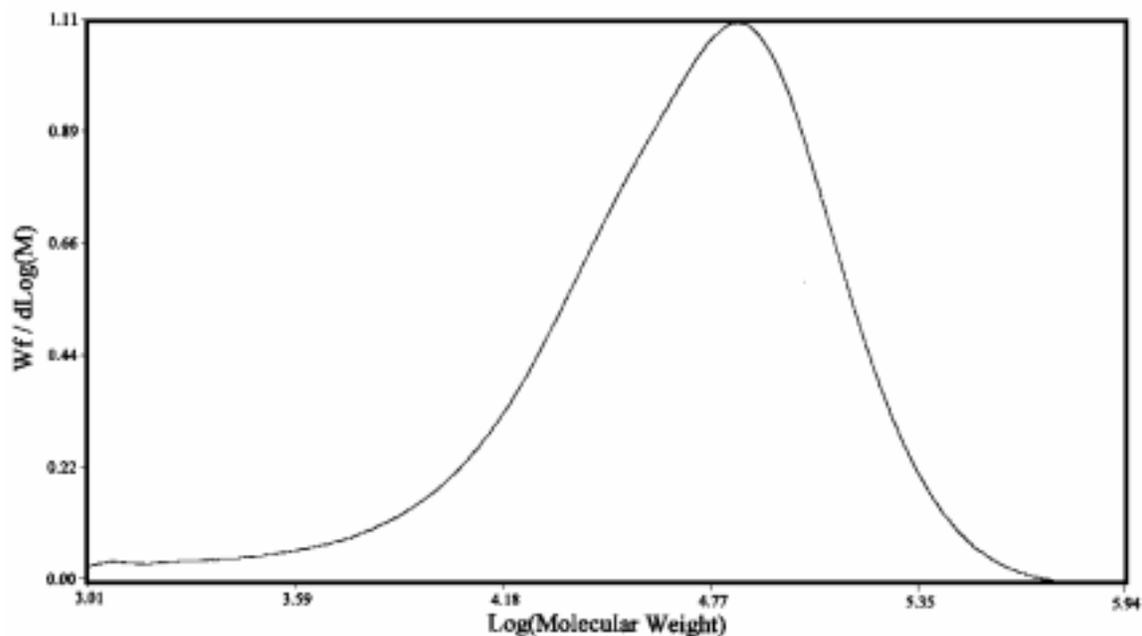
Figure 4.1.2: GPC Chromatogram of a TPER-BPDA-PA Polyamic Acid
