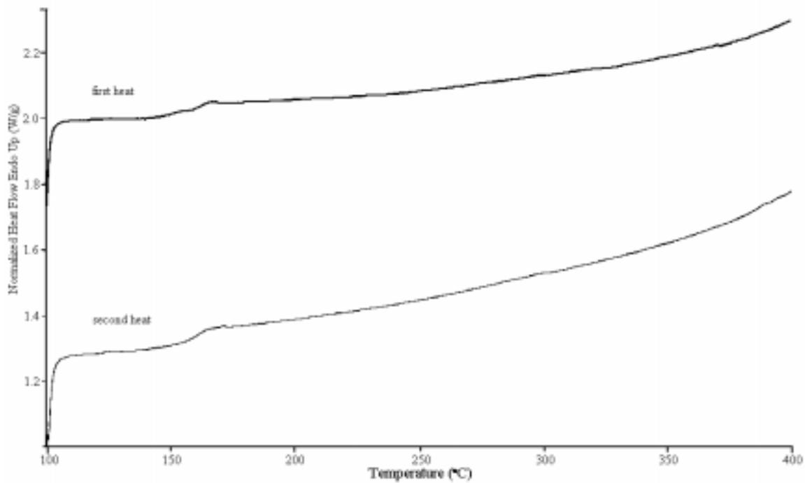
Figure 4.4.1.4.5: DSC Thermograms of BAPHB-ODPA-PA at 10°C/min
