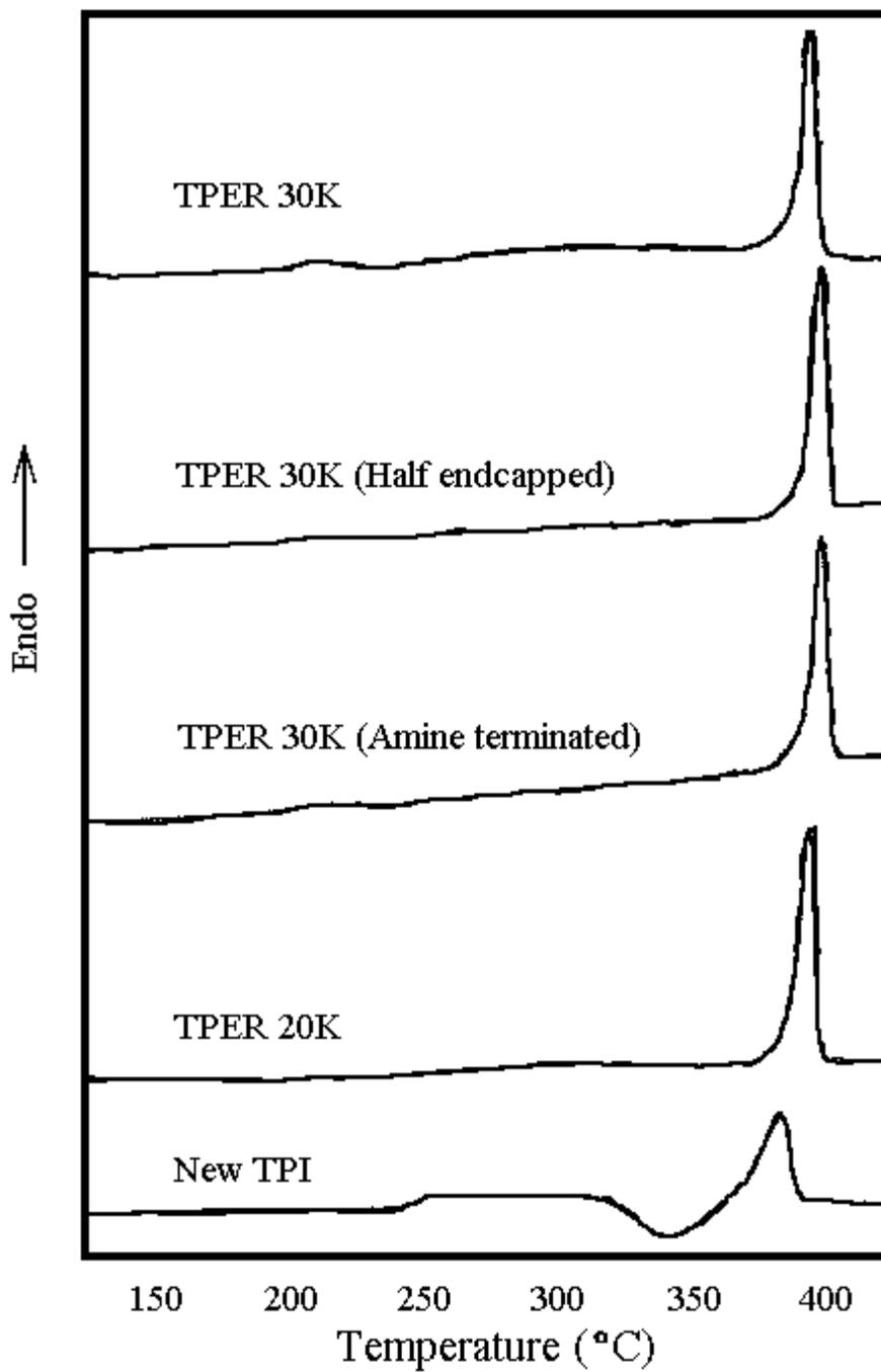
Figure 4.3.2.2.4: Second Heat DSC Thermograms of TPER-BPDA Samples at 10°C/min
