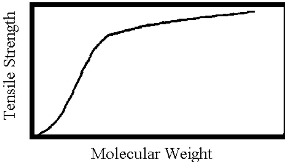
Figure 2.4.1: Effect of Polymer Number Average Molecular Weight ( $M_n$ ) on Tensile Strength ( $\sigma_b$ )<sup>131</sup>
