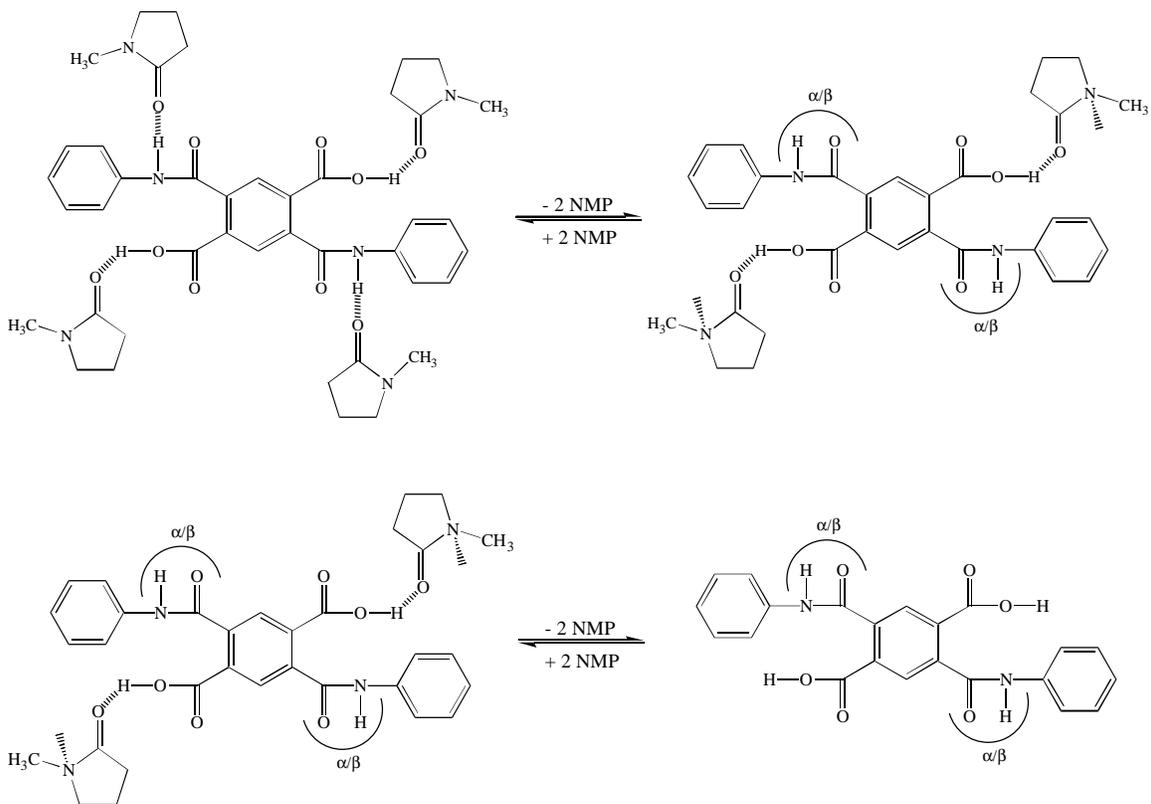
Scheme 2.2.1.1.3: Proposed NMP Solvent Complexation of Polyamic Acids<sup>22,23</sup>
