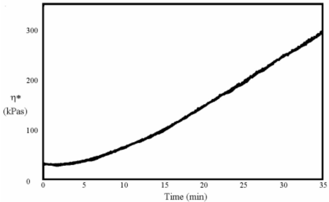
Figure 4.2.2.11: Complex Viscosity at 450°C Under Nitrogen as a Function of Time for 12.5K TPEQ-ODPA-PA
