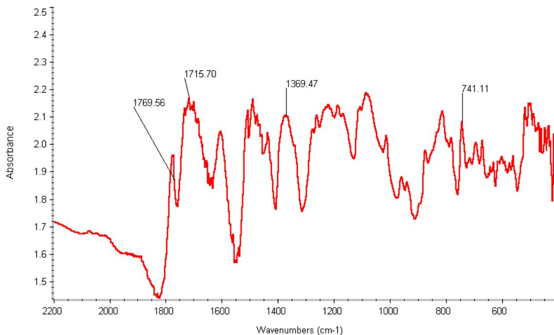
Figure 4.2.1.2: FTIR Spectrum of a Fully Imidized Polyimide Powder
