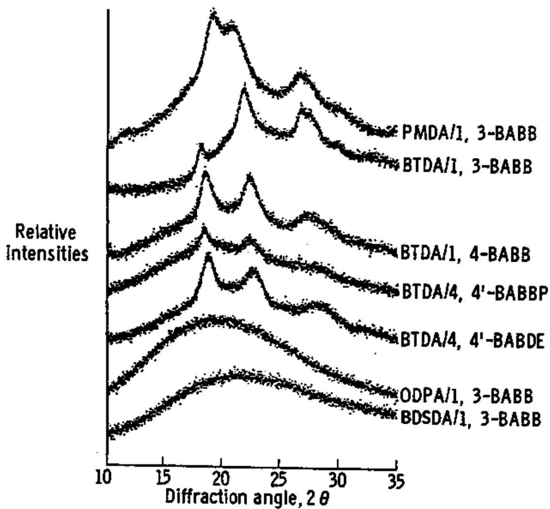
Figure 2.5.5: X-ray Diffractograms of Ether and Carbonyl-Containing Polyimide Films<sup>144</sup>
