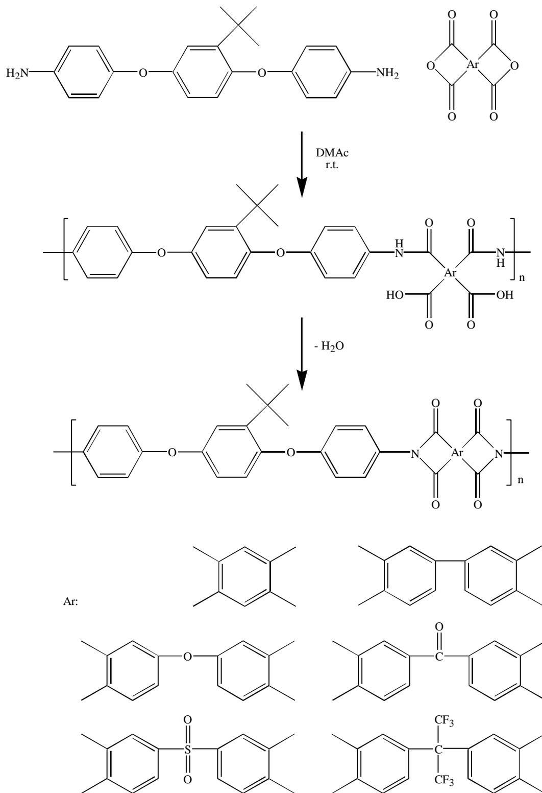
Scheme 2.6.5: Synthetic Scheme for BATB-Based Polyimides<sup>202</sup>
