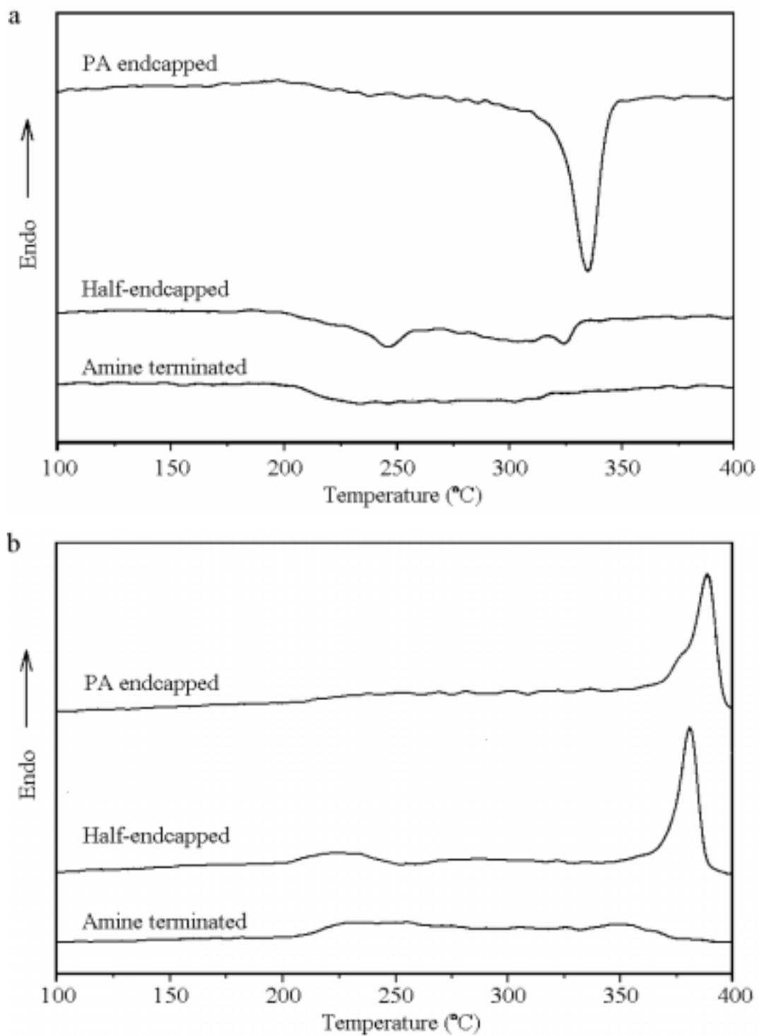
Figure 4.3.2.2.10: DSC Cooling (a) and Heating (b) Scans of TPER-BPDA Samples of Different Degree of Endcapping (10°C/min)
