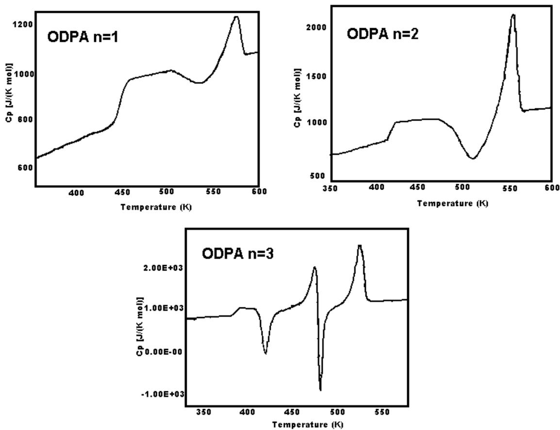
Figure 2.5.15: DSC Thermograms of 1-(m-aminophenoxy)-2-(p-aminophenoxy)ethane-ODPA Polyimides of Varying Oxyethylene Lengths <sup>170</sup>
