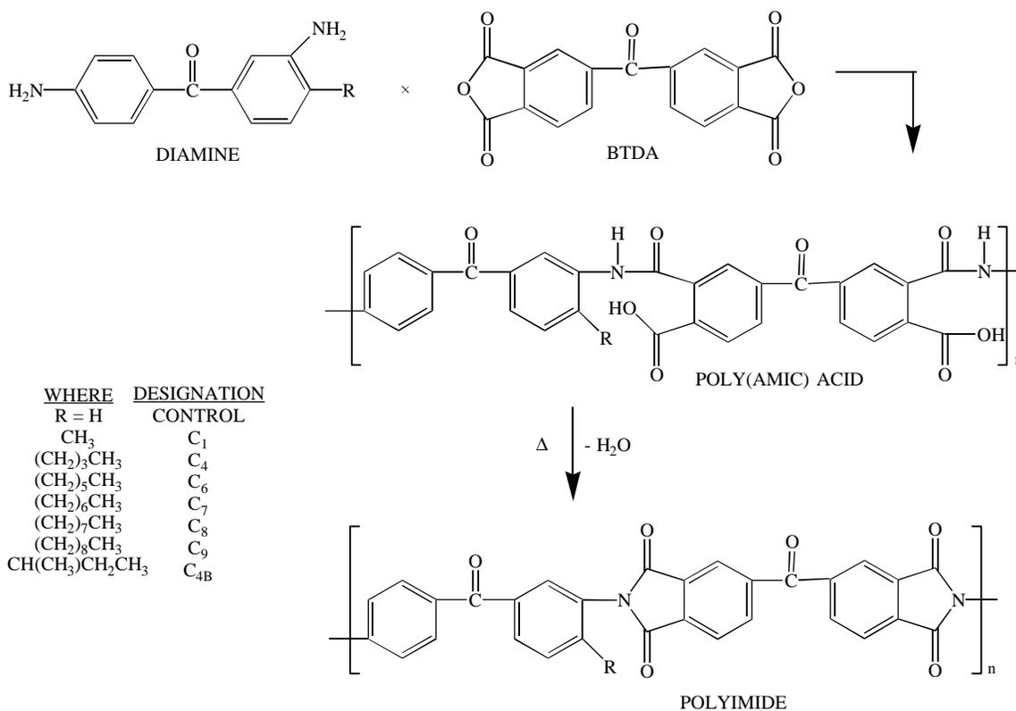
Scheme 2.6.1: Polyimide Synthetic Scheme for Alkylated Benzophenone Diamines with BTDA<sup>186</sup>
