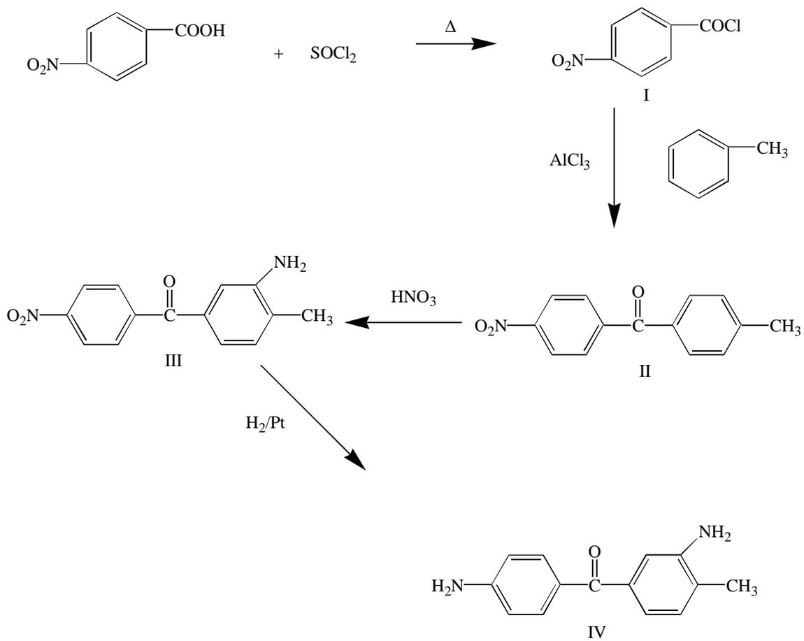
Scheme 2.6.2: Representative Synthetic Scheme for Alkylated Benzophenone Diamines<sup>186</sup>
