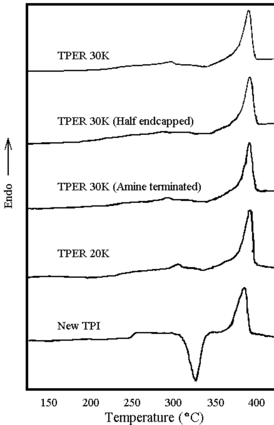
Figure 4.3.2.2.3: First Heat DSC Thermograms of TPER-BPDA Samples at 10°C/min
