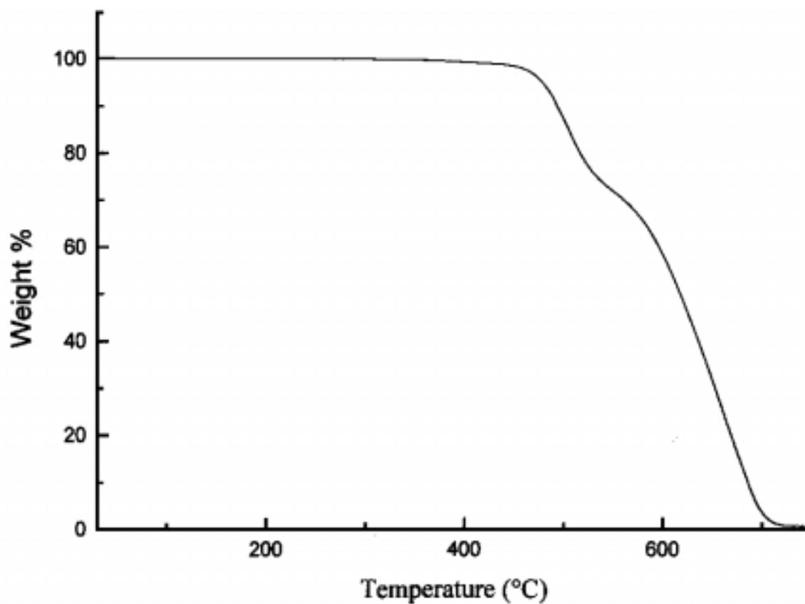
Figure 4.4.1.4.3: TGA Thermogram of BAPHB-ODPA-PA at 10°C/min
