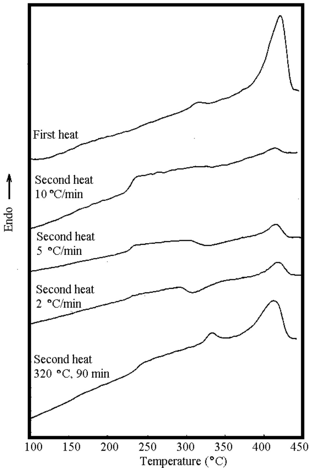
Figure 4.2.2.6: DSC Thermograms of 15K TPEQ-ODPA-PA at 10°C/min
