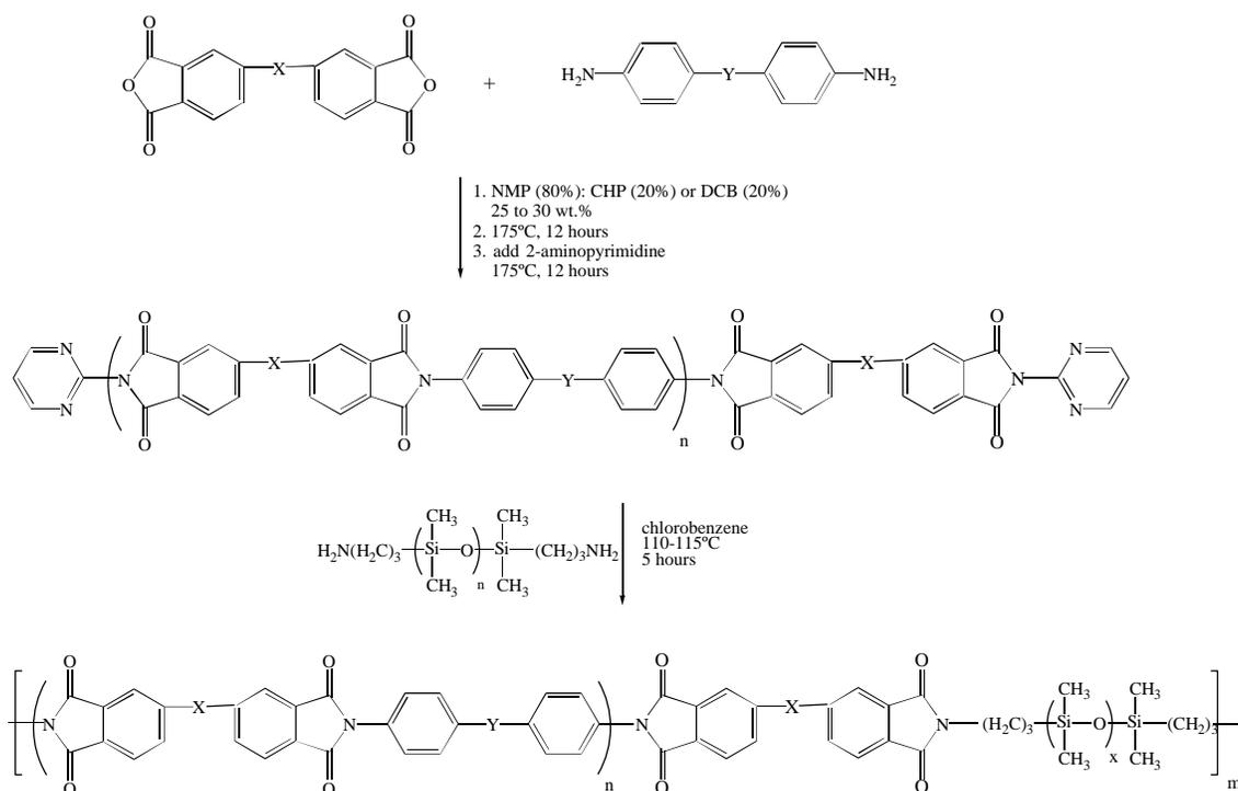
Scheme 2.2.2.4.3: Synthesis of Polyimide Siloxane Copolymers by Transimidization<sup>123</sup>
