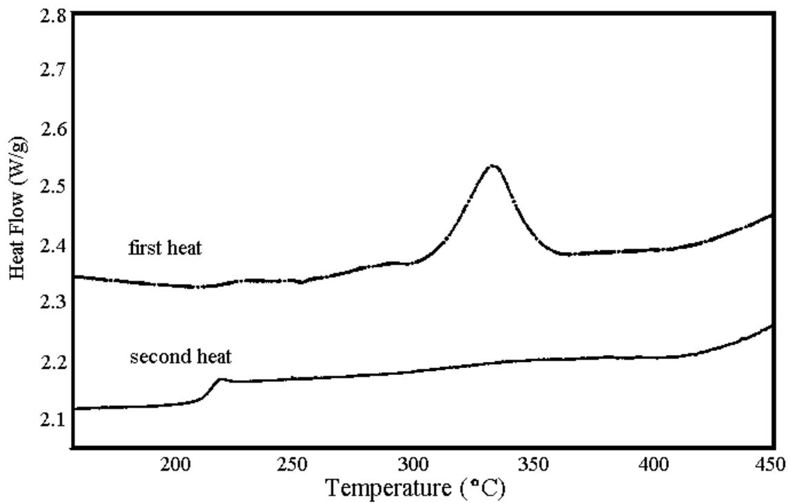
Figures 4.3.1.2: DSC Thermograms of TPER-ODPA-PA at 10°C/min
