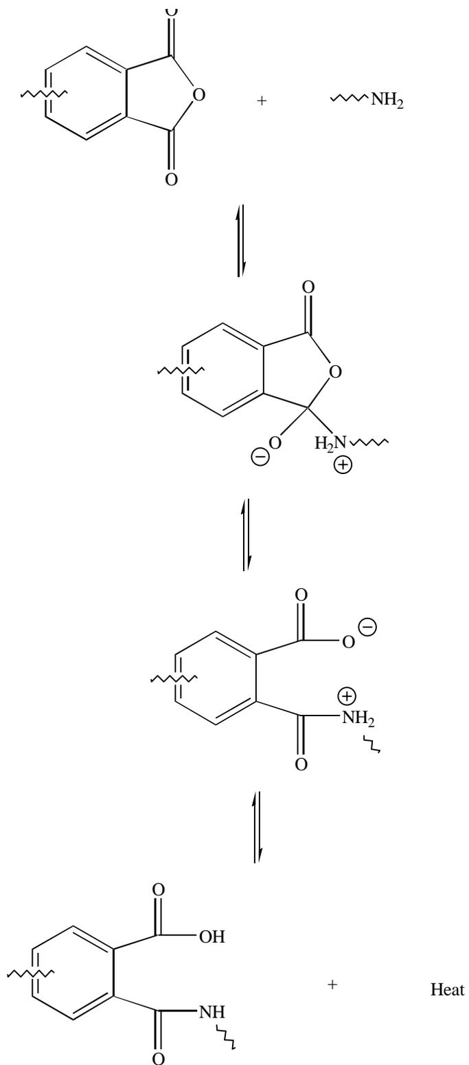
Scheme 2.2.1.1.2: Proposed Mechanism for Polyamic Acid Formation<sup>19-21</sup>
