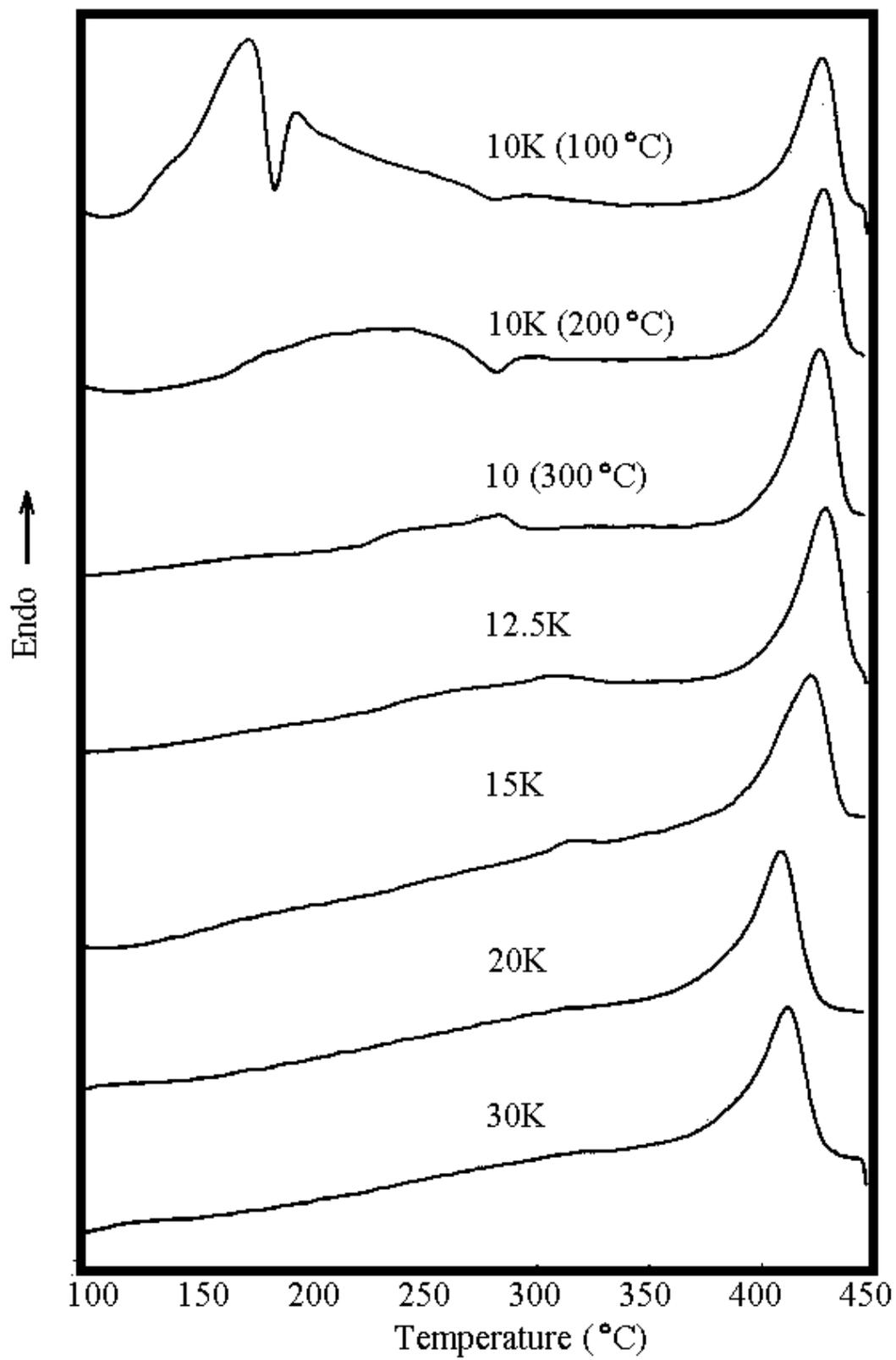
Figure 4.2.2.4: First Heat DSC Thermograms of TPEQ-ODPA-PA Samples at 10°C/min
