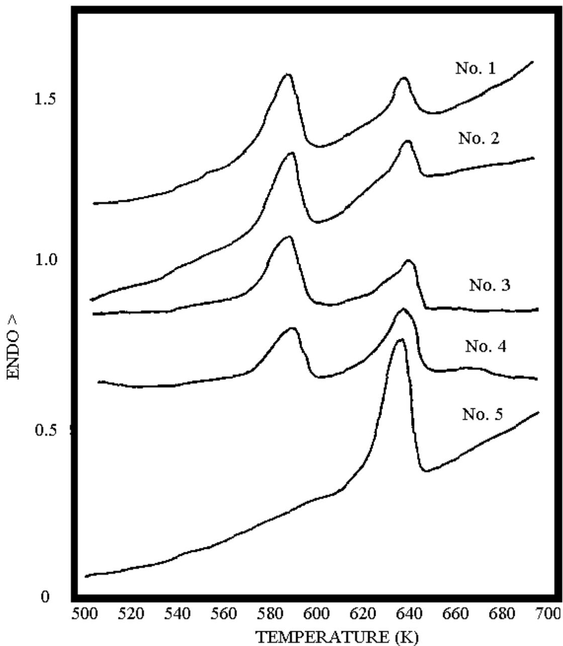
Figure 2.5.2: DSC Thermograms of LARC-TPI After Exposure to NMP at 200°C <sup>143</sup>
