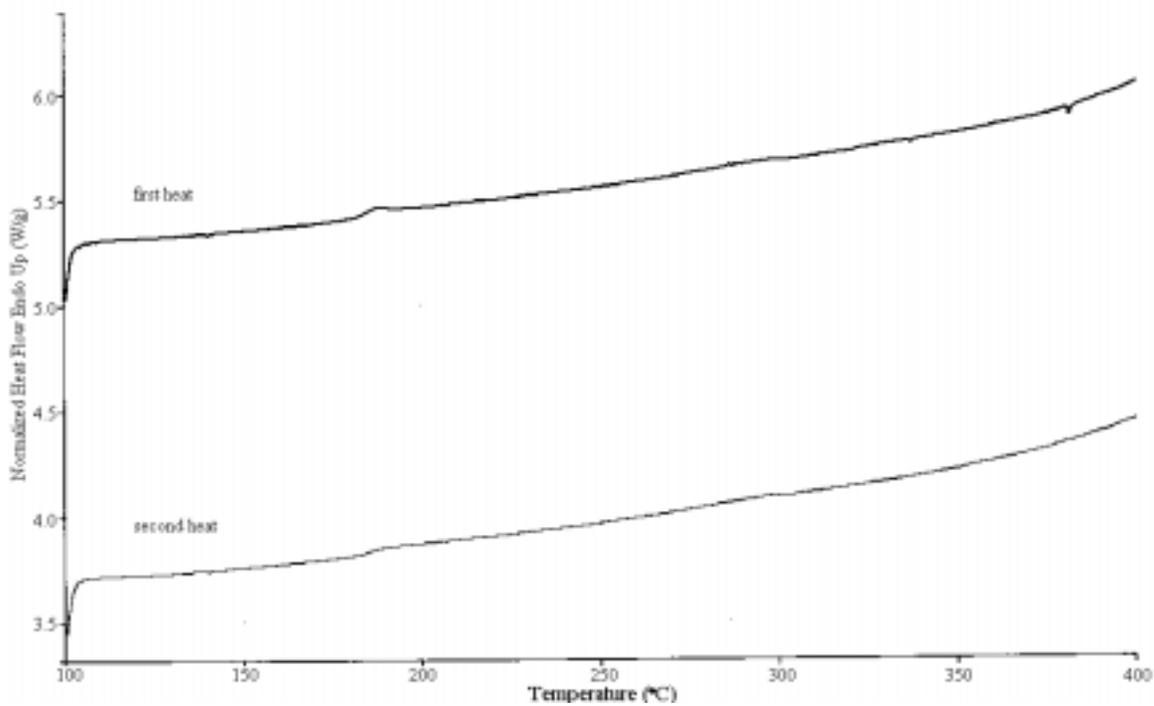
Figure 4.4.1.4.4: DSC Thermograms of BAPHB-BPDA-PA at 10°C/min
