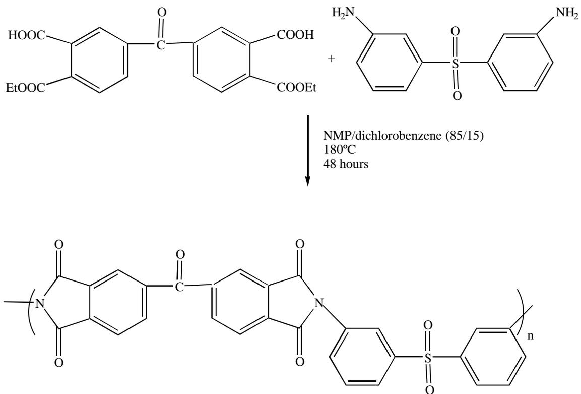
Scheme 2.2.2.2: Synthesis of BTDA-3,3'-DDS Using the Diester-Diacid of BTDA<sup>97</sup>
