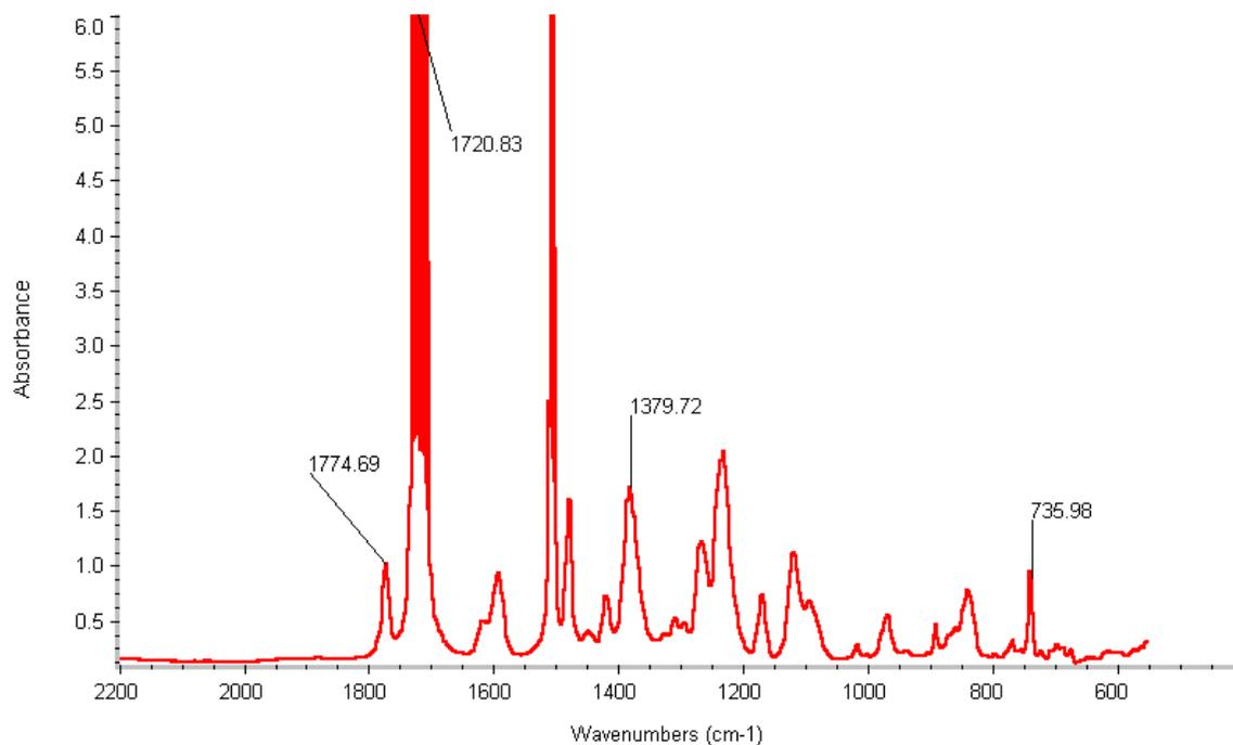
Figure 4.3.2.2.2: FTIR Spectrum of TPER-BPDA-PA
