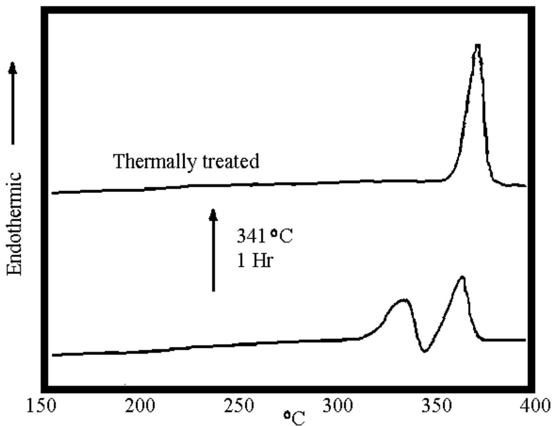
Figure 2.5.8: DSC Thermograms of As-received (Bottom) and Annealed (Top) Samples of LARC-CPI-2<sup>149</sup>
