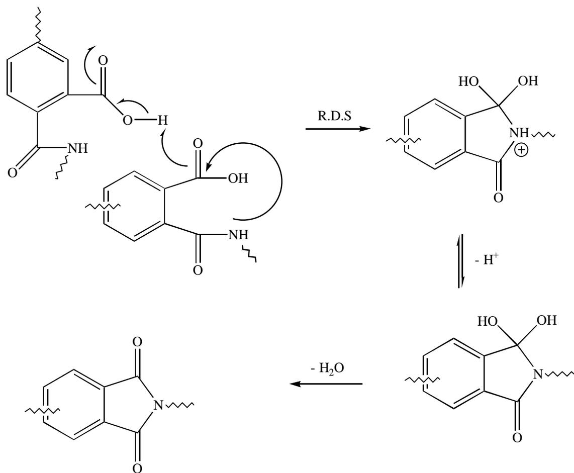
Figure 2.2.1.3.2: Proposed Mechanism for the Solution Imidization Process <sup>62</sup>
