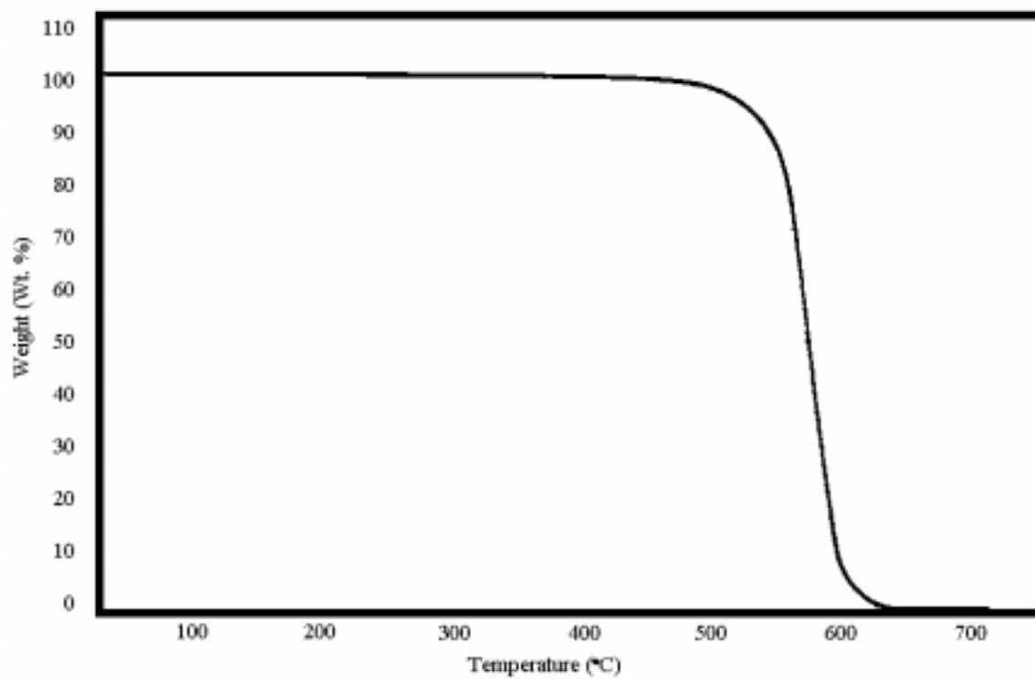
Figure 4.2.1.3: TGA Thermogram of TPEQ-BPDA-PA Polyimide Powder in Air at 10°C/min
