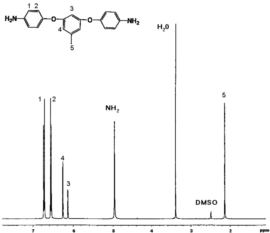
Figure 4.4.1.3.2: Proton NMR Spectrum of 3,5-bis(4-aminophenoxy)toluene (3,5-BAPT) in DMSO-d<sub>6</sub>
