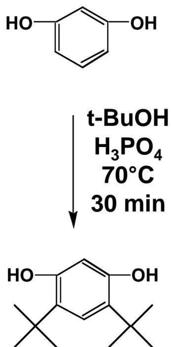
Scheme 4.4.1.1: Synthesis of Di-t-butylresorcinol by Electrophilic Aromatic Substitution
