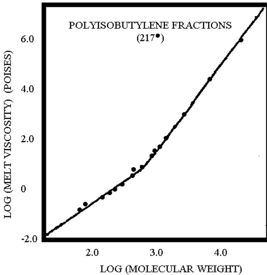
Figure 2.4.2: Effect of Polymer Weight Average Molecular Weight ( $M_w$ ) on Melt Viscosity<sup>132</sup>
