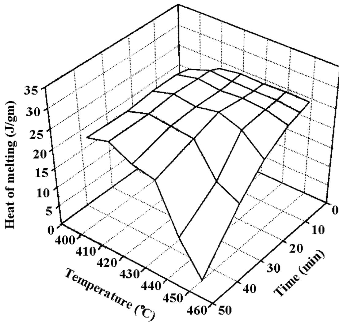
Figure 4.3.2.2.9: Effect of Temperature and Time in the Melt on the Heat of Crystallization of 30K TPER-BPDA-PA<sup>224,236</sup>
