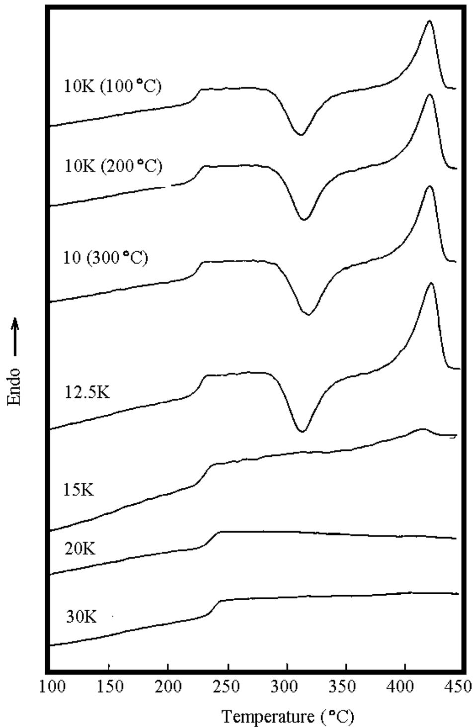
Figure 4.2.2.5: Second Heat DSC Thermograms of TPEQ-ODPA-PA Samples at 10°C/min
