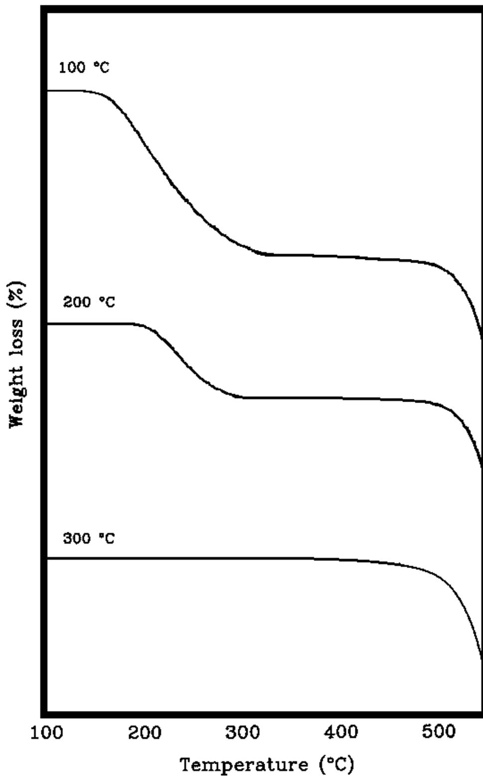
Figure 4.2.2.2: Influence of Imidization Temperature on TGA Weight Loss Behavior of 10K TPEQ-ODPA-PA Samples (10°C/min)
