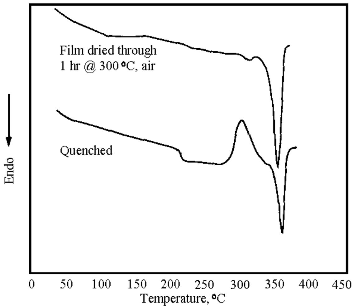
Figure 2.5.6: DSC Thermograms of LARC-CPI <sup>148</sup>
