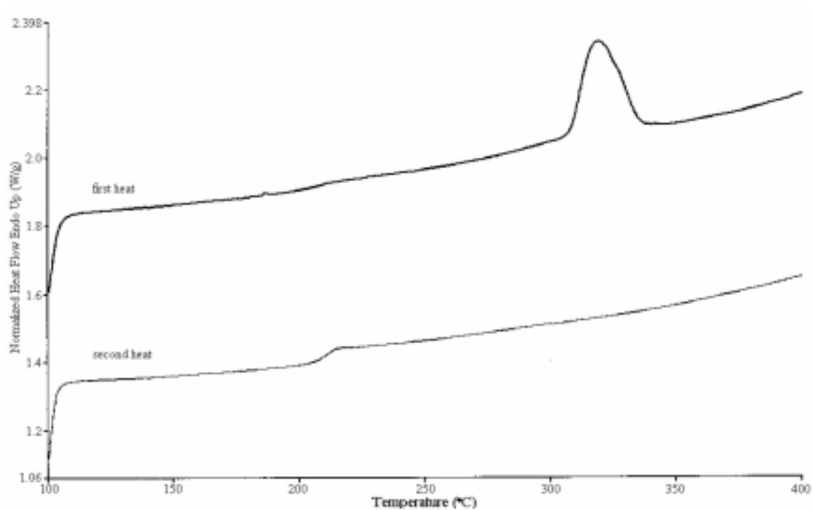
Figure 4.4.1.4.2: DSC Thermograms of 3,5-BAPT-ODPA-PA at 10°C/min
