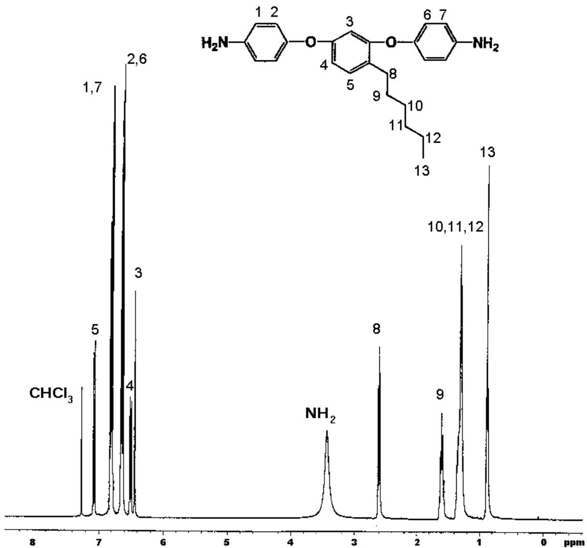
Figure 4.4.1.3.3: Proton NMR Spectrum of 1,3-bis(4-aminophenoxy)-4-hexylbenzene (BAPHB) in CDCl<sub>3</sub>
