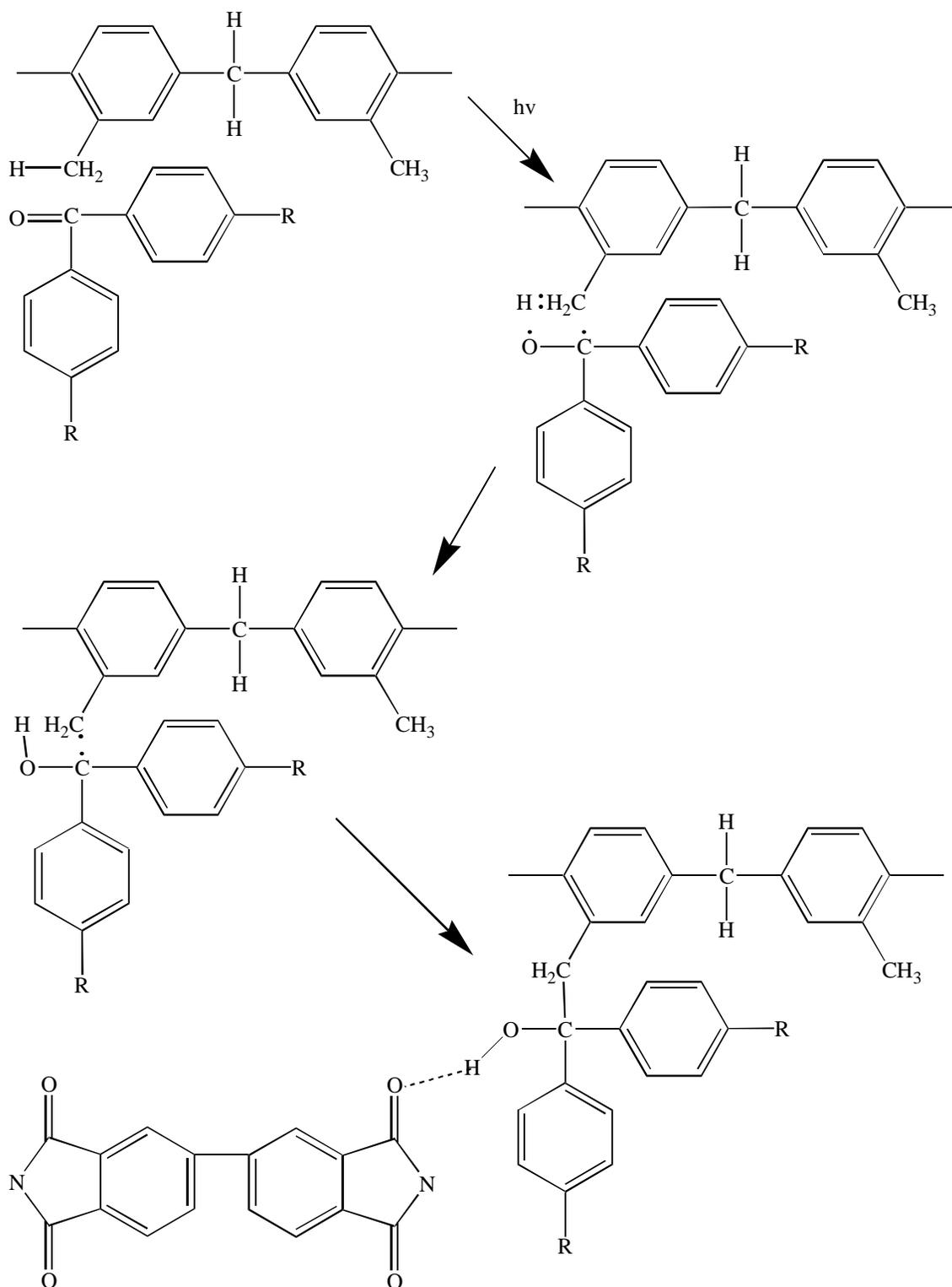
Scheme 2.6.7: Photocoupling and Hydrogen Bonding of Alkylated Polyimide with Benzophenone<sup>210</sup>
