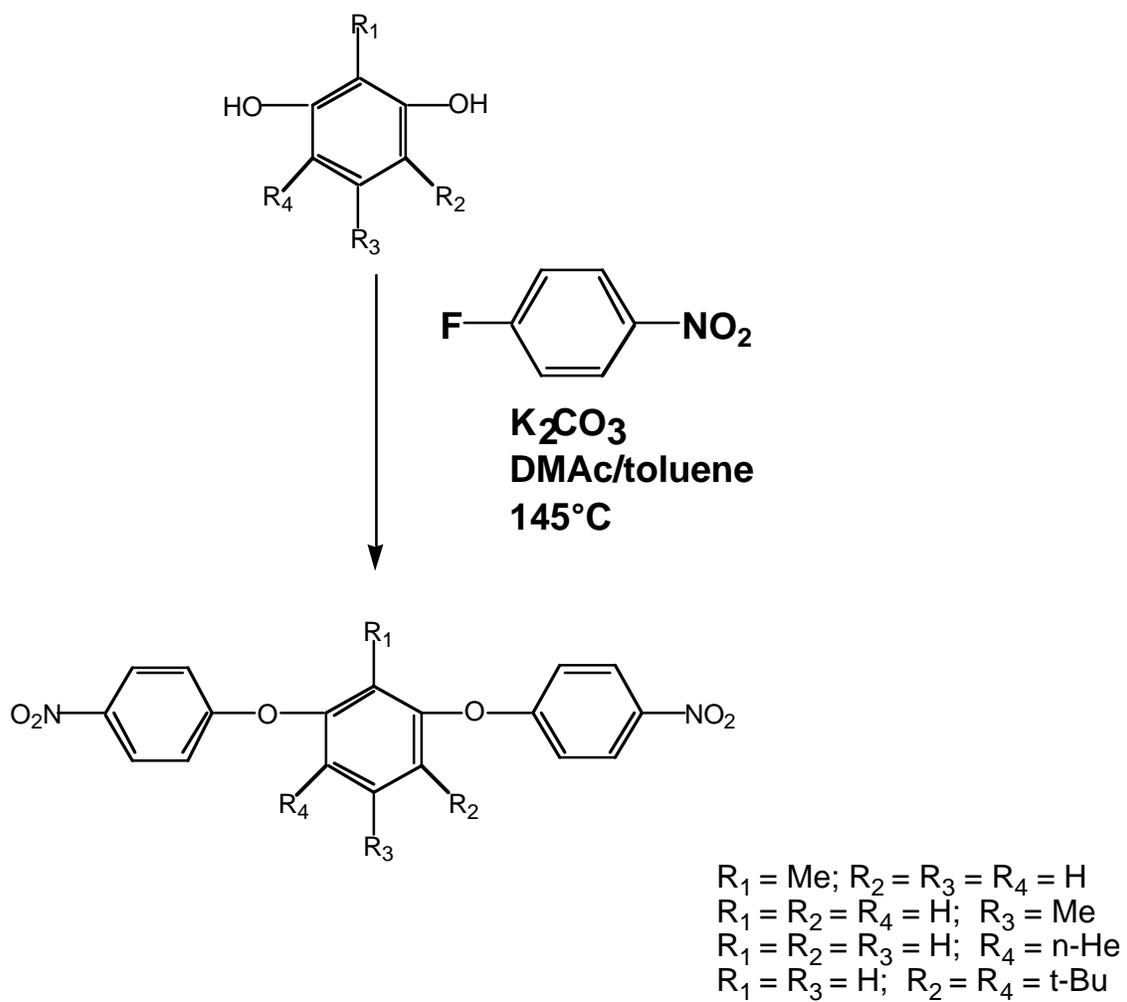
Scheme 4.4.1.2: Synthesis of 1,4-bis(4-nitrophenoxy)alkylbenzenes by Nucleophilic Aromatic Substitution
