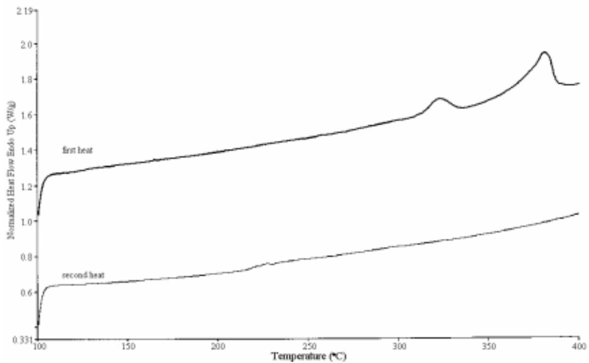
Figure 4.4.1.4.1: DSC Thermograms of 2,6-BAPT-ODPA-PA at 10°C/min
