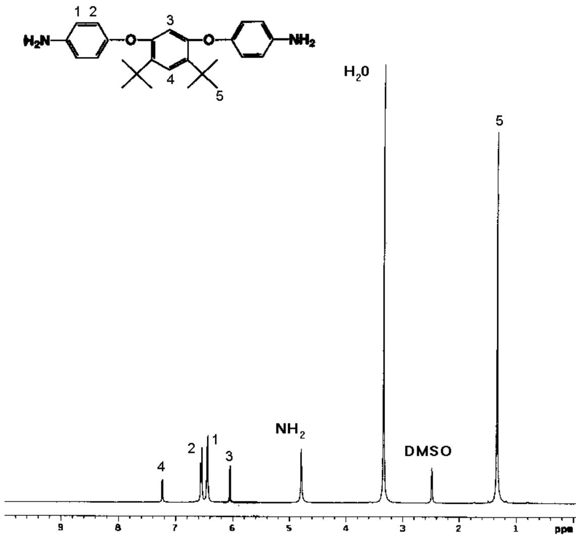
Figure 4.4.1.3.4: Proton NMR Spectrum of 1,3-bis(4-aminophenoxy)-4,6-di-tert-butylbenzene (BAPDTB) in DMSO-d<sub>6</sub>
