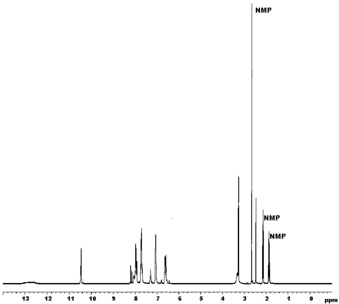
Figure 4.1.1: Proton NMR Spectrum of a Precipitated Polyamic Acid (in DMSO-d6)
