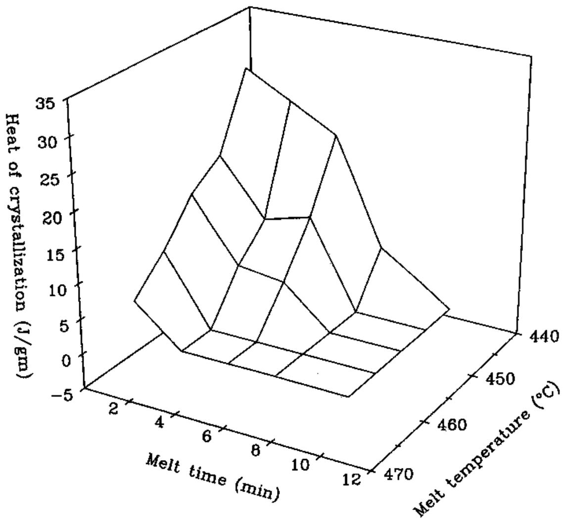
Figure 4.2.2.10: Effect of Temperature and Time in the Melt under Nitrogen on the Heat of Crystallization of 12.5K TPEQ-ODPA-PA<sup>224,235</sup>
