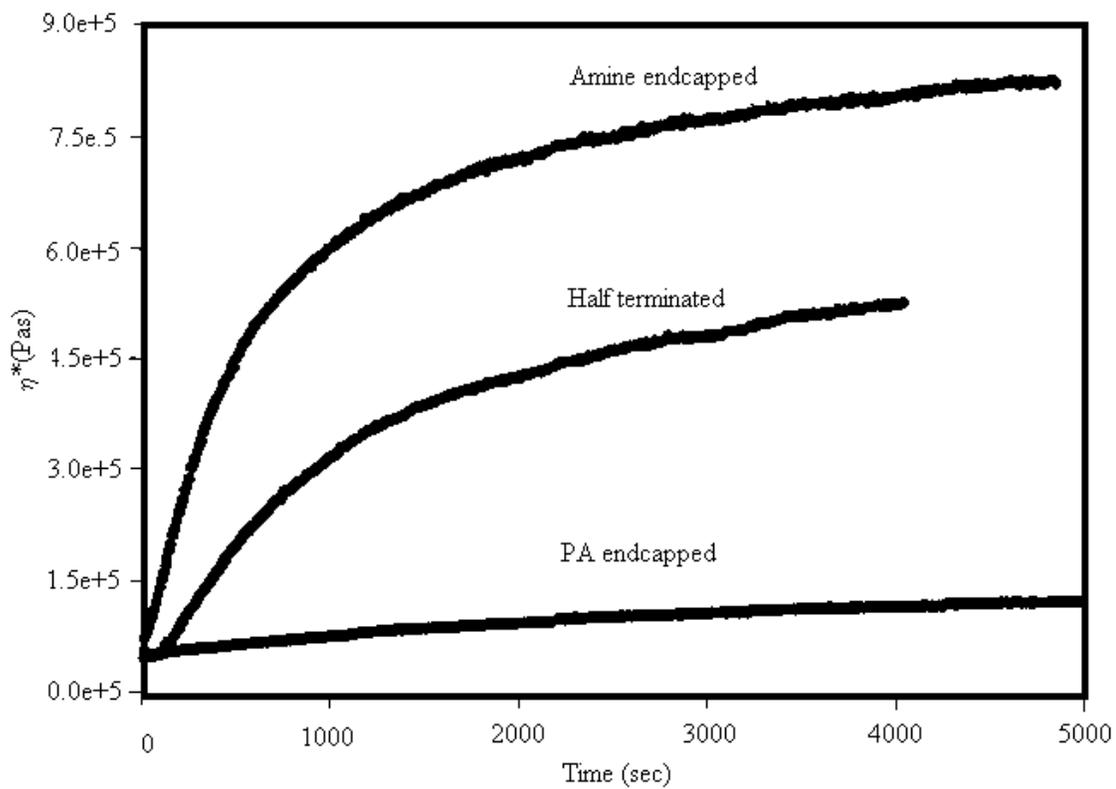
Figure 4.3.2.2.11: Isothermal Melt Rheology at 430°C of the TPER-BPDA Samples of Different Degree of Endcapping
