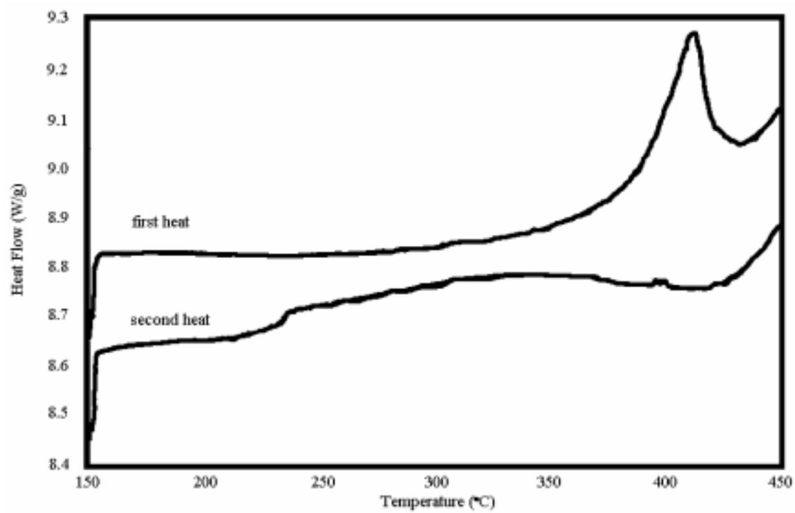
Figure 4.2.2.1: DSC Thermograms of 30 kg/mole TPEQ-ODPA-PA at 10°C/min
