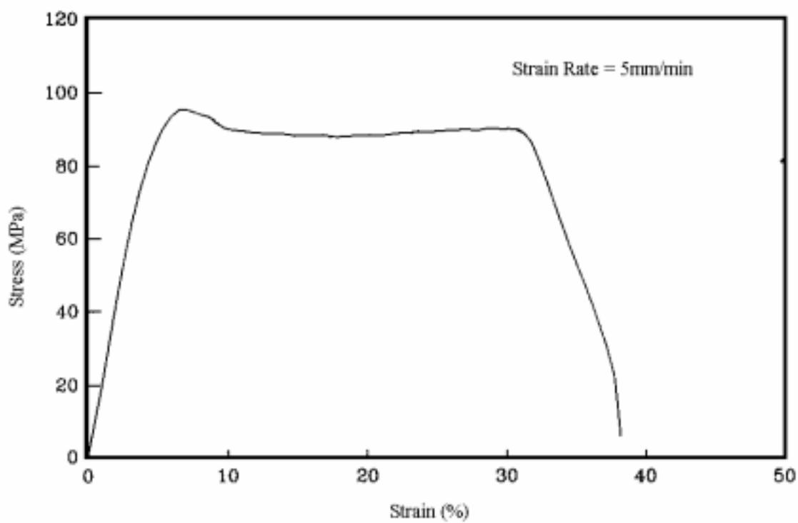
Figure 4.3.2.2.8: Room Temperature Stress-Strain Behavior of TPER-BPDA-PA
