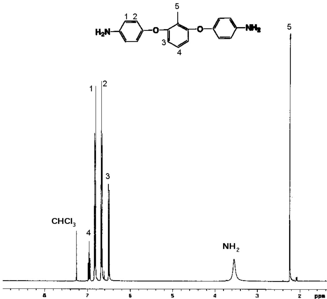
Figure 4.4.1.3.1: Proton NMR Spectrum of 2,6-bis(4-aminophenoxy)toluene (2,6-BAPT) in CDCl<sub>3</sub>
