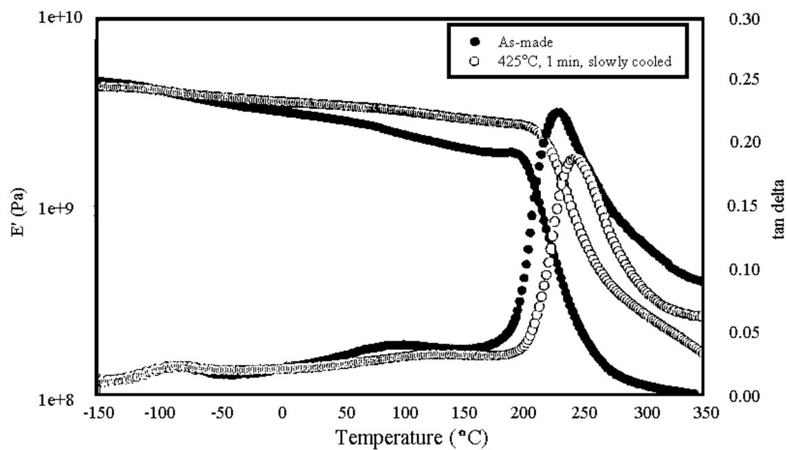
Figure 4.3.2.2.6: DMA Spectra of As-made and Slow Cooled (1°C/min) Samples of TPER-BPDA-PA
