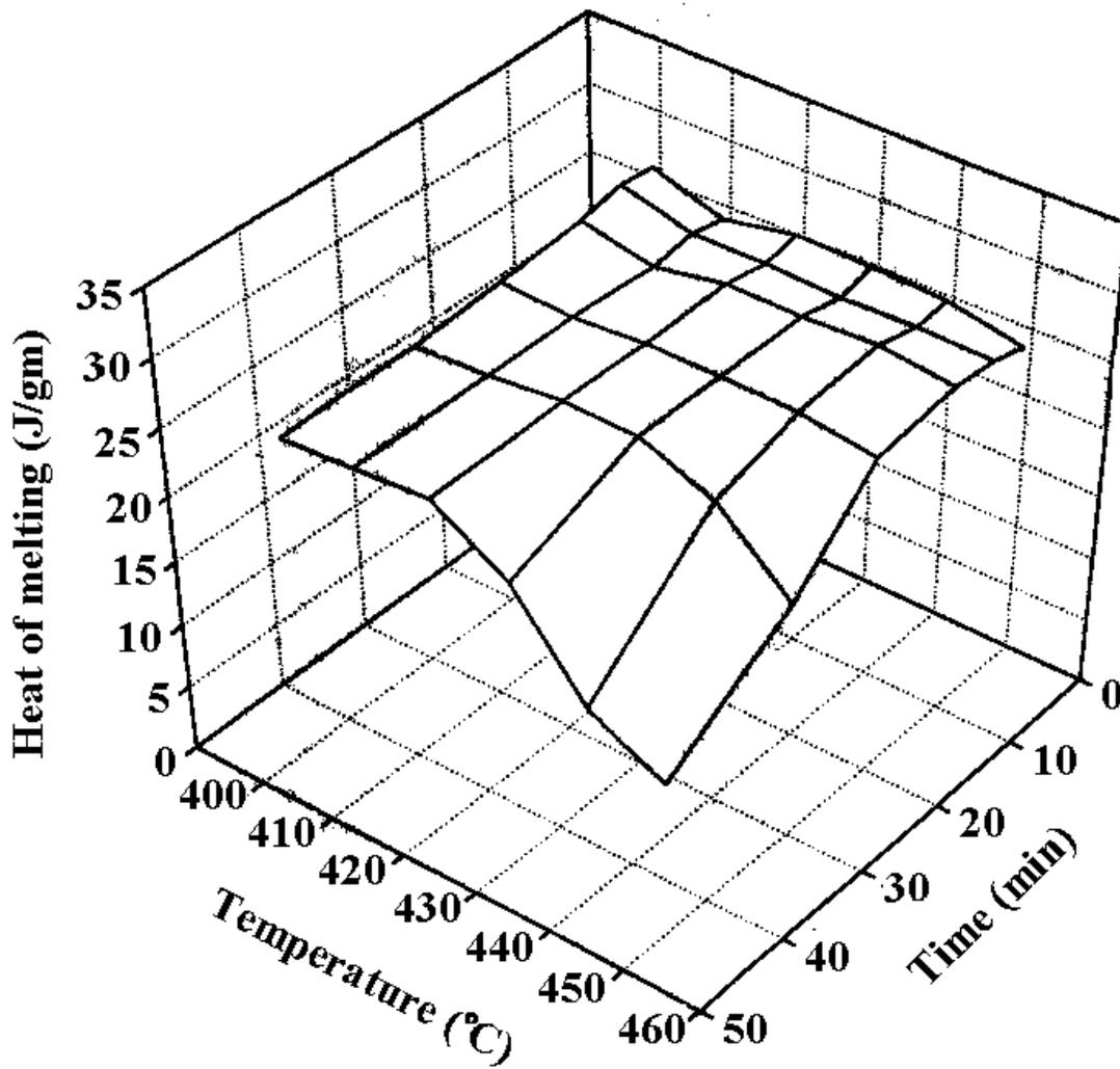
Figure 4.3.2.2.7: Effect of Temperature and Time in the Melt on the Heat of Melting of 30K TPER-BPDA-PA<sup>224,236</sup>
