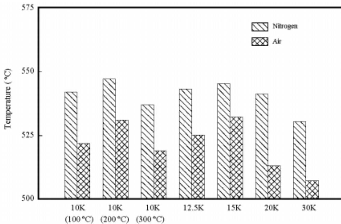
Figure 4.2.2.3: 5% Weight Loss Temperature of Fully Cyclized TPEQ-ODPA-PA Samples
