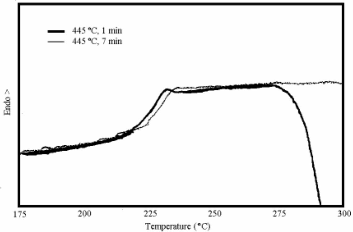
Figure 4.2.2.12: DSC Scans for Melt-Treated 12.5K TPEQ-ODPA-PA at 10°C/min
