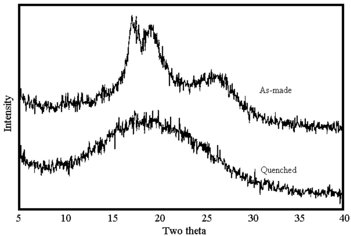
Figure 4.2.2.8: Wide Angle X-ray Scattering (WAXS) Patterns for 15K TPEQ-ODPA-PA
