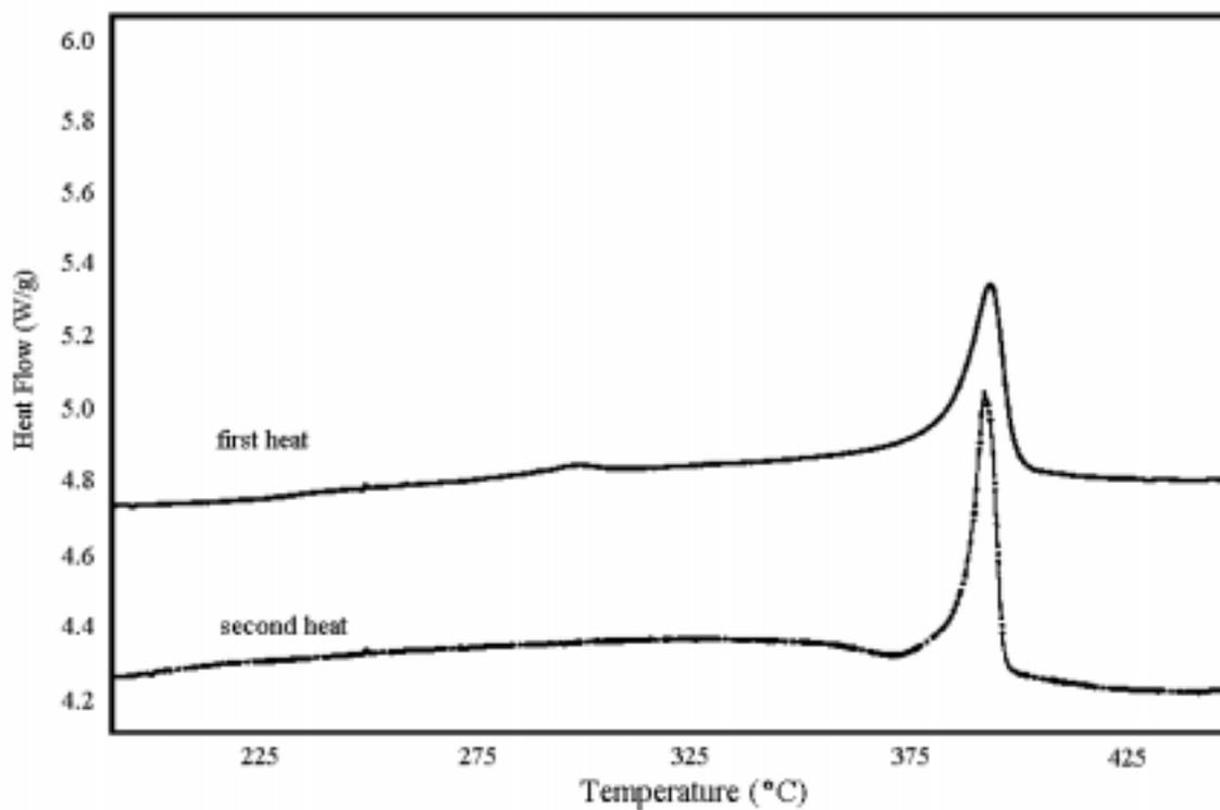
Figure 4.3.2.2.1: DSC Thermograms of 30,000 g/mole TPER-BPDA-PA at 10°C/min
