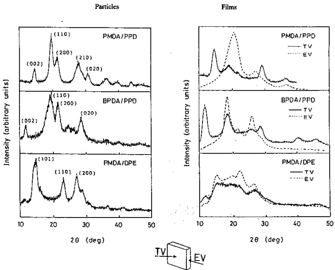
Figure 2.5.18: X-ray Diffractograms of Polyimide Particles and Films<sup>182</sup>
