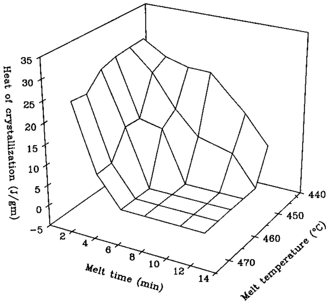
Figure 4.2.2.9: Effect of Temperature and Time in the Melt under Nitrogen on the Heat of Crystallization of 10K (300°C) TPEQ-ODPA-PA<sup>224,235</sup>
