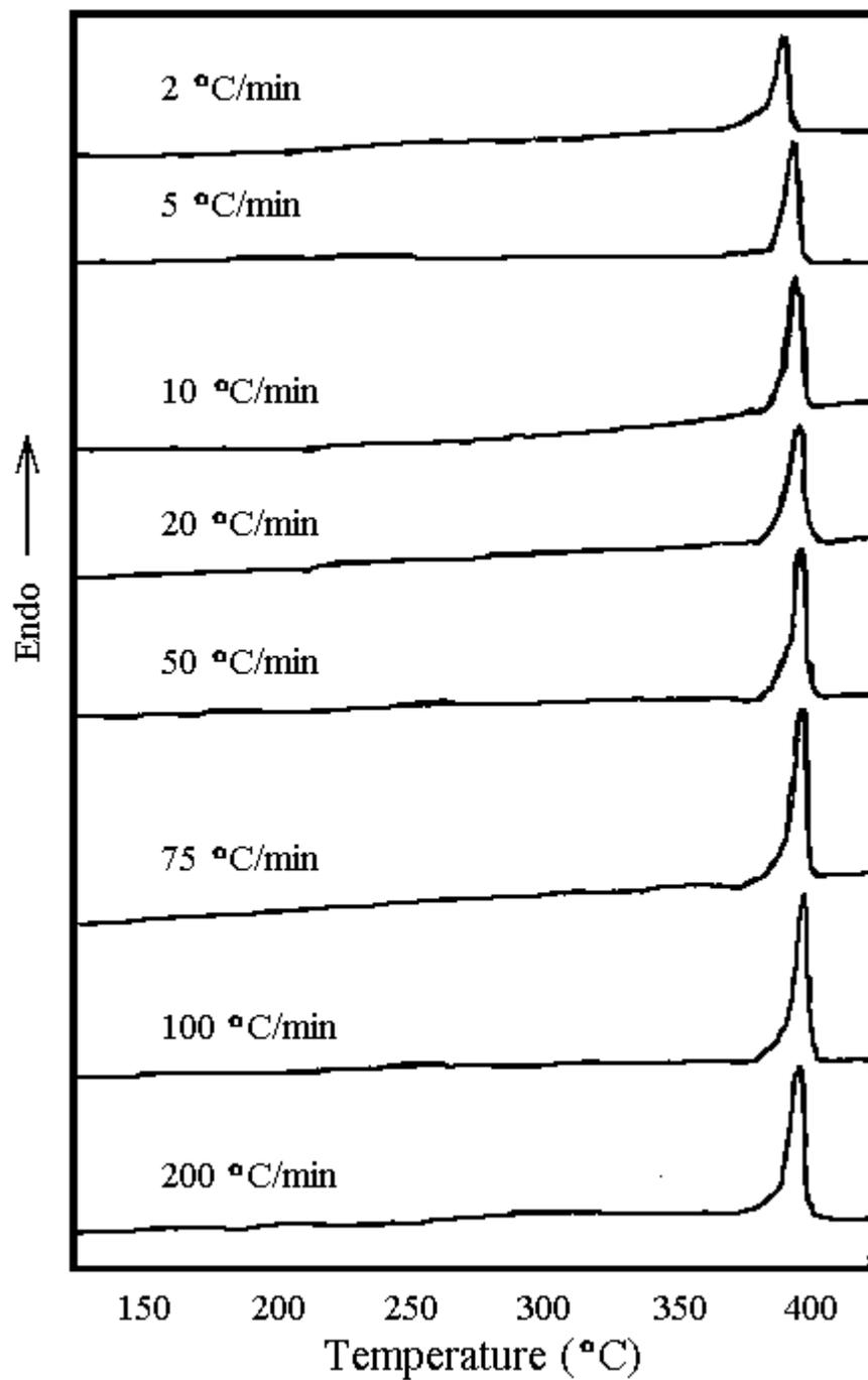
Figure 4.3.2.2.5: Influence of Cooling Rate on the DSC Thermograms of TPER-BPDA-PA Polyimide
