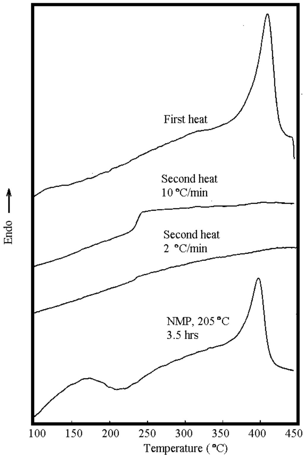
Figure 4.2.2.7: DSC Thermograms of 30K TPEQ-ODPA-PA at 10°C/min
