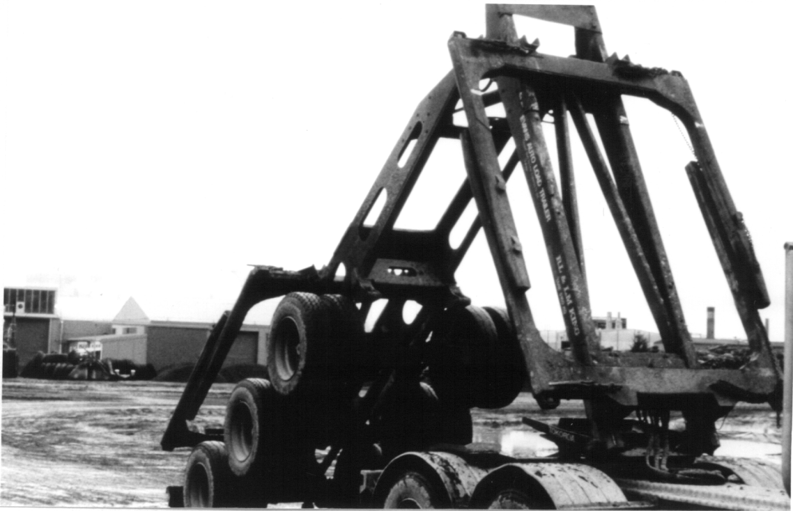
Figure 8. Self Loading Sequence for Evans Folding Frame Trailer: Loading trailer on the tractor.
