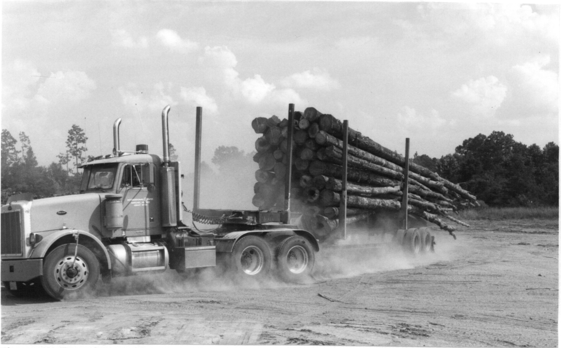
Figure 60. Experimental Stress Analysis of the Gooseneck Trailer: Simulating extreme situations--hard braking.
