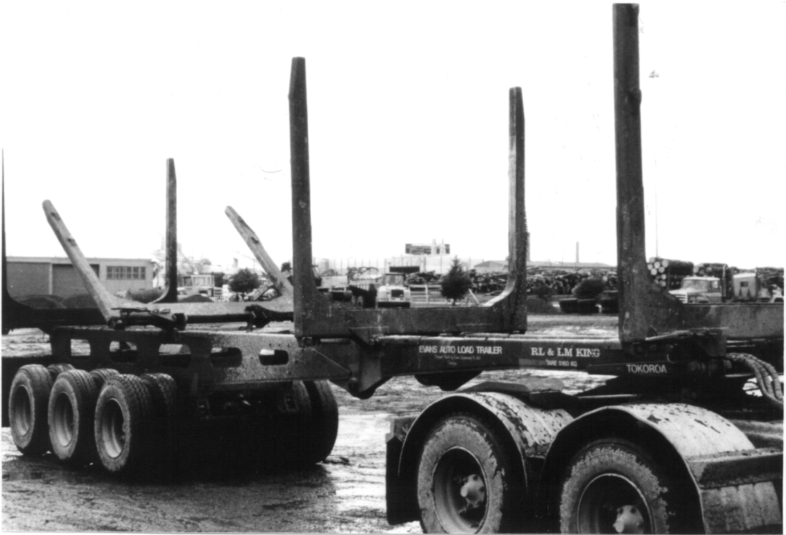
Figure 4. Self Loading Sequence for Evans Folding Frame Trailer: Folding the third bolster and standards.
