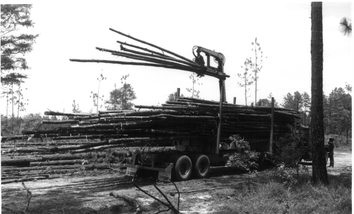
Figure 62. Experimental Stress Analysis of the Gooseneck Trailer: Monitoring the dynamic loading and the resultant stresses at critical locations--loading with a Barko 160A knuckle-boom loader on in-woods landing.
