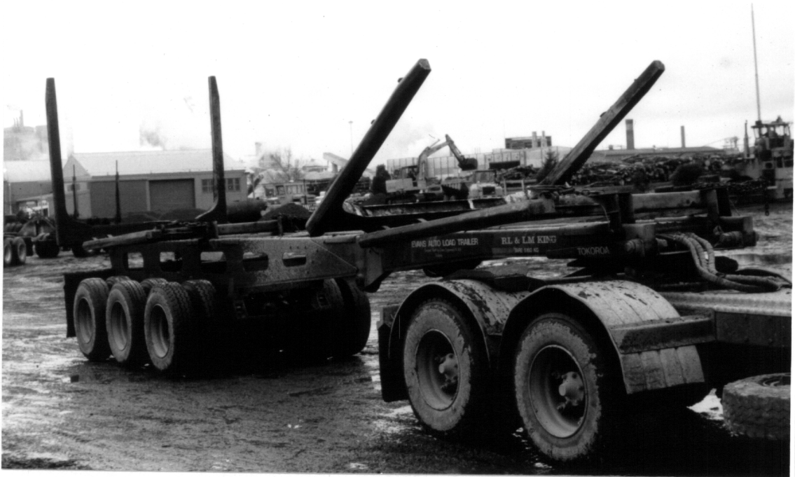
Figure 5. Self Loading Sequence for Evans Folding Frame Trailer: Folding the front and then the second bolsters and standards.
