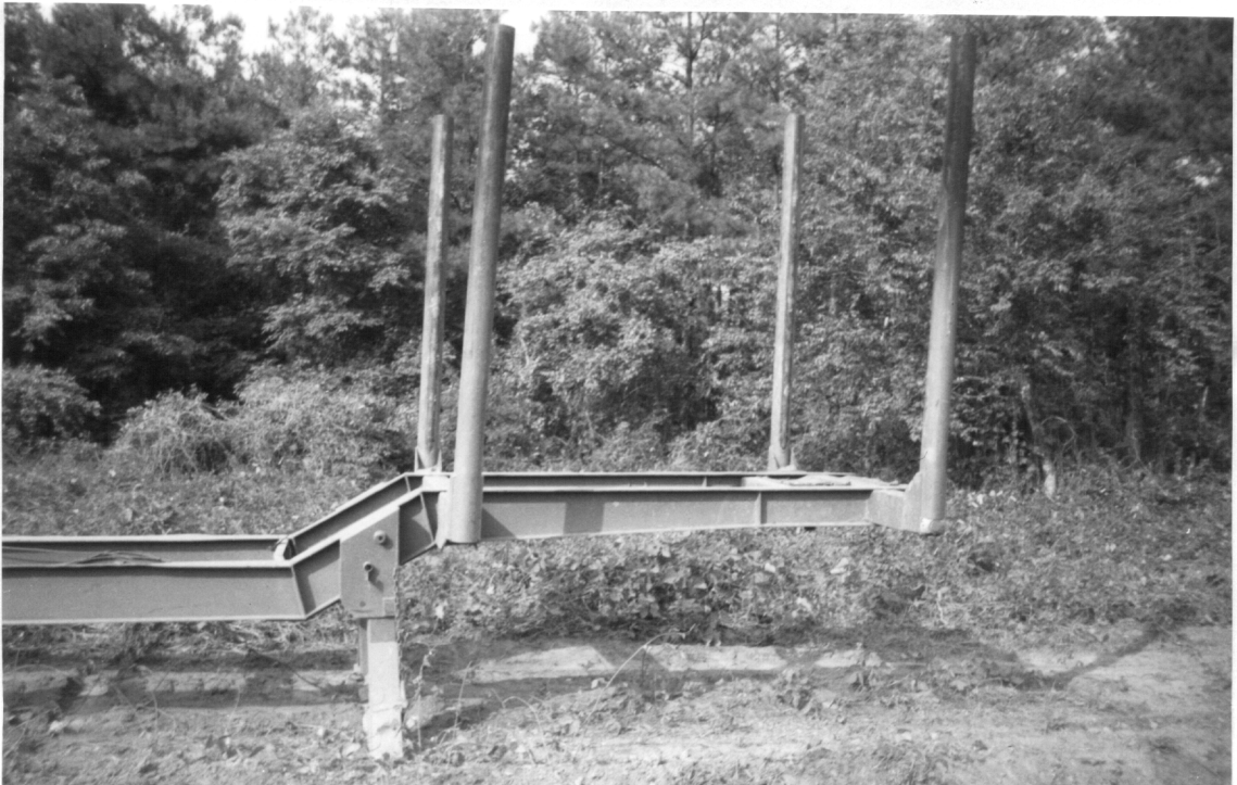
Figure 25. Double-Drop Trailer: Trailer's neck.
