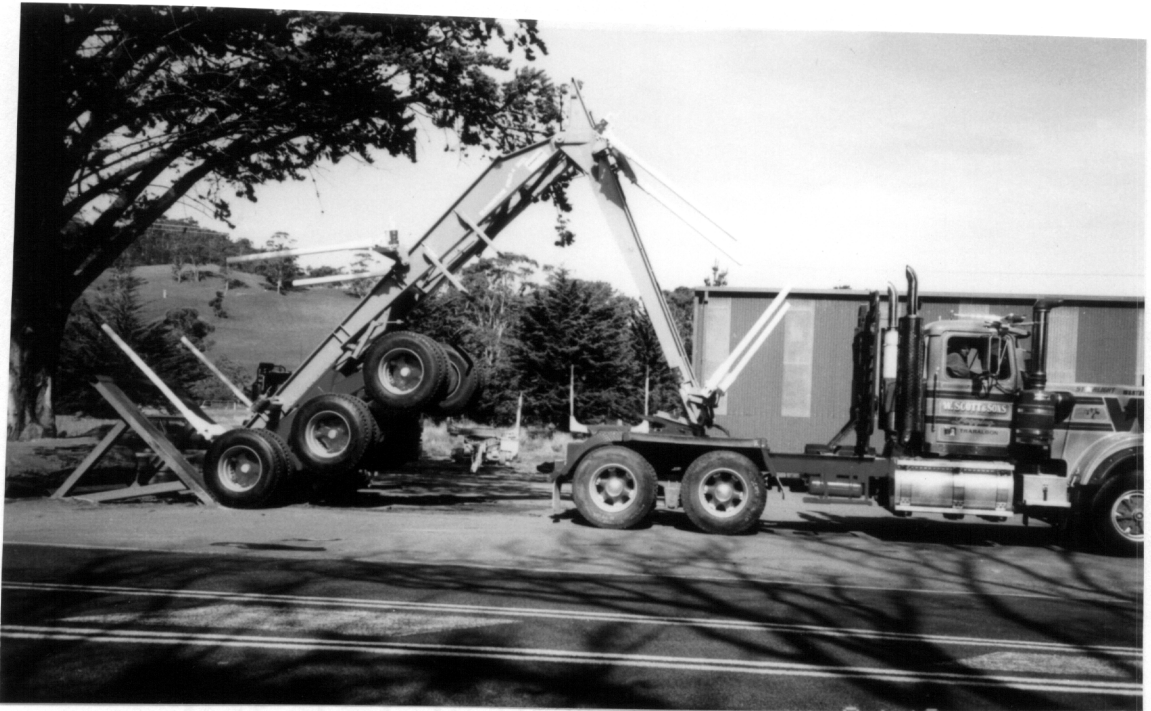
Figure 15. Self Loading Sequence for "Fold-A-Skel" Trailer: When trailer folds, bolsters close automatically by means of a special mechanism.
