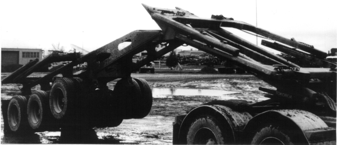
Figure 7. Self Loading Sequence for Evans Folding Frame Trailer: Folding frame.
