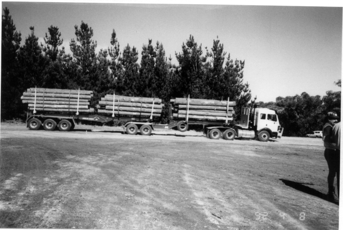
Figure 18. "B-Double" Trailer: Combination of the two "Fold-A-Skel" trailers.
