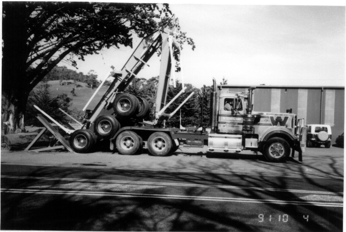
Figure 16. Self Loading Sequence for "Fold-A-Skel" Trailer: Now a driver releases trailer breaks while still reversing the truck.
