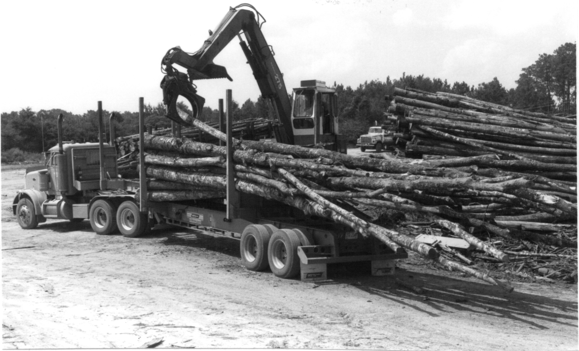
Figure 61. Experimental Stress Analysis of the Gooseneck Trailer: Simulating extreme situations--loading with a knuckle-boom loader.
