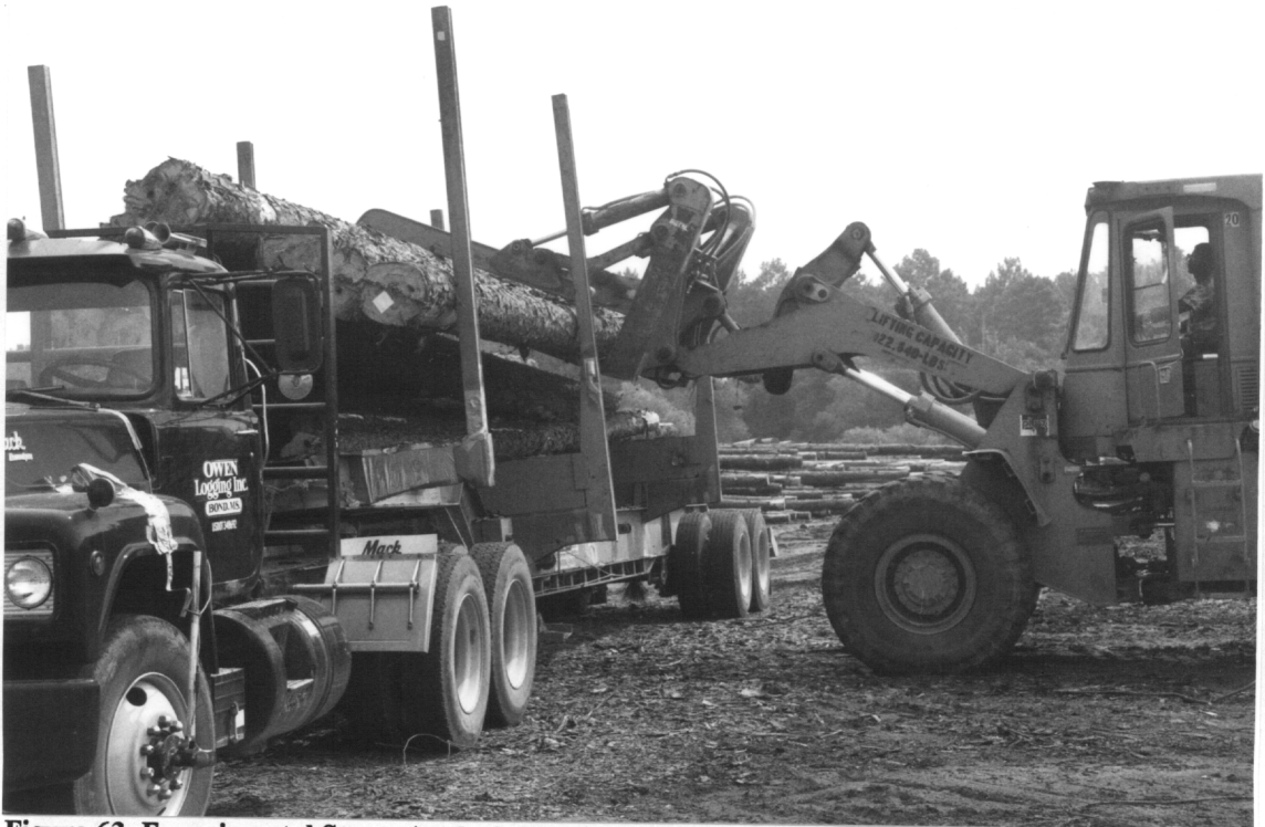
Figure 63. Experimental Stress Analysis of the Gooseneck Trailer: Monitoring the dynamic loading and the resultant stresses at critical locations--unloading with a Cat front-end loader at the pole plant.
