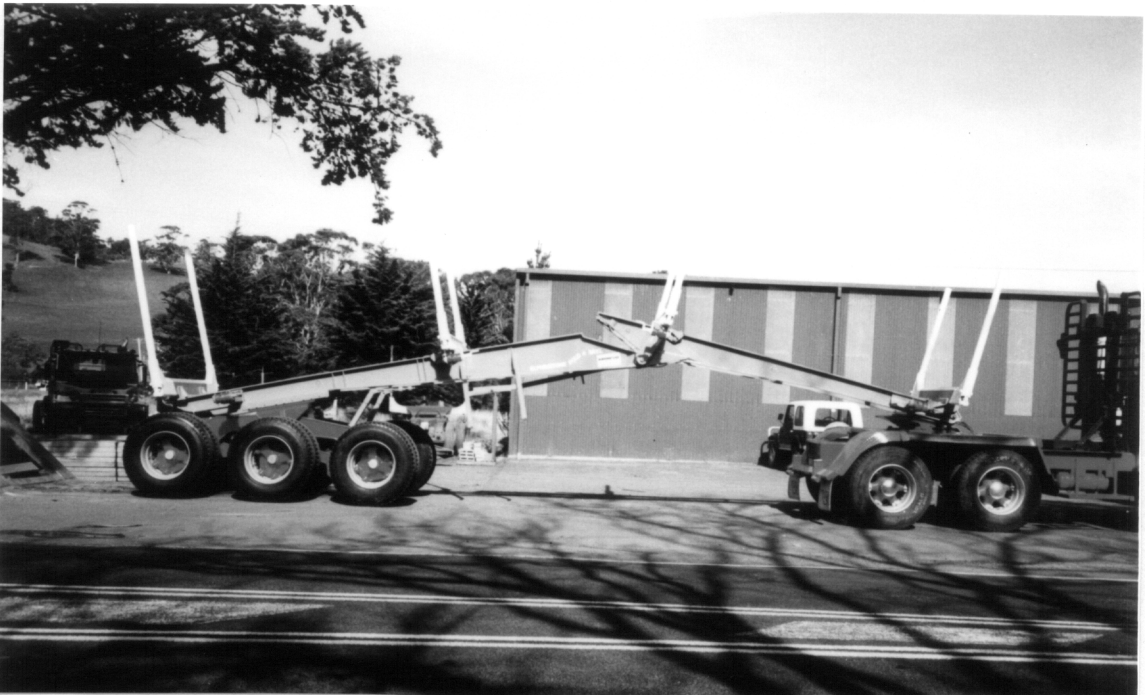
Figure 14. Self Loading Sequence for "Fold-A-Skel" Trailer: Moving from the ramp after initial breaking the beams.
