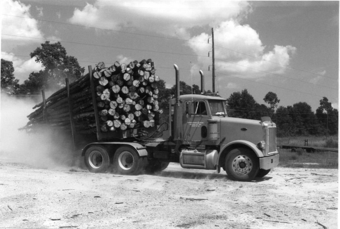
Figure 59. Experimental Stress Analysis of the Gooseneck Trailer: Simulating extreme situations--hard cornering.
