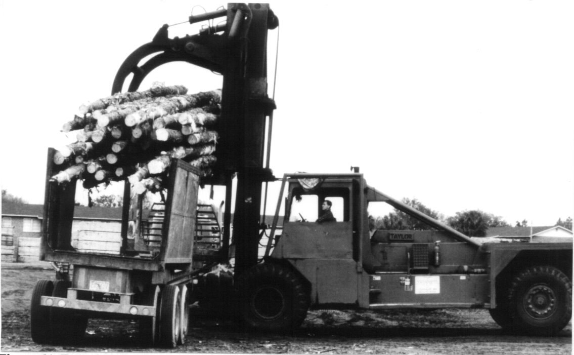
Figure 64. Experimental Stress Analysis of the Full-Tree Trailer: Monitoring the dynamic loading and the resultant stresses at critical locations--unloading with a forklift on the sawmill wood yard.
