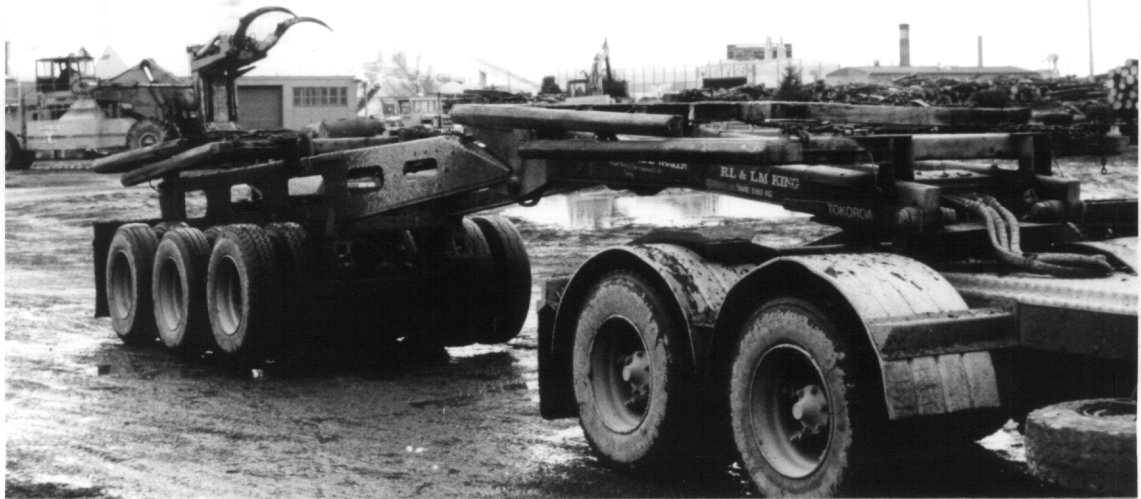
Figure 6. Self Loading Sequence for Evans Folding Frame Trailer: Breaking the frame--operation consists of breaking the frame with the aid of two hydraulic cylinders, backing up the tractor while the trailer brakes are engaged.
