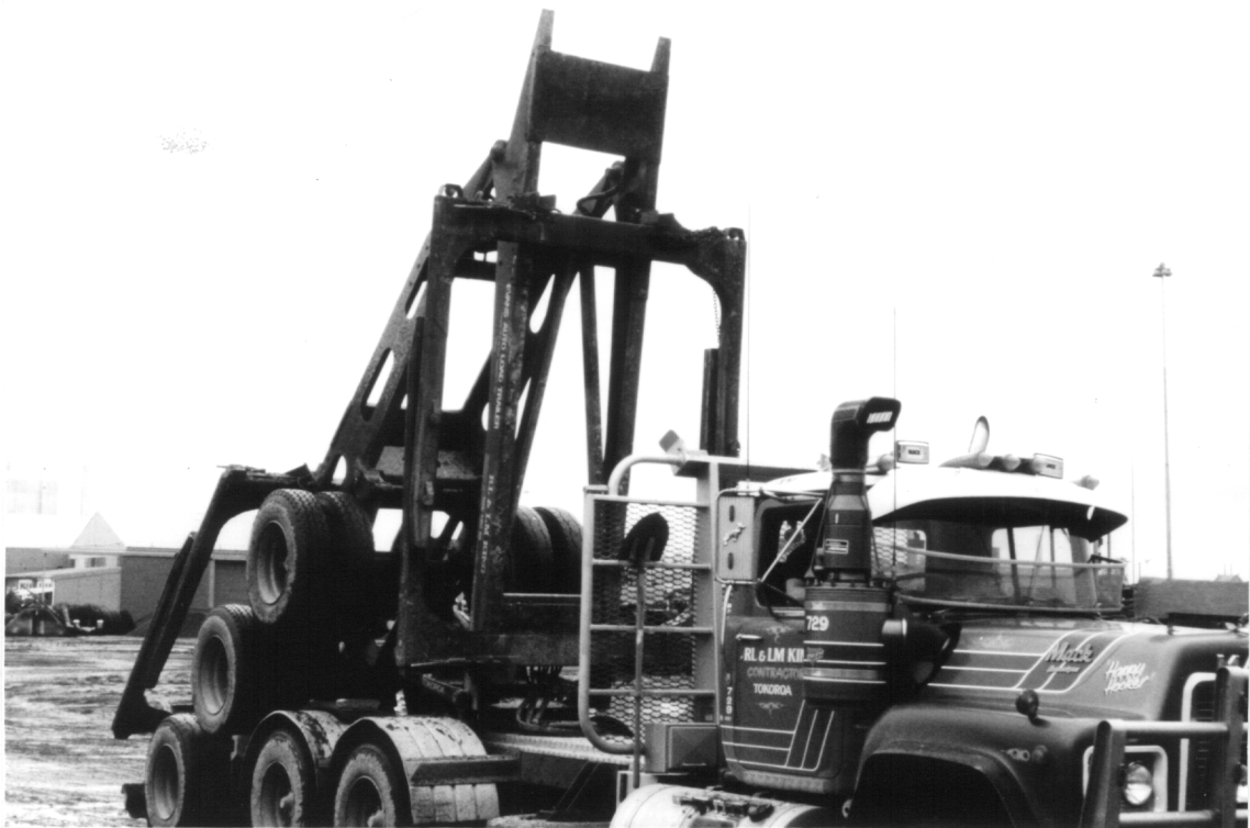
Figure 9. Self Loading Sequence for Evans Folding Frame Trailer: The final phase of loading-- hydraulic cylinders are engaged once again to put the trailer finally in place.
