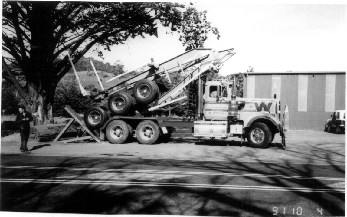
Figure 17. Self Loading Sequence for "Fold-A-Skel" Trailer: Trailer loaded on the tractor.
