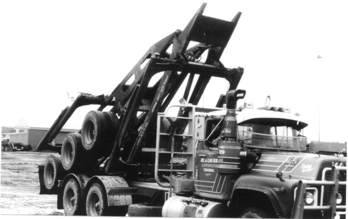
Figure 10. Self Loading Sequence for Evans Folding Frame Trailer: Trailer loaded on tractor and ready for a return trip.
