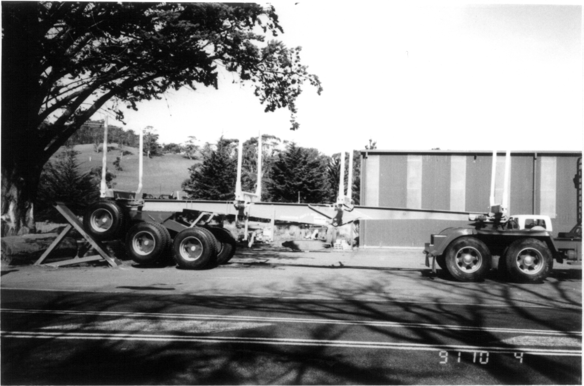
Figure 13. Self Loading Sequence for "Fold-A-Skel" Trailer: Backing up on a ramp to engage the beam breakers.
