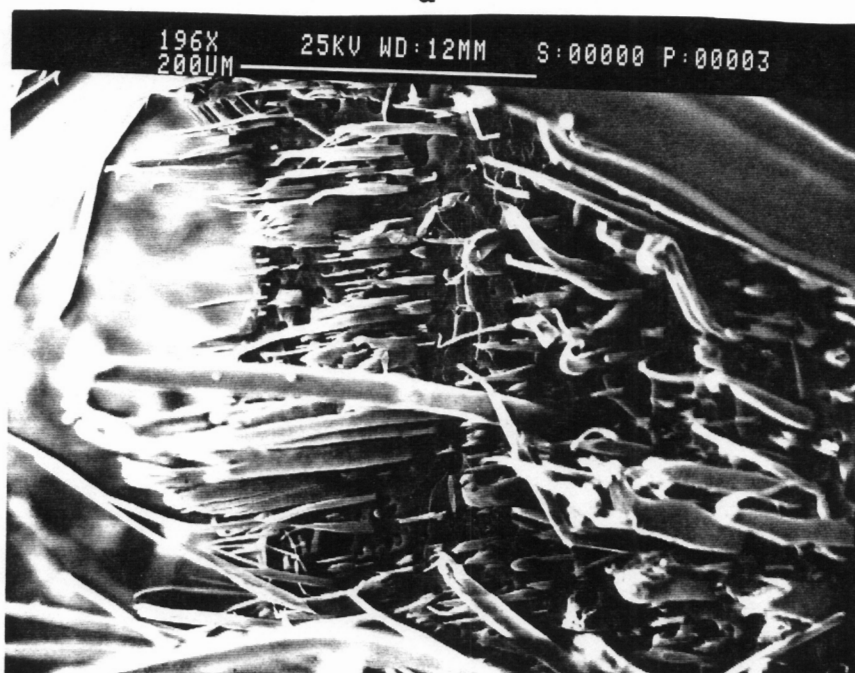
Figure 92. SEM micrographs of fracture surface of PP/Vectra A 75/25 (MB) strand at magnifications of (a) 120X and (b) 196X. Fracture is across the flow direction.
