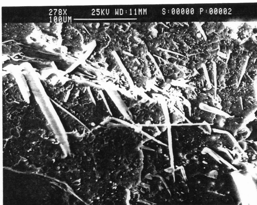
Figure 56. Scanning electron micrographs of fracture surfaces of PET/Ultrax 80/20 MB blend strands at draw ratios of (a) 1 and (b) 13.7. Fracture is across the flow direction.
