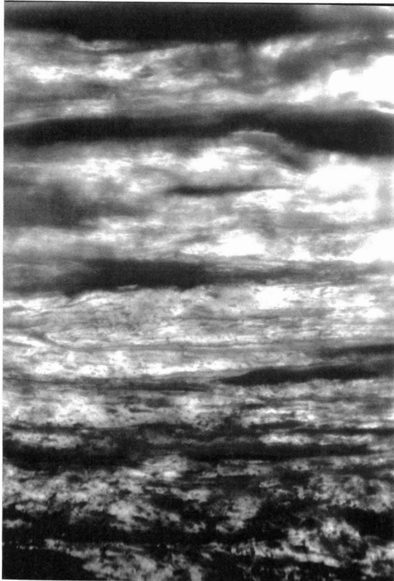
Fig. 4-7 Optical photograph of 2.3 mm thick plaque with a flexural modulus of 4.1 GPa molded in 7.8 seconds: (a) entire plaque; (b) skin/subskin region.
