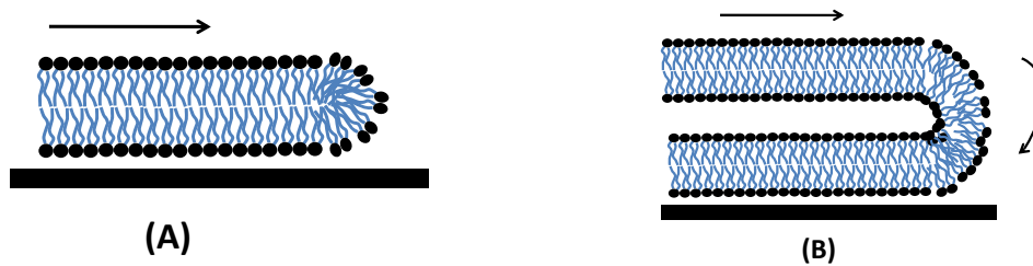
Figure 2.11. Two different types of spreading of lipid layers onto a solid substrate. (A) A single bilayer formed by sliding with a nearly straight front on a surface. (B) Finger-like lobes of juxtaposed bilayers (rolling motion) on a solid surface.
