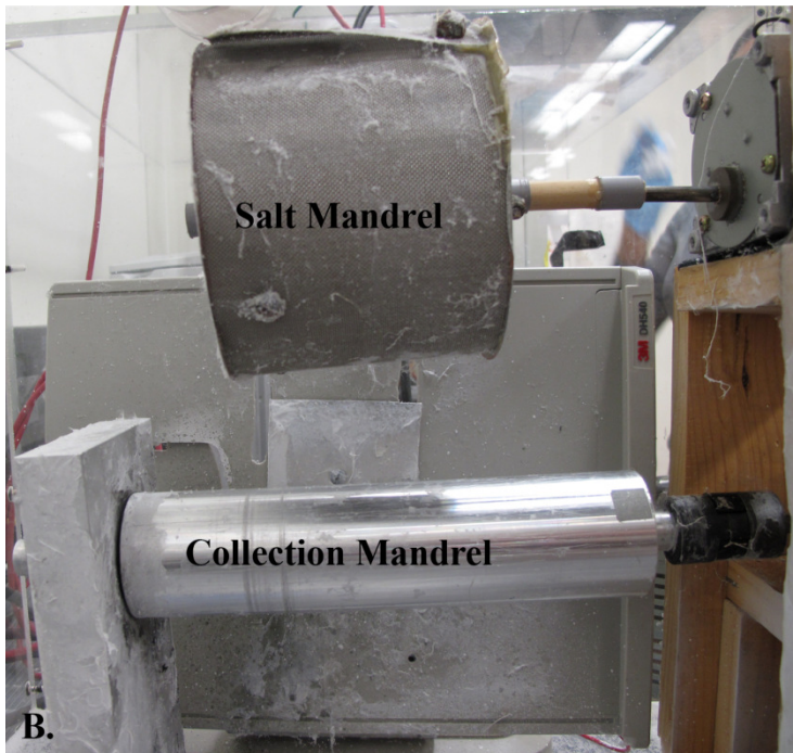
Figure 2.1. A. Schematic of NaCl addition during electrospinning and B. a picture of the salt and collection mandrels used.
