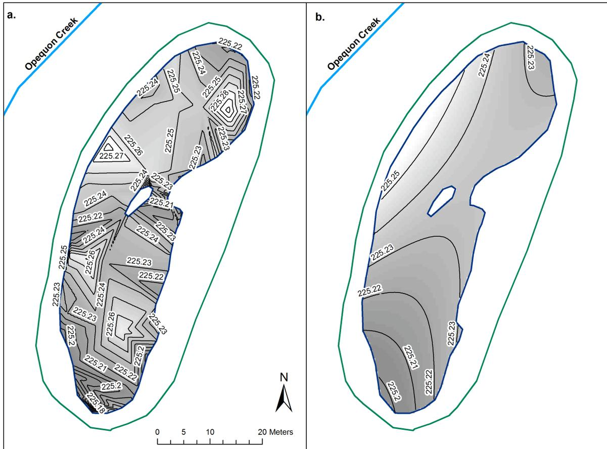
**Figure 6.3 Measured water surface slope a. interpolated using triangulated irregular network (TIN) interpolation and b. trend surface analysis.** (elevation in m, vertical datum NAVD 88)
