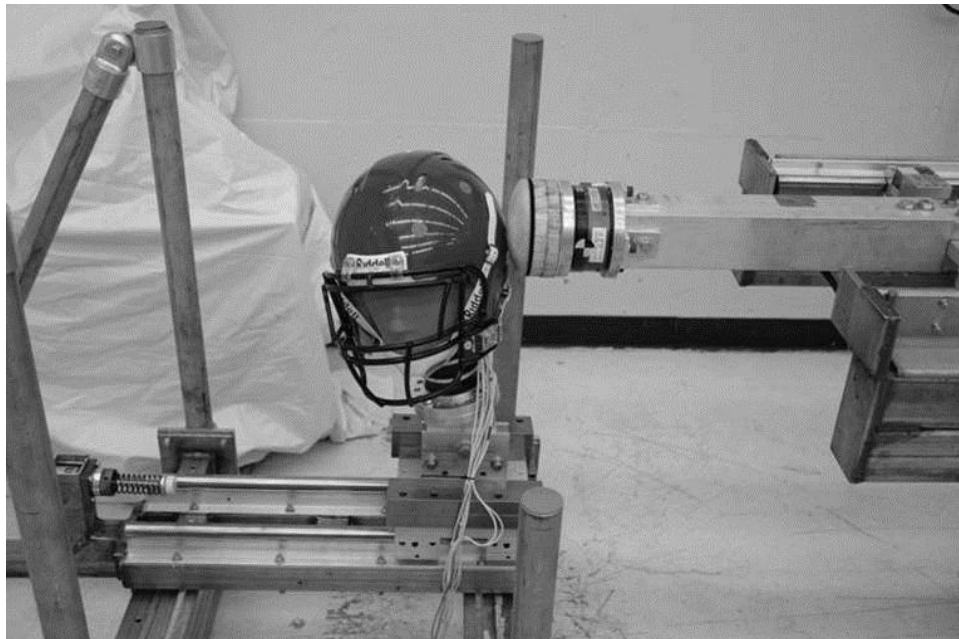
Figure 10: Pneumatic linear impactor and helmeted Hybrid III head mounted on the linear slide table.
