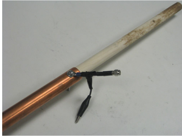
(b) Base of the monopole
