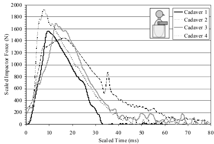
Figure 97: Scaled impactor force time history for non-destructive tests- Ribs: Arm 90.
