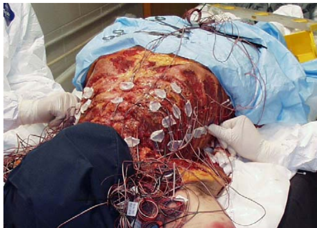
Figure 64: Example thoracic strain gage attachment for belt loading tests.
