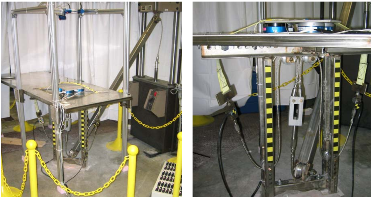
Figure 68: Oblique views of actual belt loading system.
