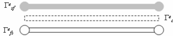
Figure 3.4 Coupling of the base structure mesh along the structure-fluid boundary, \Gamma_{sf}^e to the base fluid mesh along the fluid-structure boundary, \Gamma_{fs}^e
