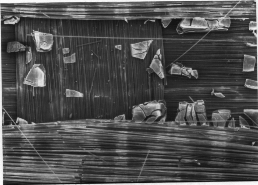
Figure 2. Example of gripped affected zone: (A) gripped and (B) gage section.
