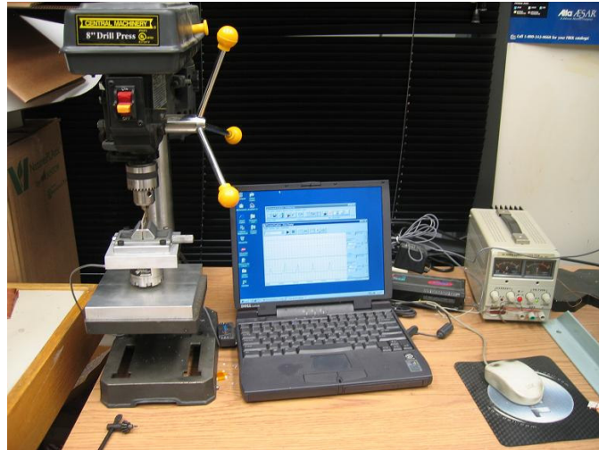
Figure 2.15. Setup to measure die-shear strength.
