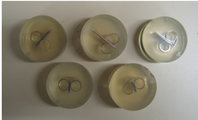
Figure 2.23. Fine polished samples.
