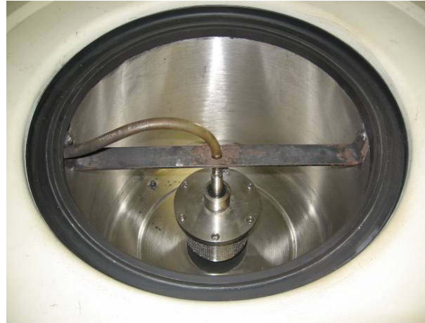
Figure 2.4 Sealed compartment of the Beckman centrifuge machine
