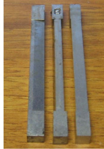
Figure 2.8 Different sides of tungsten carbide bars used to build the screen section
