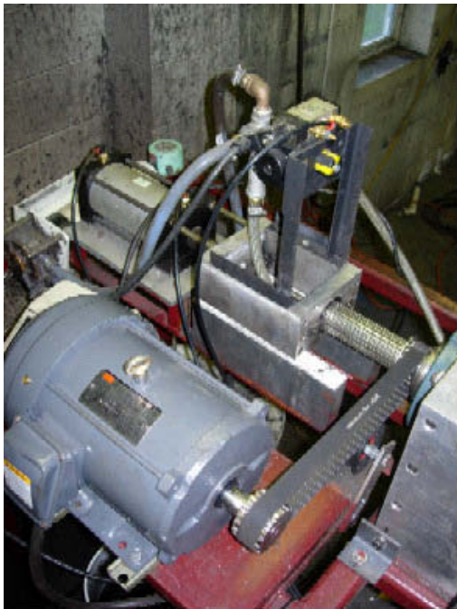
Figure 3.6 Valve system for the introduction of feed slurry and air
