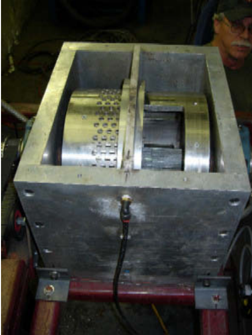
Figure 3.4 Rotating drum assembly for the pilot-scale centrifuge
