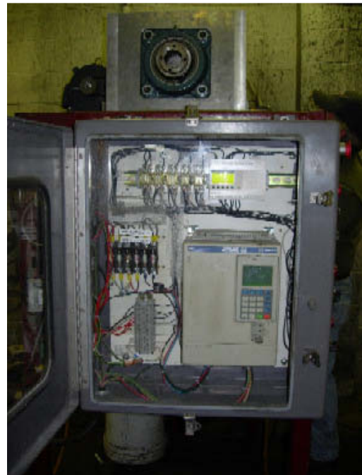
Figure 3.7 Electronic control panel for the pilot-scale centrifuge
