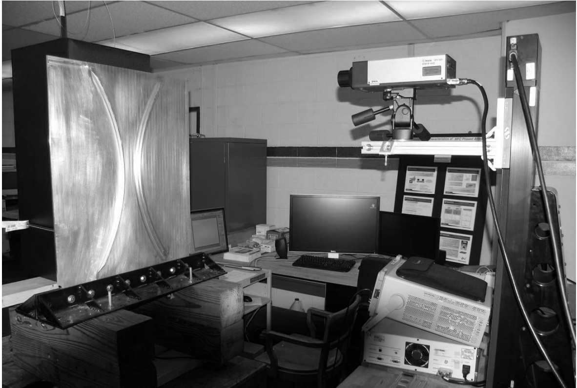
Fig. 3-6 Laser vibrometer and support equipment in place for testing, photo taken by author, 2011.
