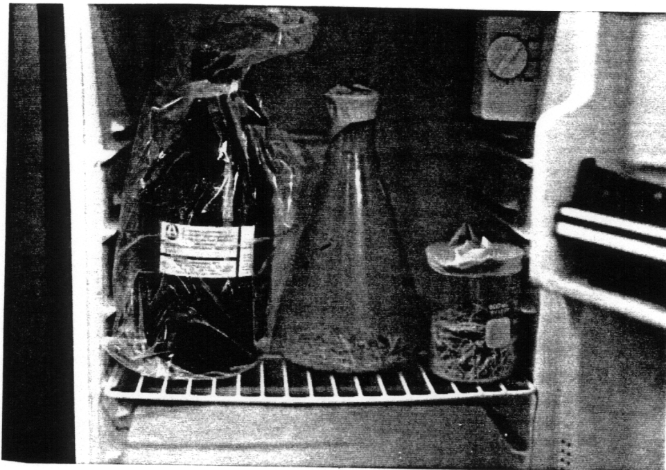
Photo 33. Storage tests were used to determine long-term effects of storing filled fibers. Here, they are stored in a refrigerated environment.
