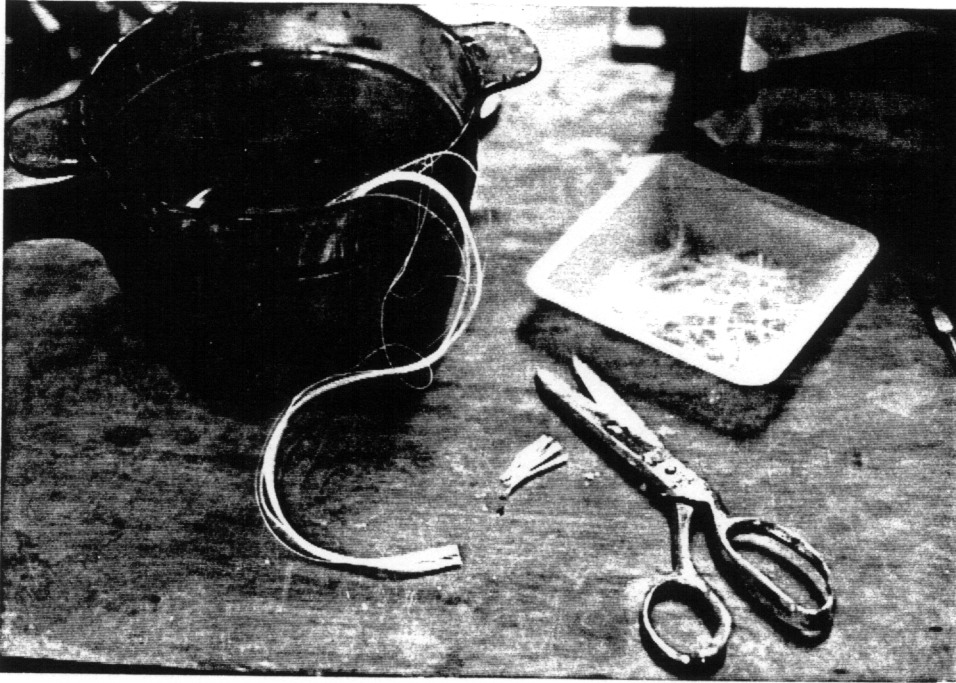
Photo 3. The porous fibers are coated with wax before cutting into 1" lengths.
