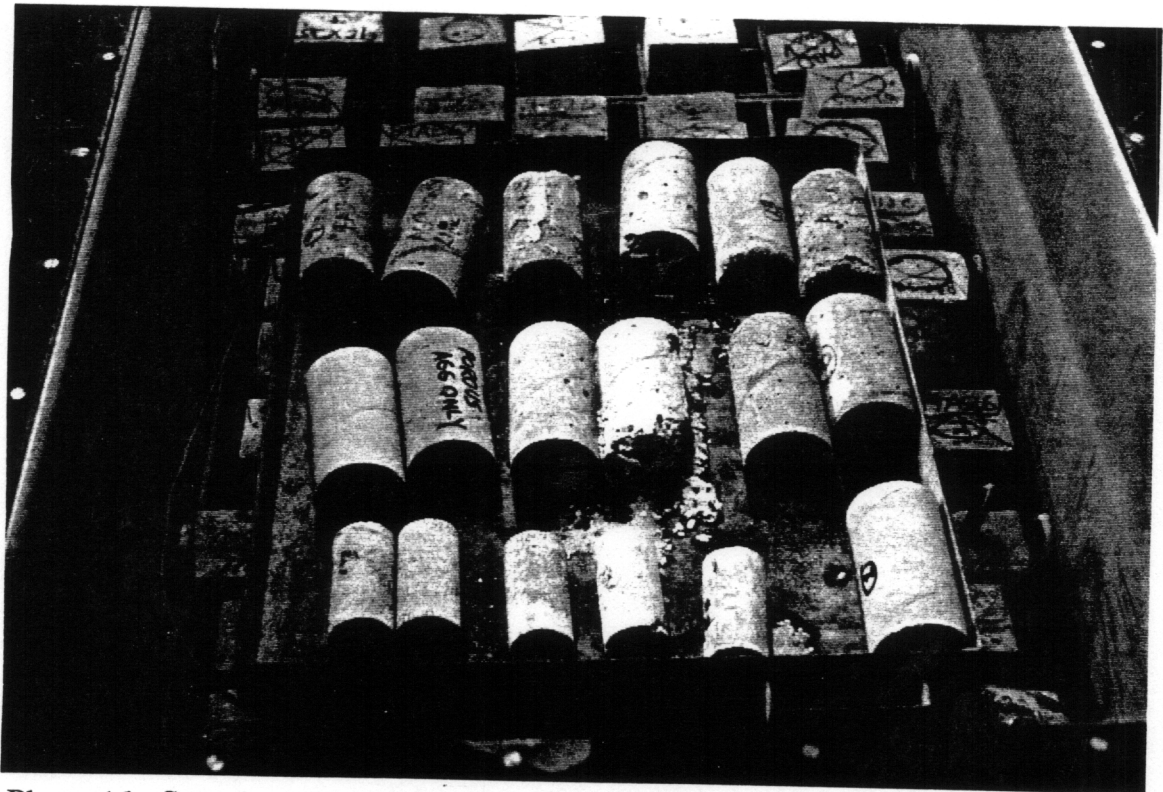
Photo 16. Samples are tested for freeze/thaw damage in the Logan machine.
