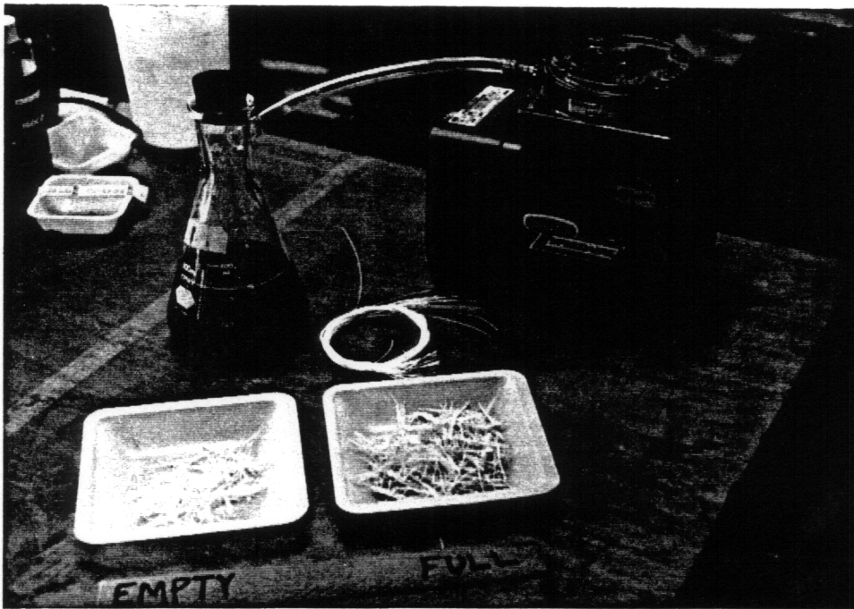
Photo 4. Filled fibers are cut in 1-inch lengths.
