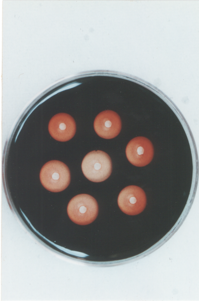
Fig. 5.3. Gel diffusion assay showing endo- \beta -mannanase-like activity on plates with locust bean galactomannan substrate in agarose gel using Congo red dye. The wells contain 4 \mu l of crude leachate from perisperm tissue adjacent to the radicle tip.
