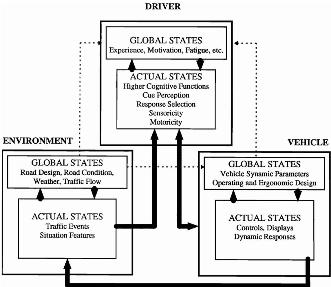
Figure 2. Interaction of the subsystems driver, vehicle and environment (from Kramer and Rohr, 1982).
