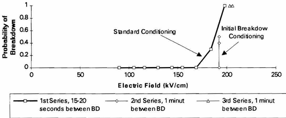
Figure 4.8 Test run of 9/9/93. Note the heavy line depicting the standard conditioning curve. Also note that the standard-conditioning curves allowed only a short time (i.e. 15-20 seconds) to elapse between breakdowns; while a longer time (i.e., 1 minute) was allowed between breakdowns for the IB-conditioning curves.
