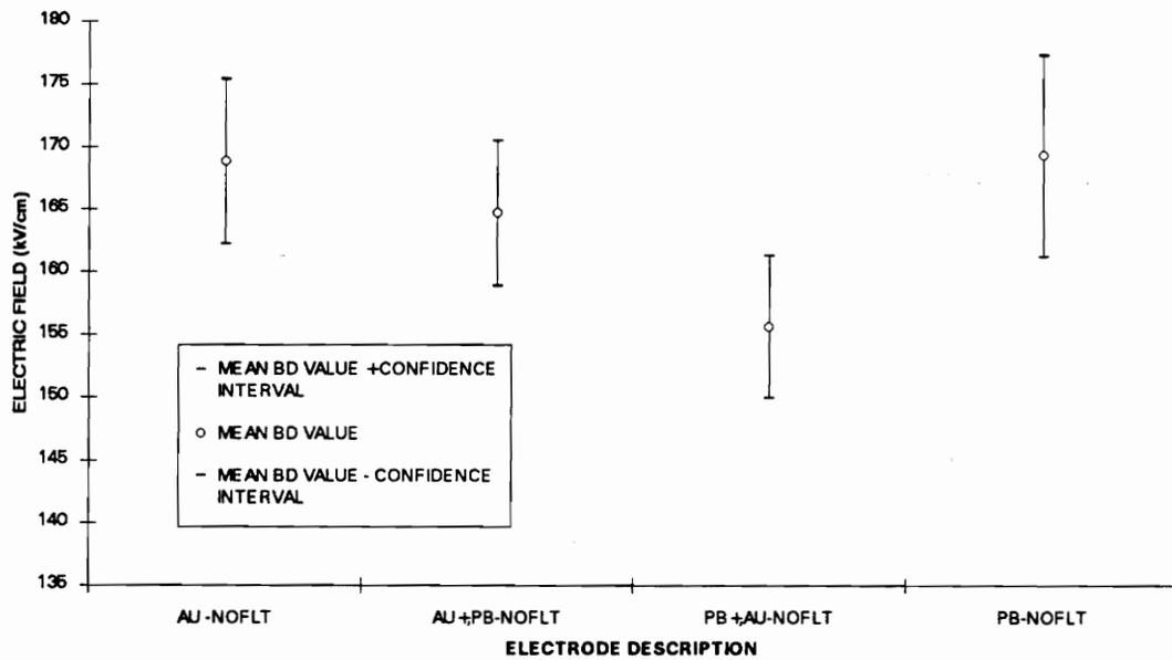
Figure 5.4 Plot of the mean breakdown field plus or minus the 95% confidence interval for pure gold, pure lead and mixed electrodes, with no filters.
