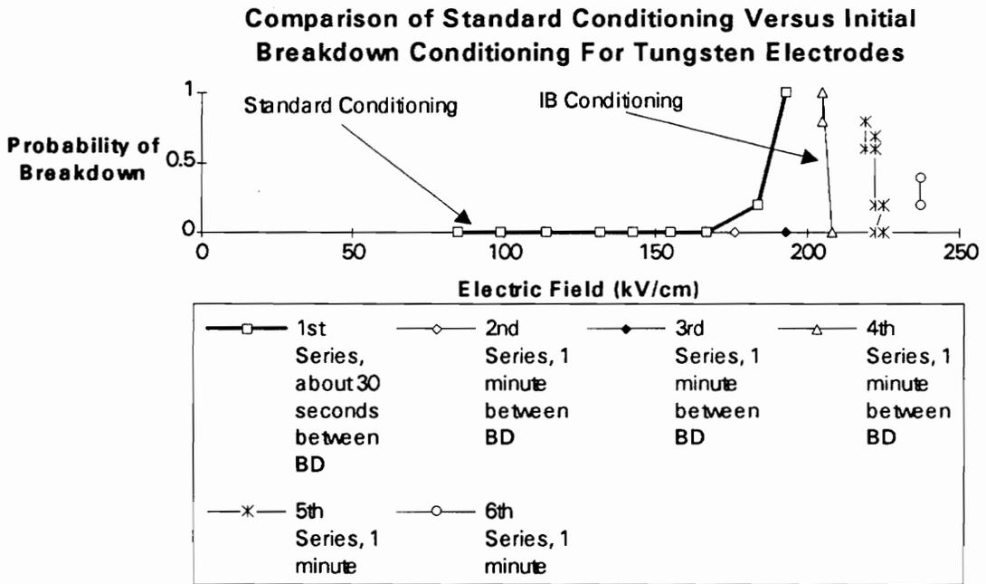
Figure 4.12 Test run of 10/05/93. Note the heavy line depicting the standard conditioning curve. This was the first attempt at IB conditioning on tungsten electrodes. Also note that 1 minute was allowed between breakdown for the IB conditioning curves. Some of the lines are not vertical because the applied voltage strays slightly about the set point due to variations in the charging circuitry.
