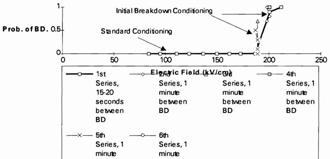
Figure 4.9 Test run of 9/10/93. Note the heavy line depicting the standard conditioning curve. Also note that the IB-conditioning curves use a longer time (i.e., 1 minute) between breakdown. Some of the lines are not vertical because the applied voltage strays slightly about the set point due to variations in the charging circuitry.
