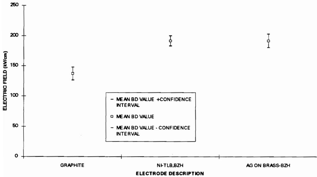
Figure 5.9 Plot of the mean breakdown field plus or minus the 95% confidence interval for graphite, nickel and silver electrodes, with filters.
