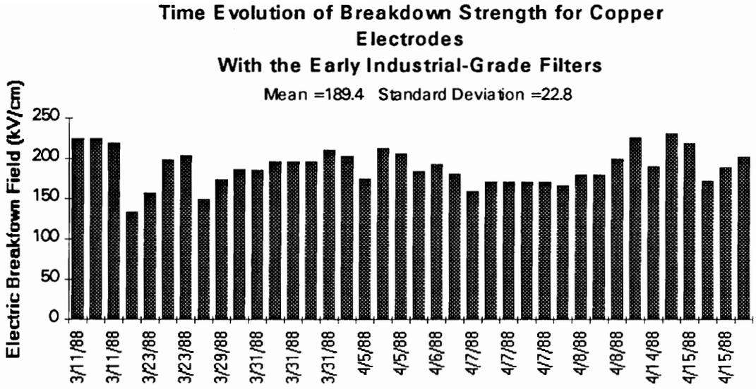
Figure 4.2 Breakdown data for copper electrodes with industrial-grade particulate filters and a Barnstead organic filter. Note the erratic behavior after the initial runs on 3/11/88.
