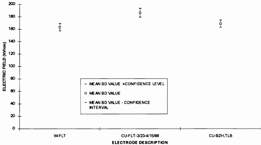
Figure 5.8 Plot of the mean breakdown field plus or minus the 95% confidence interval for tungsten and other copper electrodes, with filters.
