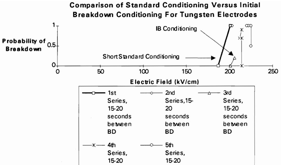
Figure 4.13 Test run of 10/06/93. Note the abbreviated standard-conditioning curve. Also note that only 15-20 seconds was allowed between breakdown for the IB conditioning curves. Some of the lines are not vertical because the applied voltage strays slightly about the set point due to variations in the charging circuitry.
