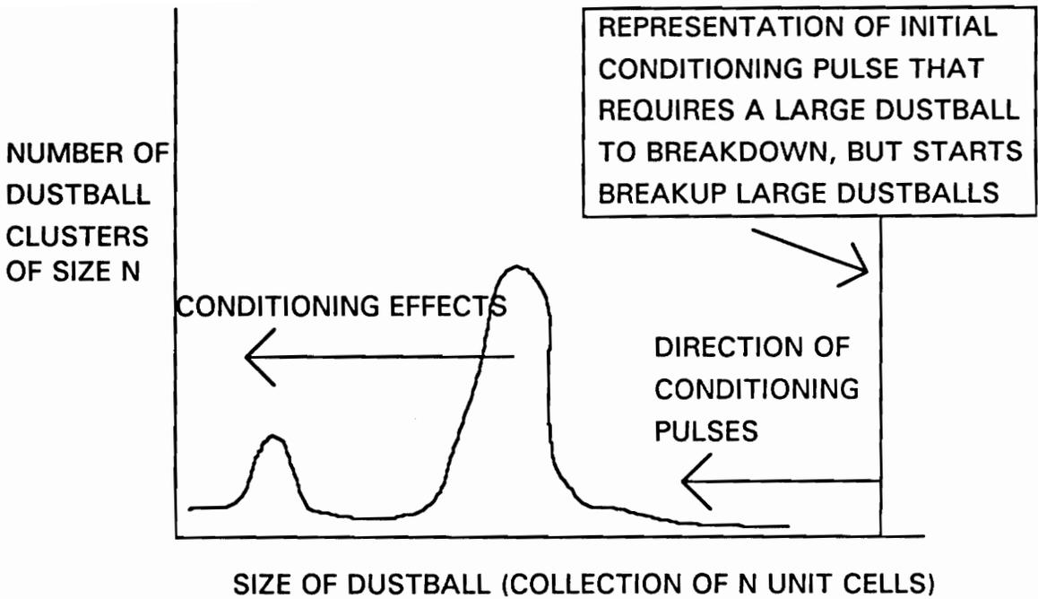
Figure 5.23. Schematic representation of a more developed idea about the mechanism of conditioning.
