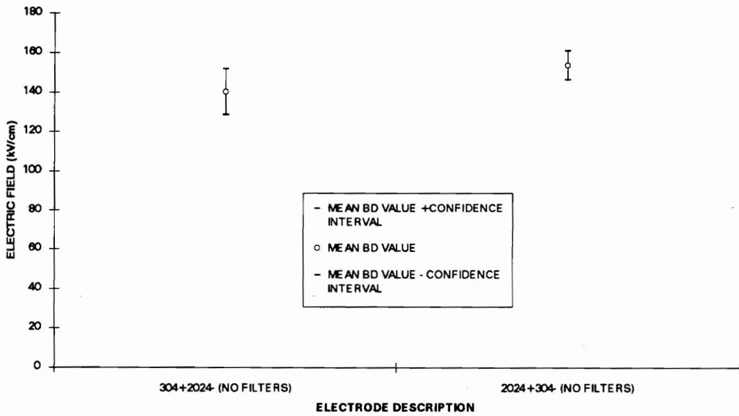
Figure 5.3 Plot of the mean breakdown field plus or minus the 95% confidence interval for 304 stainless steel, 2024 aluminum electrode sets with no filters.
