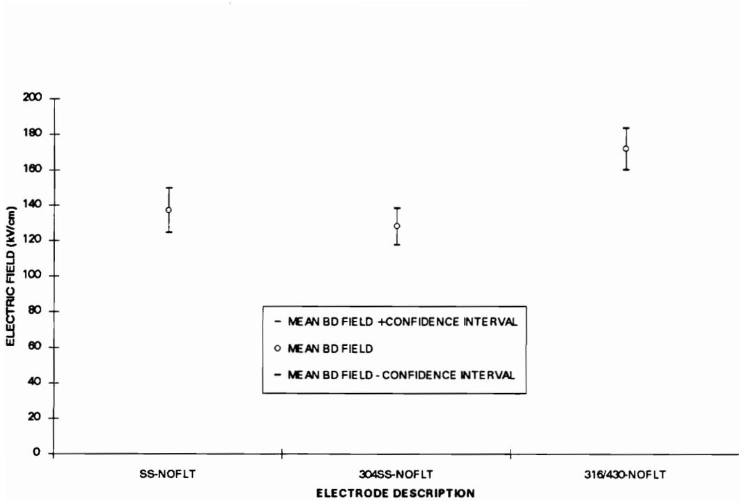
Figure 5.1 Plot of the mean breakdown field plus or minus the 95% confidence interval for stainless-steel electrodes with no filters.
