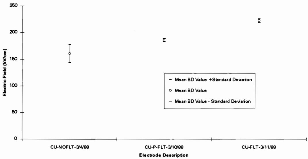
Figure 4.1 Plot of the mean breakdown field plus or minus the 95% confidence interval for a series of experiments on copper demonstrating the efficacy of various industrial-grade filter combinations. On the left is no filters, in the center is only particulate filters, and on the right is the combination of particulate plus organic filter.
