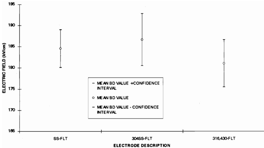
Figure 5.5 Plot of the mean breakdown field plus or minus the 95% confidence interval for stainless steel electrodes, with filters.
