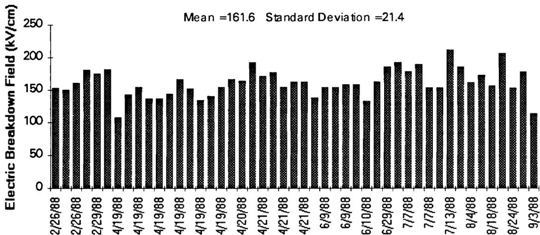
Figure 4.3 Breakdown data for tungsten electrodes with industrial-grade particulate filters and a Barnstead organic filter. Note the erratic behavior.
