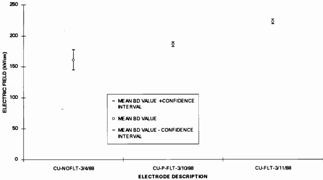
Figure 5.7 Plot of the mean breakdown field plus or minus the 95% confidence interval for a series of experiments on copper demonstrating the efficacy of various filter combinations. On the left is no filters, in the center is only particulate filters, and on the right is the combination of particulate plus organic filter.
