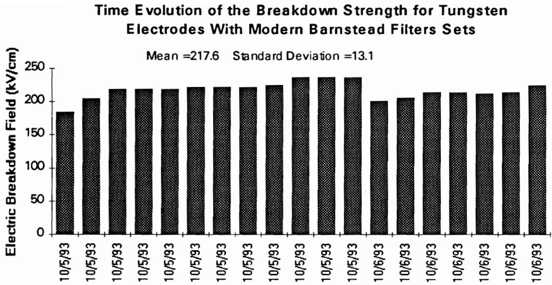
Figure 4.5 Breakdown data for tungsten electrodes with modern Barnstead particulate and organic filters. Note the more consistent breakdown behavior as compared to Figure 4.3.
