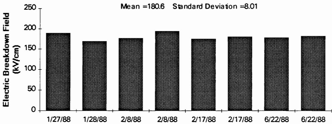
Figure 4.4 Breakdown data for stainless-steel electrodes with industrial-grade particulate filters and a Barnstead organic filter. Note the consistent breakdown behavior.
