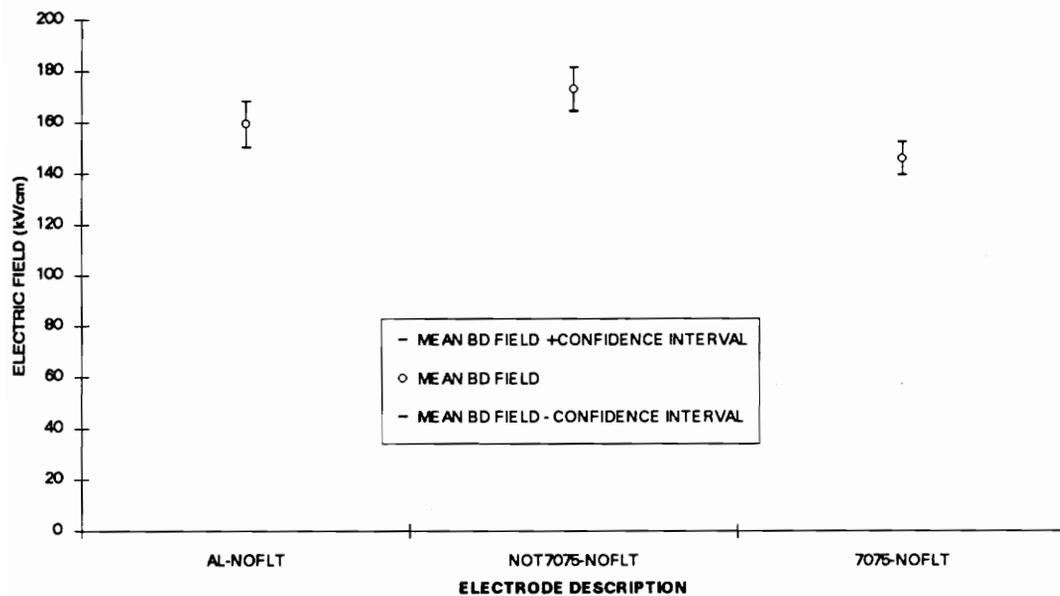
Figure 5.2 Plot of the mean breakdown field plus or minus the 95% confidence interval for aluminum electrodes with no filters.
