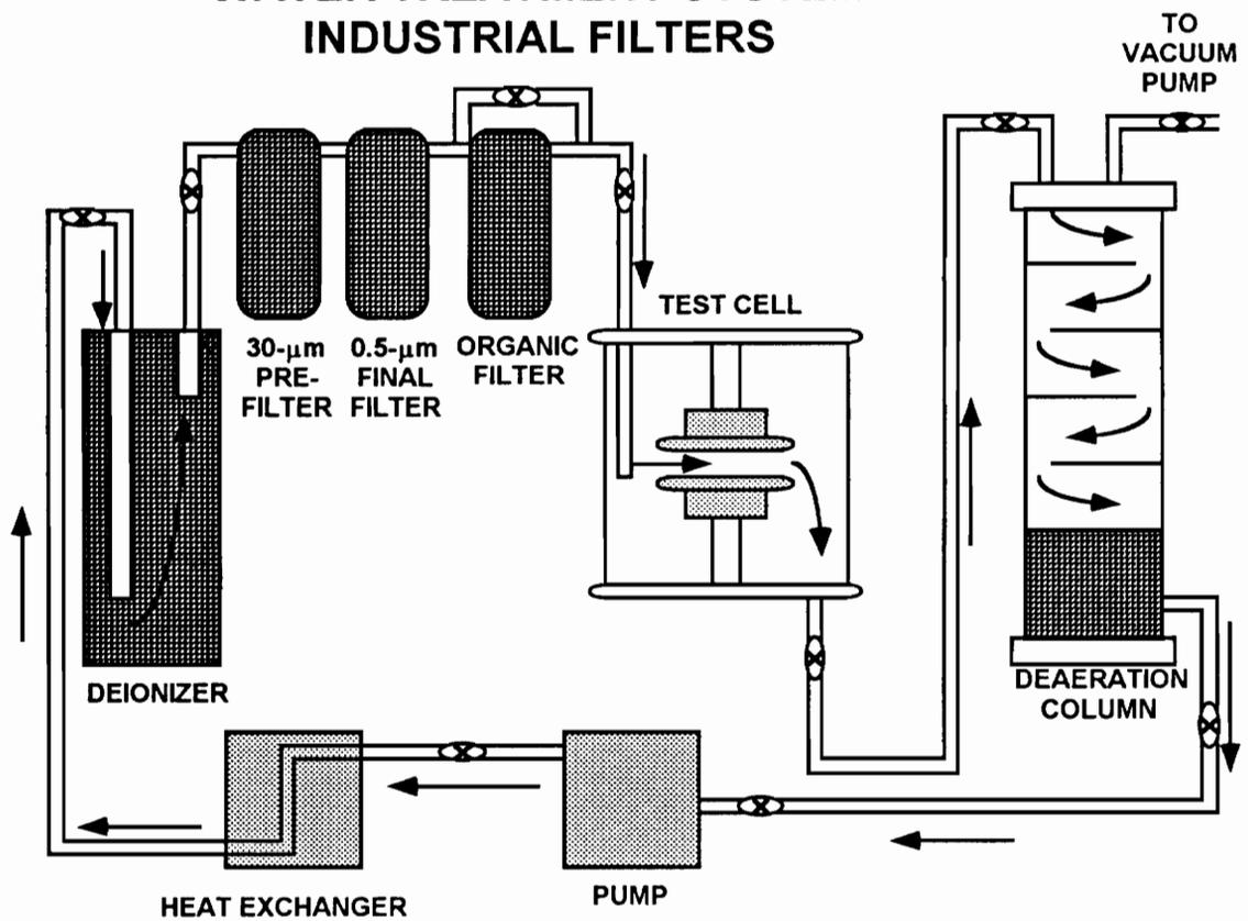
Figure 3.1 The sketch of the older, industrial-grade water-treatment apparatus for the electrical-impulse, water-breakdown experiment.
