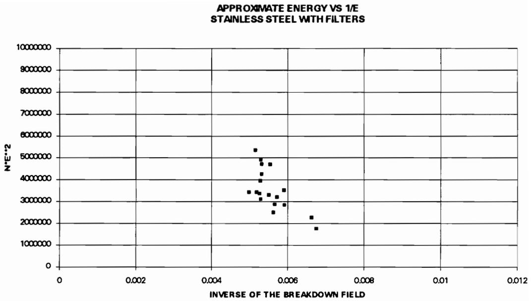
Figure 5.16. Same plot for filters and stainless steel electrodes.
