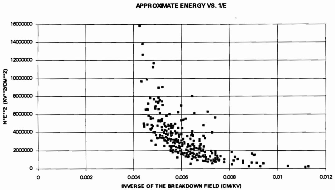
Figure 5.11. The plot of approximate energy (arbitrary units) versus  $1/E$  for all the experiments in the database.
