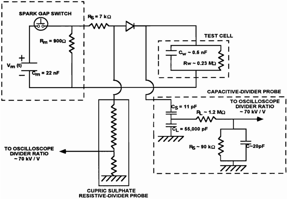
Figure 3.3 An electrical sketch of the electrical-impulse, water-breakdown experiment.
