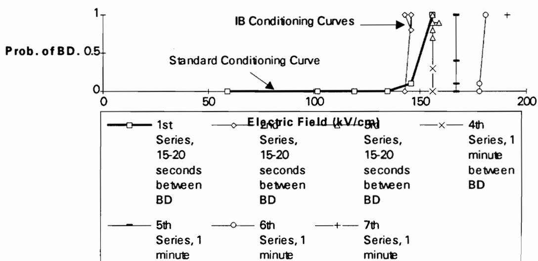
Figure 4.7 Test run of 9/3/93. Note the heavy line depicting the standard conditioning curve. Also note that the IB-conditioning curves are of two types:
