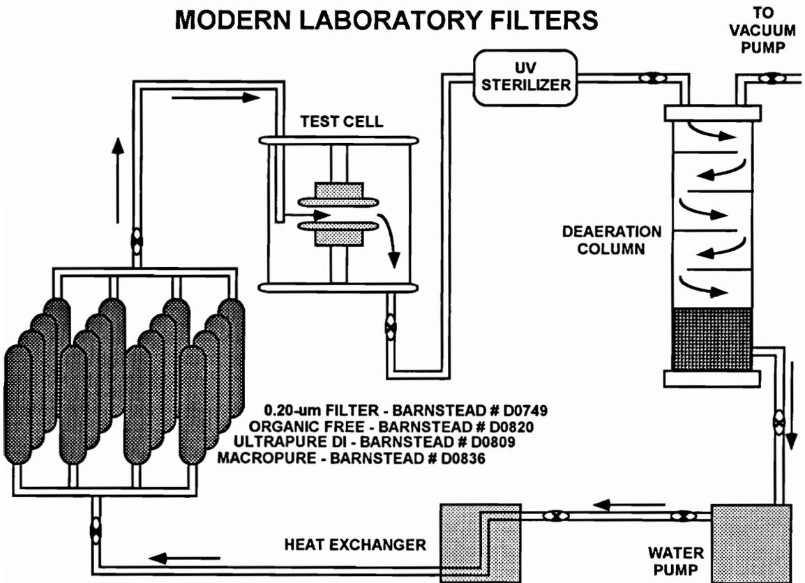
Figure 3.2 The sketch of the more modern water-treatment apparatus for the electrical-impulse, water-breakdown experiment.
