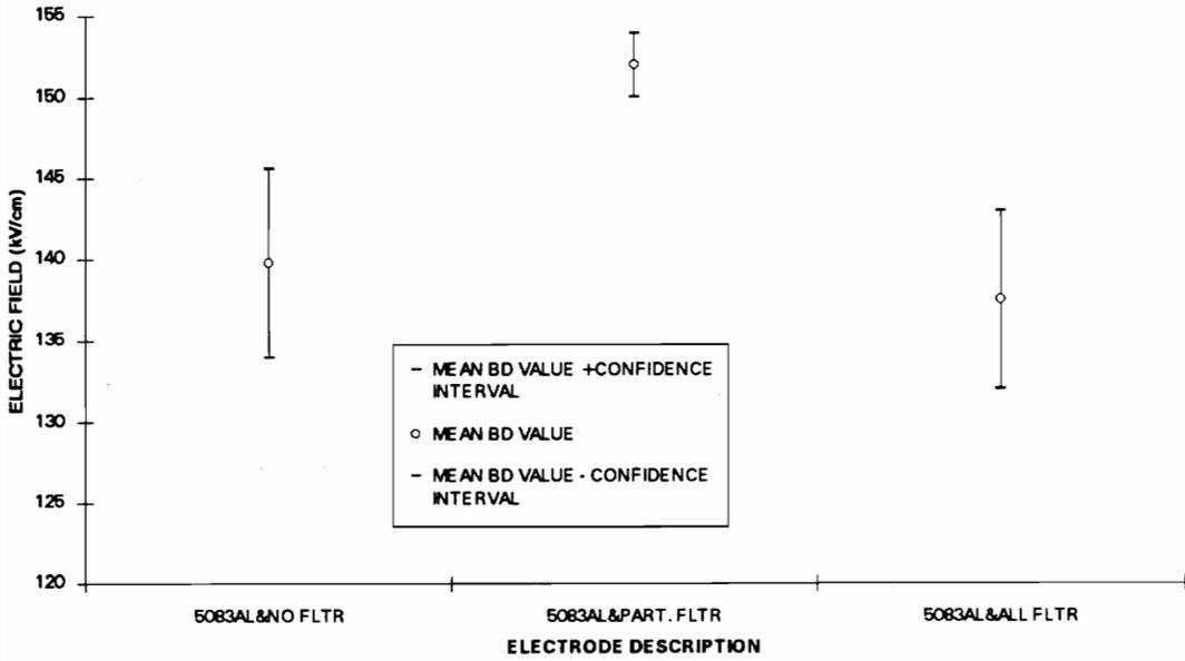
Figure 5.6 Plot of the mean breakdown field plus or minus the 95% confidence interval for aluminum 5083-alloy electrodes, with filters.
