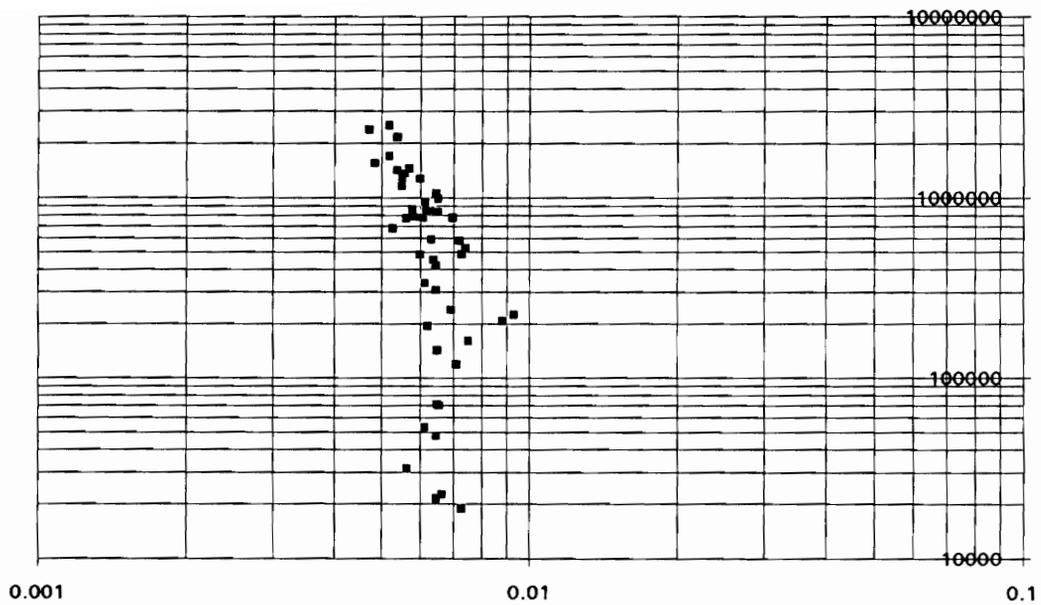
Figure 5.22. Plot of the log of "true" energy versus  $1/E$  for tungsten electrodes.
