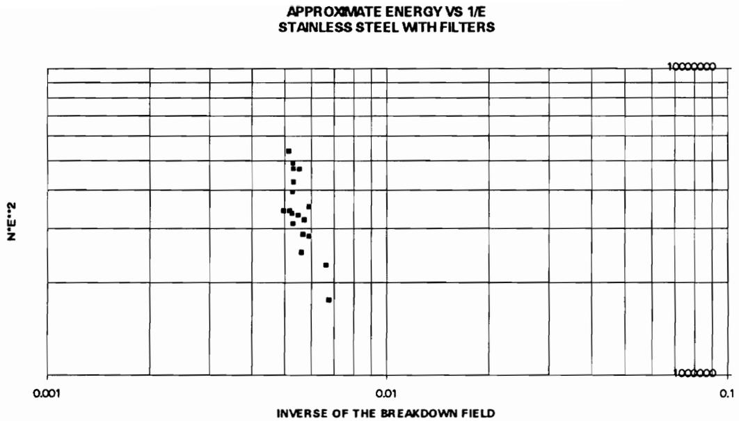
Figure 5.20. Same plot, but for filters with stainless steel electrodes. There are fewer data points here, which may help explain the poor agreement of the exponent with the expected value of -5. The exponent measured on a blown-up graph was -3.17.
