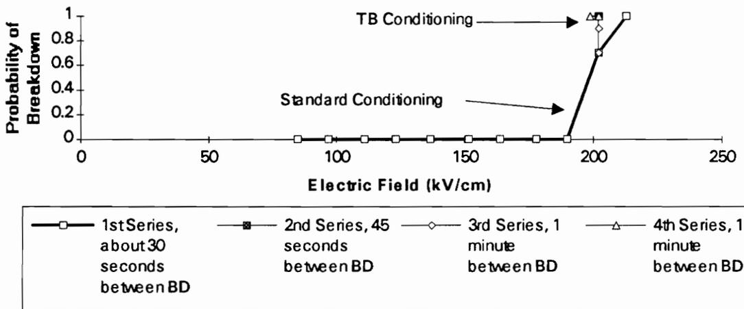
Figure 4.11 Test run of 9/24/93. Note the heavy line depicting the standard conditioning curve. We want to determine if there is any difference in TB conditioning when 45 seconds elapsed between breakdowns or a longer time (i.e., 1 minute) is allowed between breakdowns. Some of the lines are not vertical because the applied voltage strays slightly about the set point due to variations in the charging circuitry.
