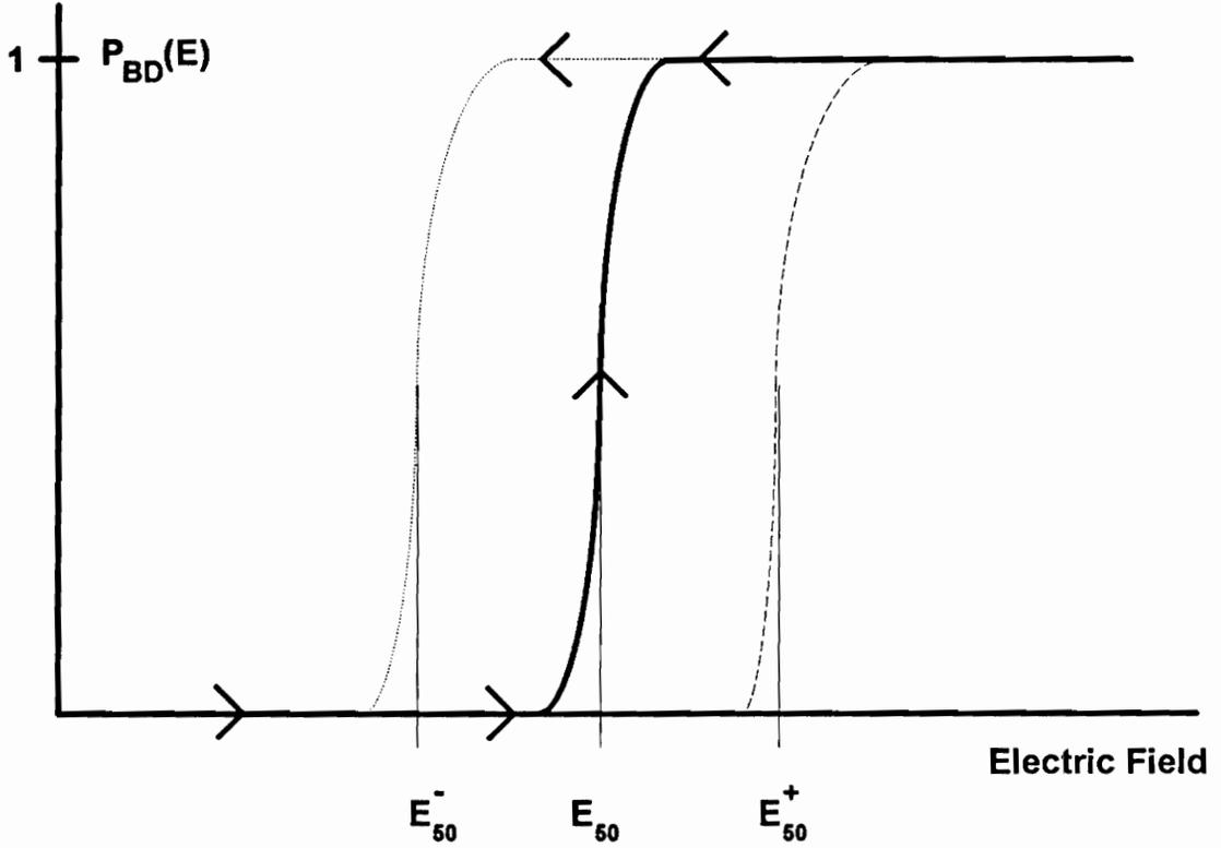
Figure 6.1 Conceptual diagram of the hysteresis region for the breakdown probability as a function of electric field.
