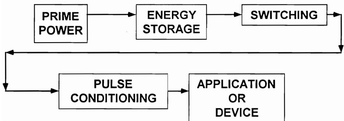
Figure 1.2: Pulsed-power circuit.
