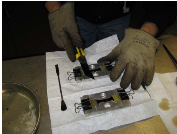
Figure 3-8 Making asphalt binder specimen
