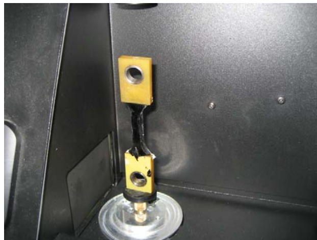
Figure 3-13 Whole mastic specimen to be scanned
