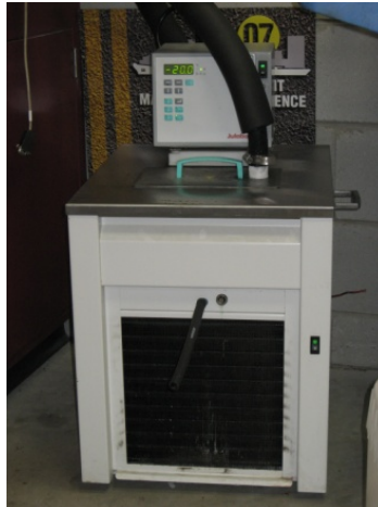
Figure 3-3 Chiller system of direct tension tester
