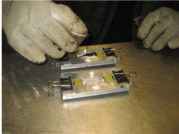
Figure 3-8 Making asphalt binder specimen
