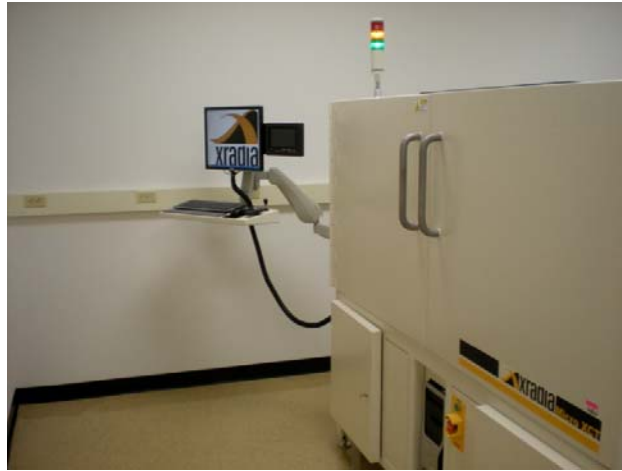
Figure 7-10 Xraida MicroCT-200 system
