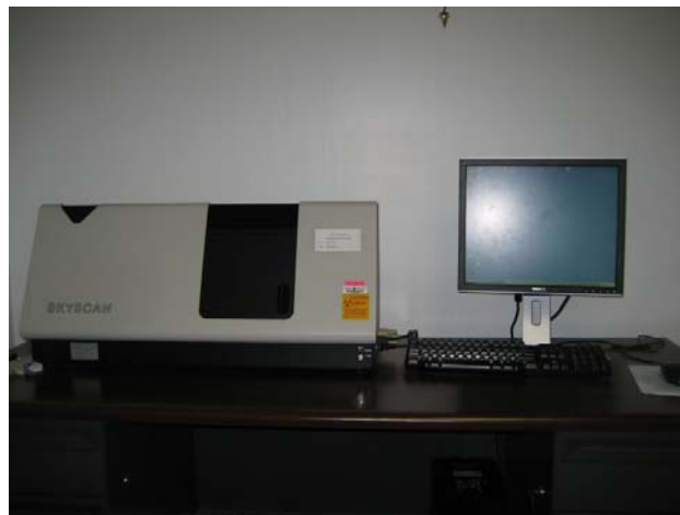
Figure 3-12 Skyscan Micro-CT 1174 system
