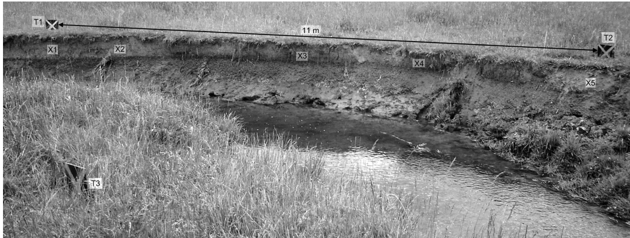
Figure 2.1. Image of streambank showing locations of scan targets (T's) and cross sections (X's).
