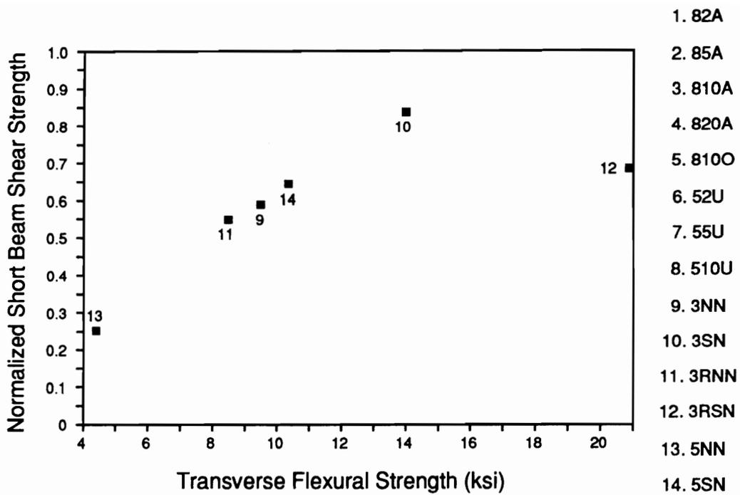
Figure 6. Normalized Short Beam Shear Strength versus Transverse Flexural Strength of the Northrop Materials [39].
