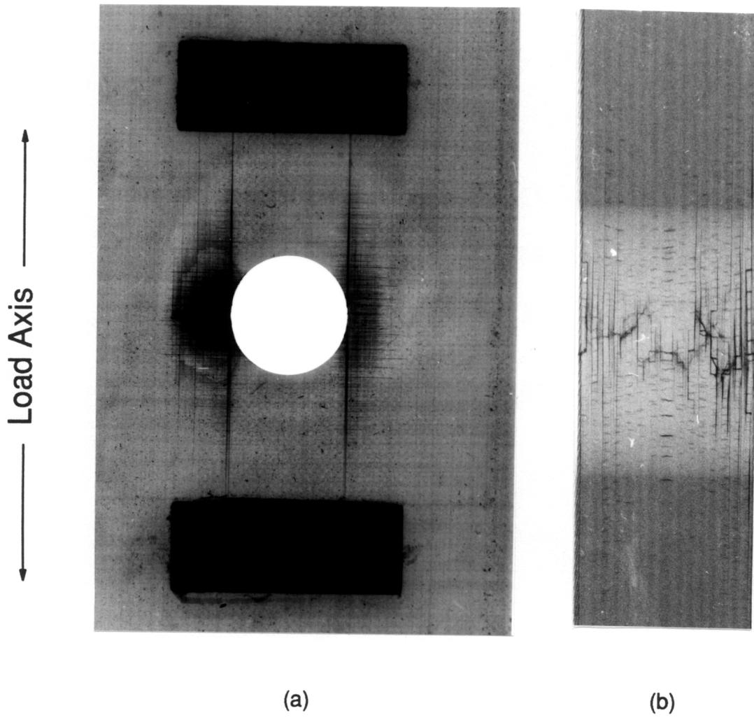
Figure 38. X-ray Radiograph of an 820A Specimen after 19,000 Cycles; a.) Front View, b.) Edge View.
