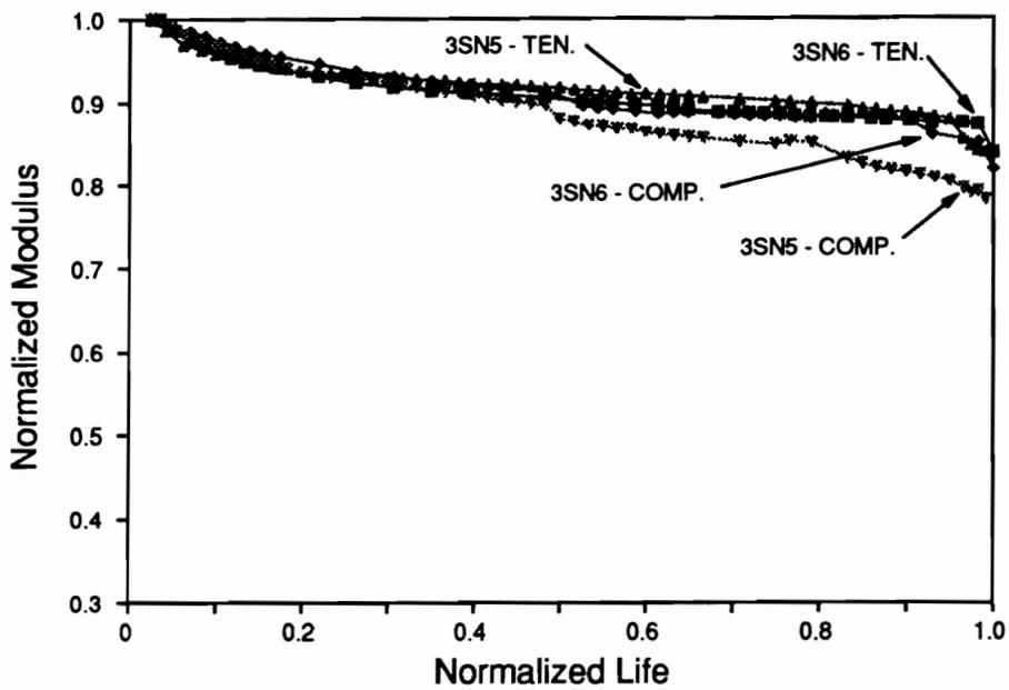
Figure 58. Plot of Normalized Modulus versus Normalized Life for Two 3SN Specimens; Max. Stress = 75% UCS; R = -1 at 10 Hz.
