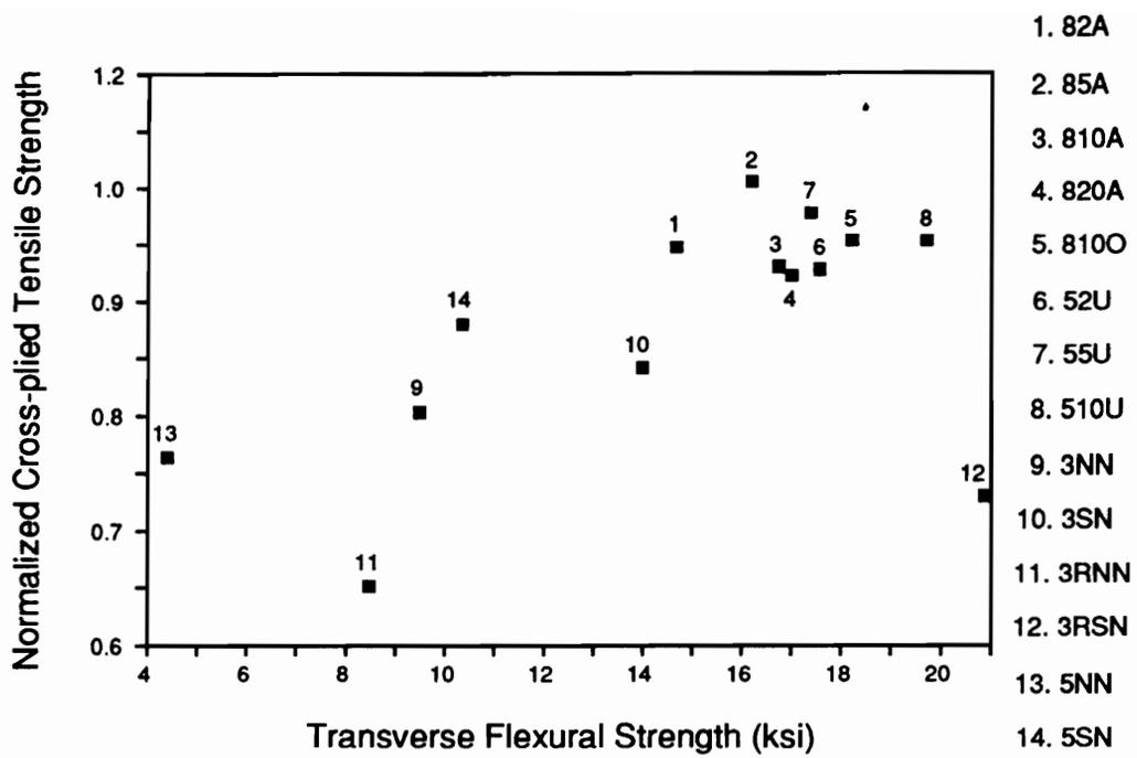
Figure 80. Normalized Cross-plyed Tensile Strength versus Transverse Flexural Strength of the McAir and Northrop Materials [37,40].
