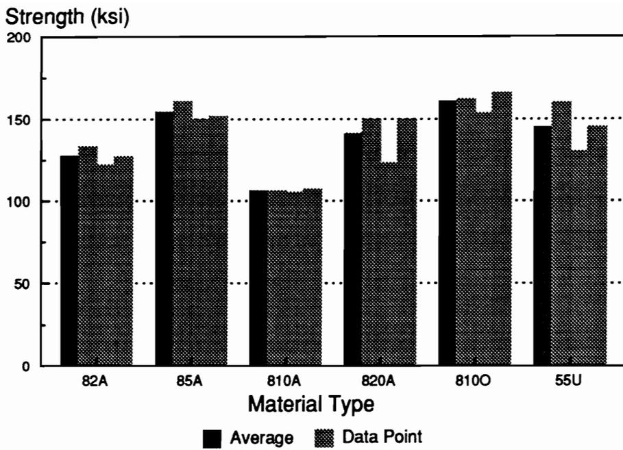
Figure 30. Average Strength and Strength of Individual Unidirectional Compressive Specimens from the McAir Materials.
