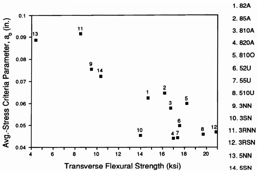
Figure 82. The Calculated Average-Stress Criteria Parameter versus the Transverse Flexural Strength of the McAir & Northrop Materials.
