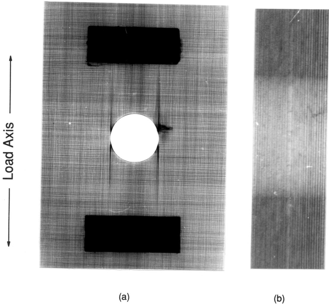
Figure 50. X-ray Radiograph of a 3RNN Specimen after 2200 Cycles; a.) Front View, b.) Edge View.
