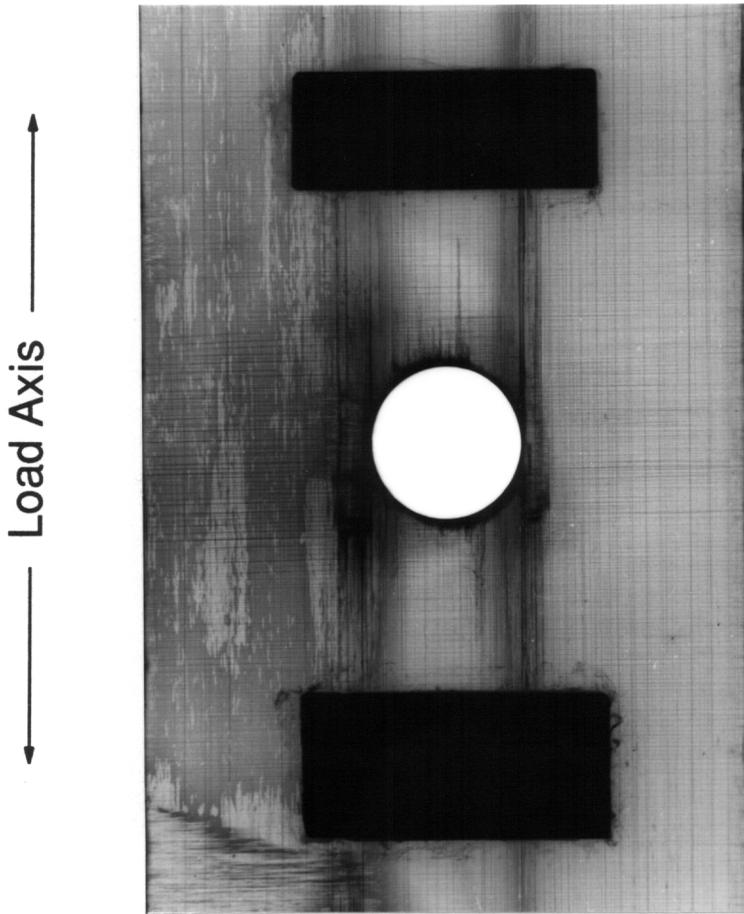
Figure 52. X-ray Radiograph of a 5NN Specimen after 112,000 Cycles.
