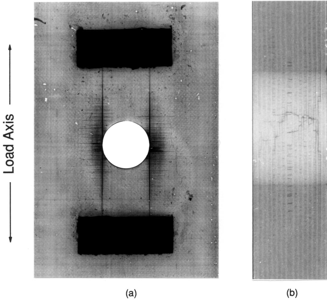
Figure 37. X-ray Radiograph of an 820A Specimen after 30,000 Cycles; a.) Front View, b.) Edge View.
