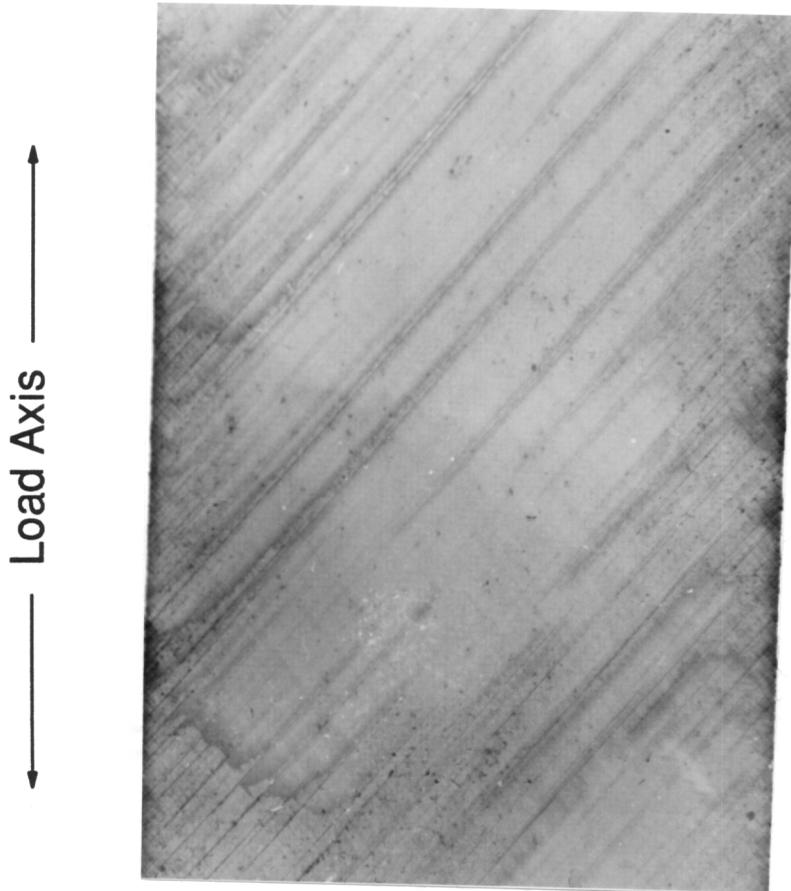
Figure 76. X-ray Radiograph of a  $\pm 45^\circ$  510U Specimen after 1 Million Cycles; Max. Stress = 24 ksi; R = -1 at 10 Hz.
