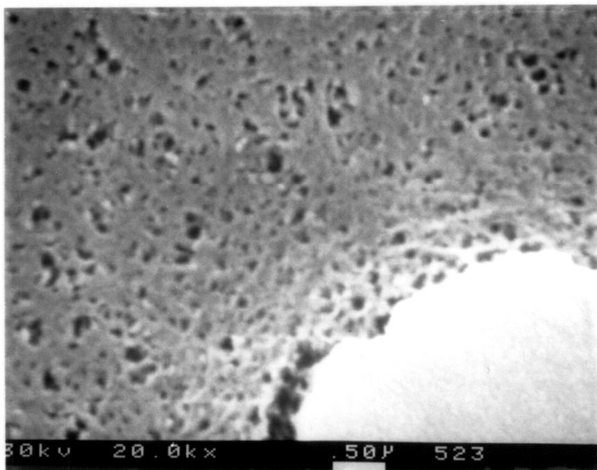
Figure 67. SEM Micrograph of an Etched 820A Specimen (x 20,000).
