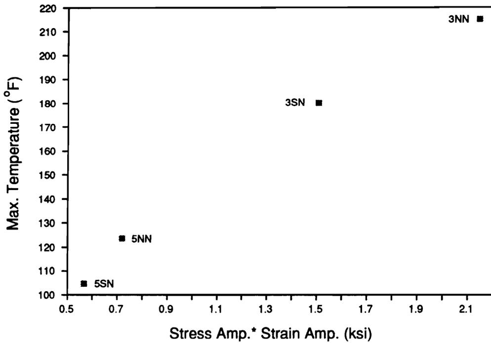
Figure 65. Plot of Maximum Specimen Temperature versus Specific Energy Term for Northrop Materials; Max. Stress = 75% UCS; R = -1 at 10 Hz.
