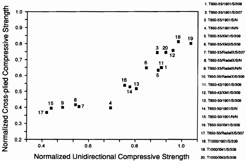
Figure 85. Normalized Cross-plyed Compressive Strength vs. Normalized Unidirectional Compressive Strength; Northrop Materials [39,40].
