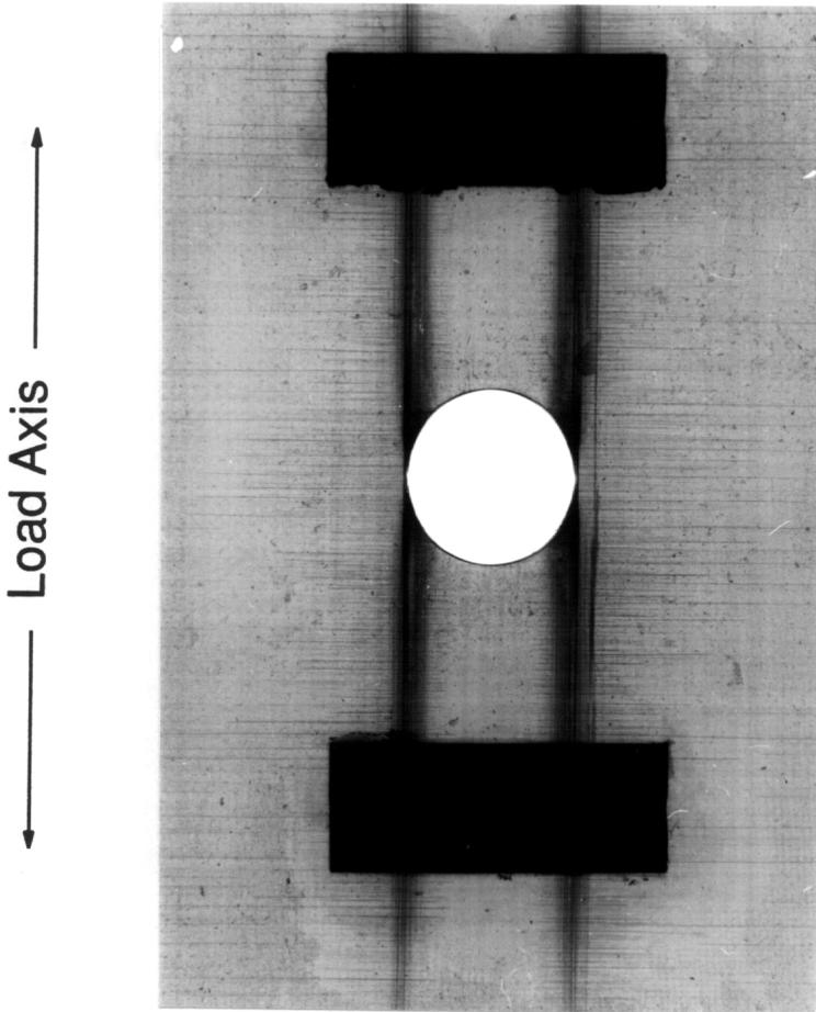
Figure 42. X-ray Radiograph of a 52U Specimen after 70,000 Cycles.
