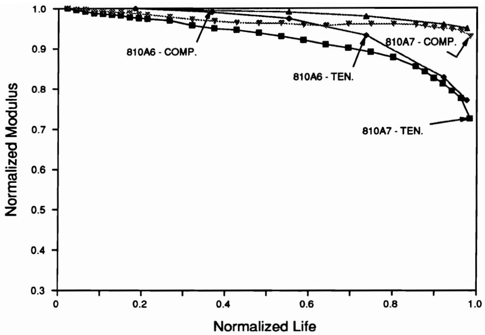
Figure 55. Plot of Normalized Modulus versus Normalized Life for Two 810A Specimens; Max. Stress = 75% UCS; R=-1 at 10 Hz.
