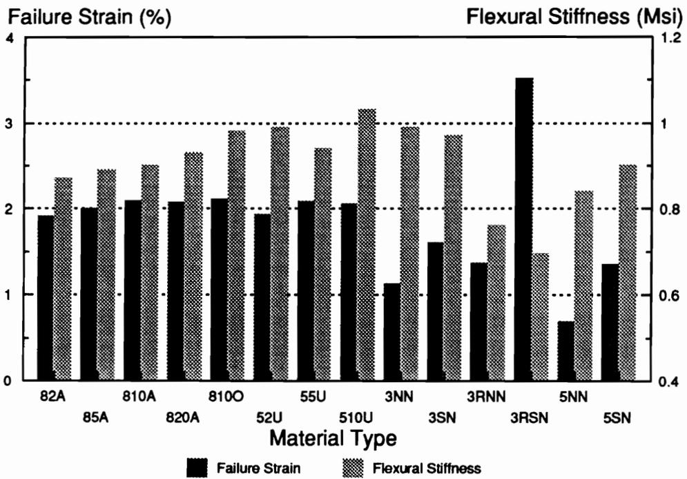
Figure 4. Average Transverse Flexural Failure Strain and Stiffness of the McAir and Northrop Materials.
