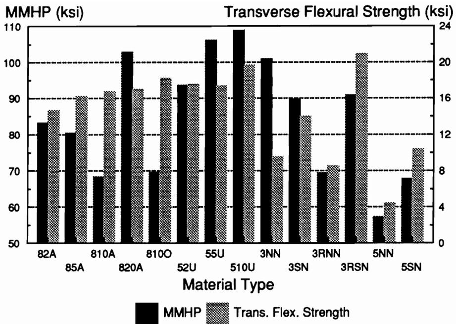
Figure 10. Maximum Mean Hardness Pressure and Transverse Flexural Strength of the McAir and Northrop Materials.
