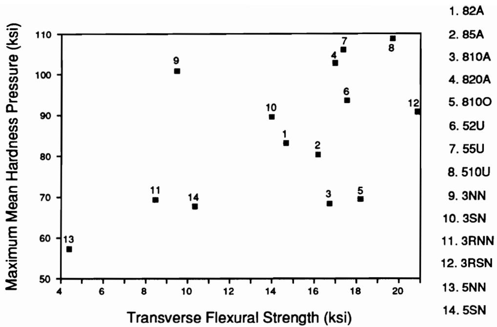
Figure 11. Maximum Mean Hardness Pressure versus Transverse Flexural Strength of the McAir and Northrop Materials.
