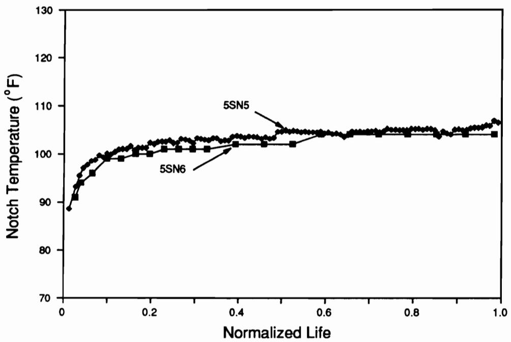
Figure 63. Plot of Notch Temperature versus Normalized Life for Two 5SN Specimens; Max. Stress = 75% UCS; R = -1 at 10 Hz.
