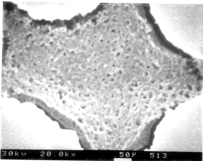
Figure 68. SEM Micrograph of an Etched 8100 Specimen (x 20,000).
