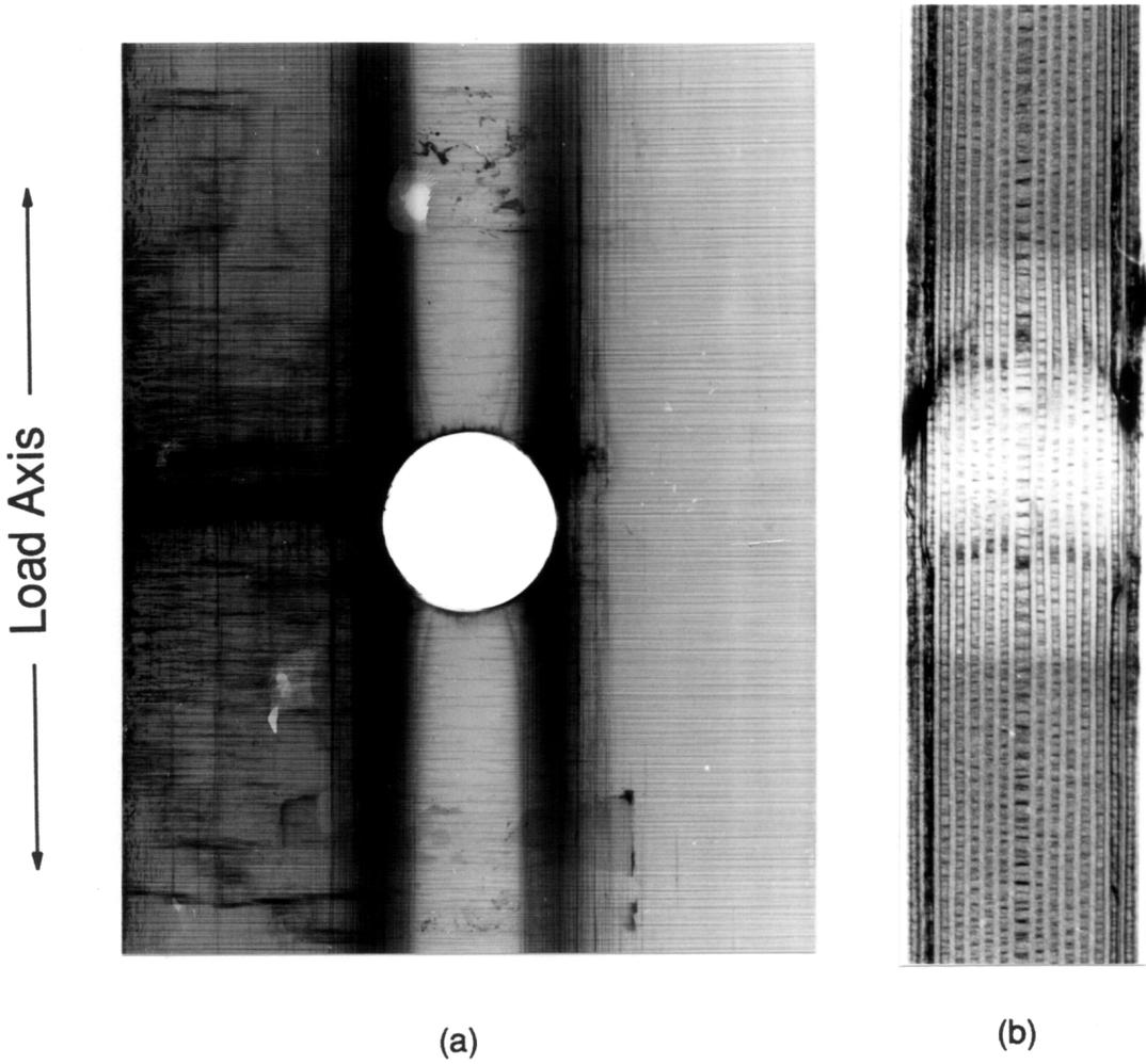
Figure 49. X-ray Radiograph of a 3NN Specimen after 12,300 Cycles; a.) Front View, b.) Edge View.
