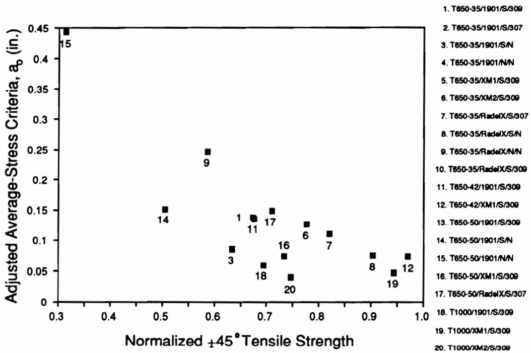
Figure 88. Adjusted Average-Stress Criteria Parameter versus Normalized  $\pm 45^\circ$  Tensile Strength; Northrop Materials [39].
