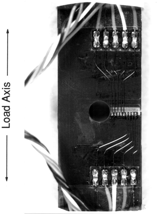
Figure 1. Photograph of a Strip Gage Applied to an 810A Specimen.
