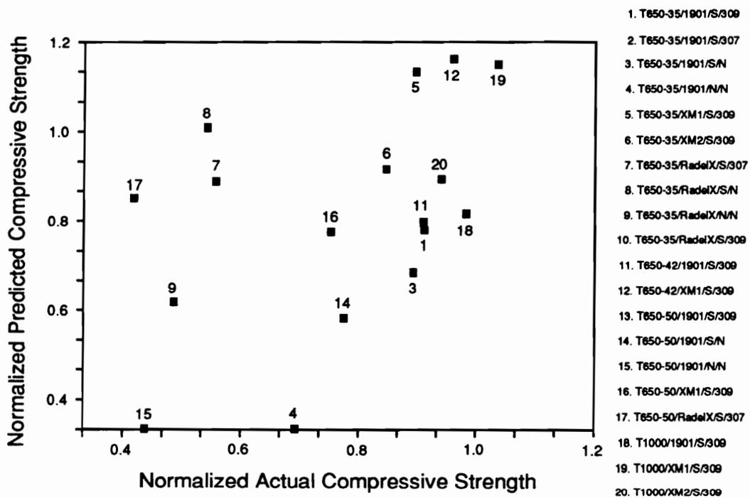
Figure 83. Normalized Unidirectional Compressive Strength; Predicted Values versus Actual Values (Shear Failure Scenario) [39].
