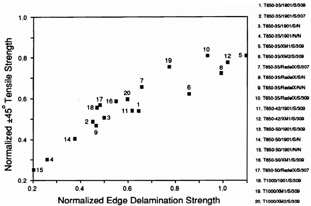
Figure 26. Normalized  $\pm 45^\circ$  Tensile Strength versus Normalized Edge Delamination Strength of the Northrop Materials [39].
