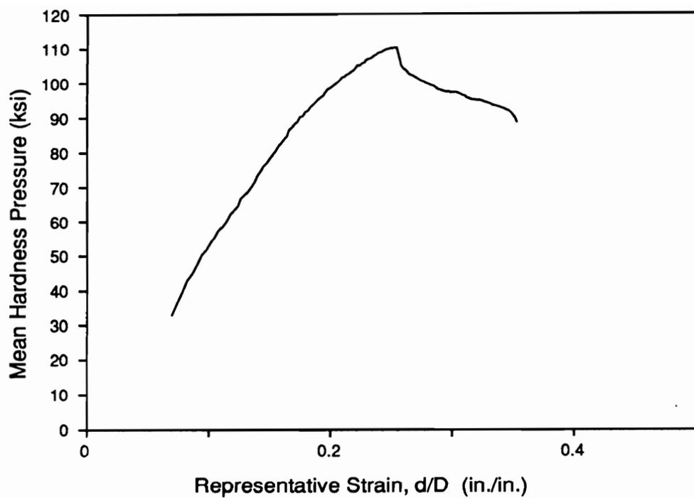
**Figure 8. Mean Hardness Pressure versus Representative Strain for a 55U Specimen using the CBIT.**
