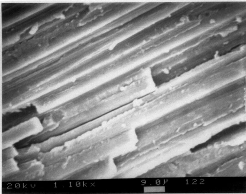
Figure 70. SEM Micrograph of a Failed Notched Cross-plyed 8100 Tensile Specimen (x 1100).
