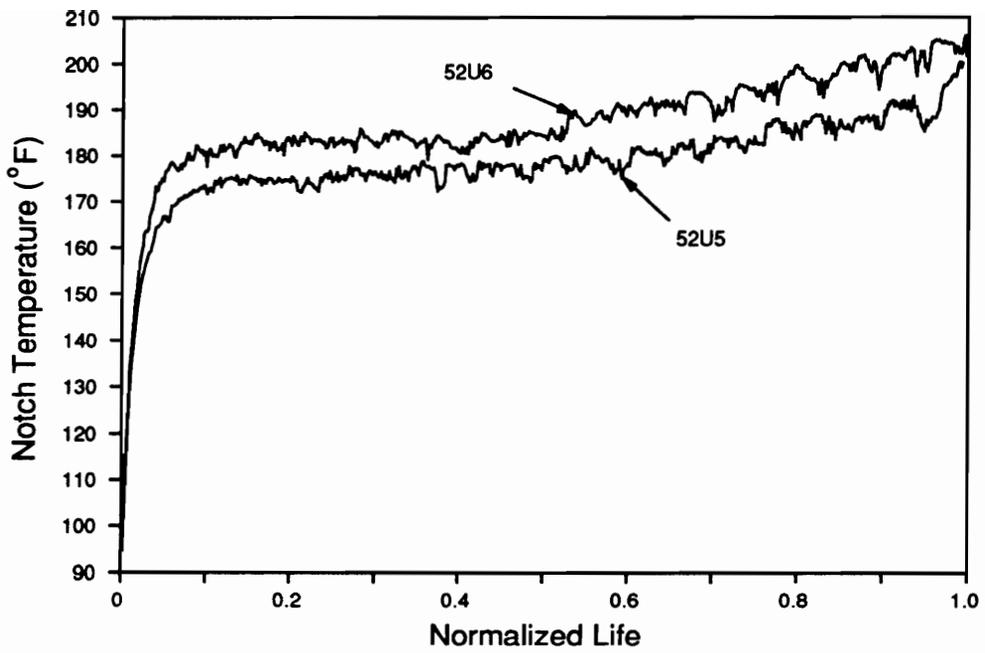
Figure 62. Plot of Notch Temperature versus Normalized Life for Two 52U Specimens; Max. Stress = 75% UCS; R = -1 at 10 Hz.
