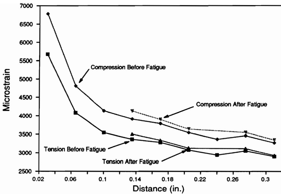
Figure 74. Longitudinal Strain Measurements as a Function of Distance from the Hole; 8100 Before and After Fatigue.
