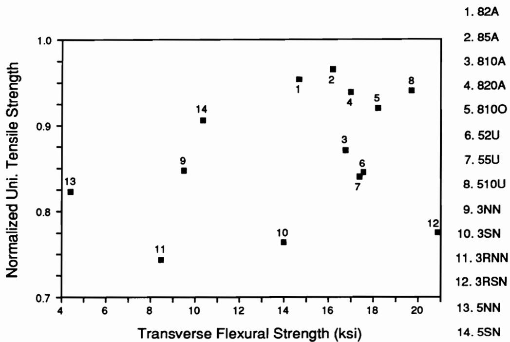
Figure 78. Normalized Unidirectional Tensile Strength versus Transverse Flexural Strength of the McAir and Northrop Materials [37,39].
