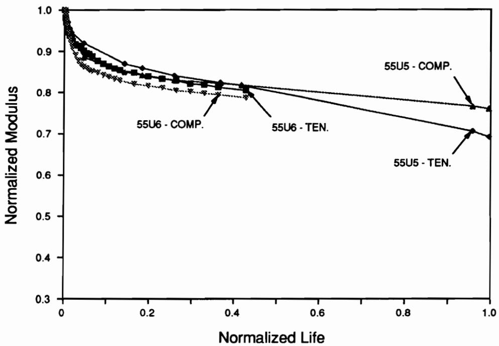
Figure 56. Plot of Normalized Modulus versus Normalized Life for Two 55U Specimens; Max. Stress = 75% UCS; R = -1 at 10 Hz.
