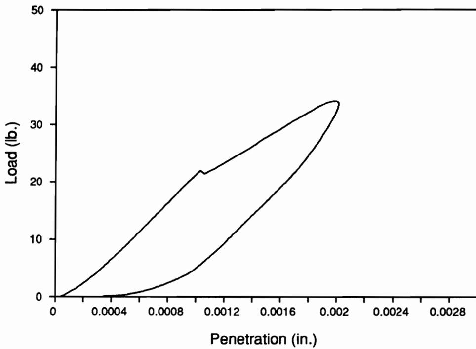
**Figure 7. Applied Load versus Indentation Depth on a 55U Specimen using the CBIT.**
