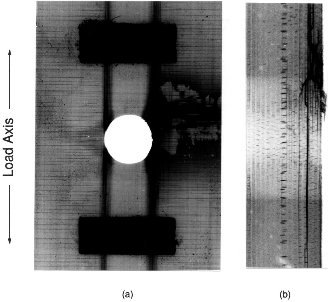
Figure 45. X-ray Radiograph of a 510U Specimen after 183,400 Cycles; a.) Front View, b.) Edge View.
