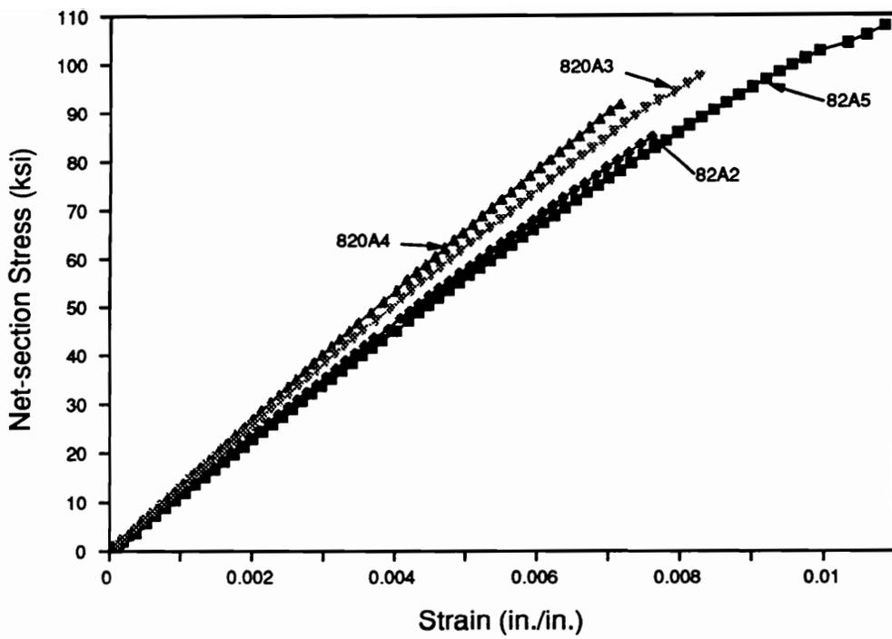
Figure 19. Net-section Tensile Stress versus Measured Strain for Two 82A Specimens and Two 820A Specimens.
