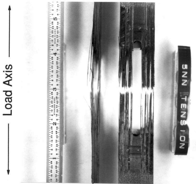
Figure 16. Photograph of Failed 5NN Tensile Specimens.
