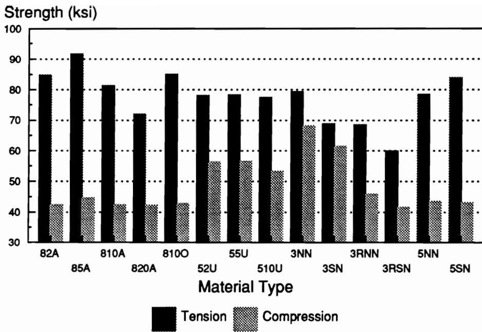
Figure 13. Average Gross-section Tensile and Compressive Strengths of the Notched Cross-plyed McAir and Northrop Materials.
