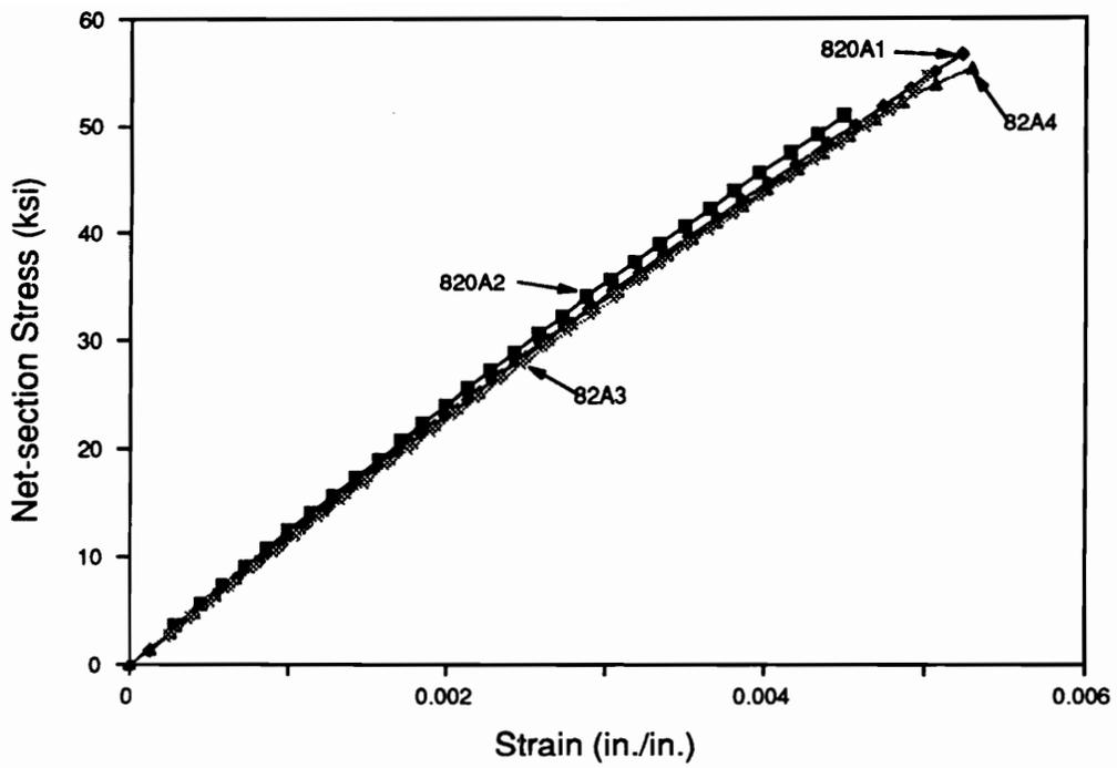
Figure 21. Net-Section Compressive Stress vs. Measured Strain for Two 82A Specimens and Two 820A Specimens.
