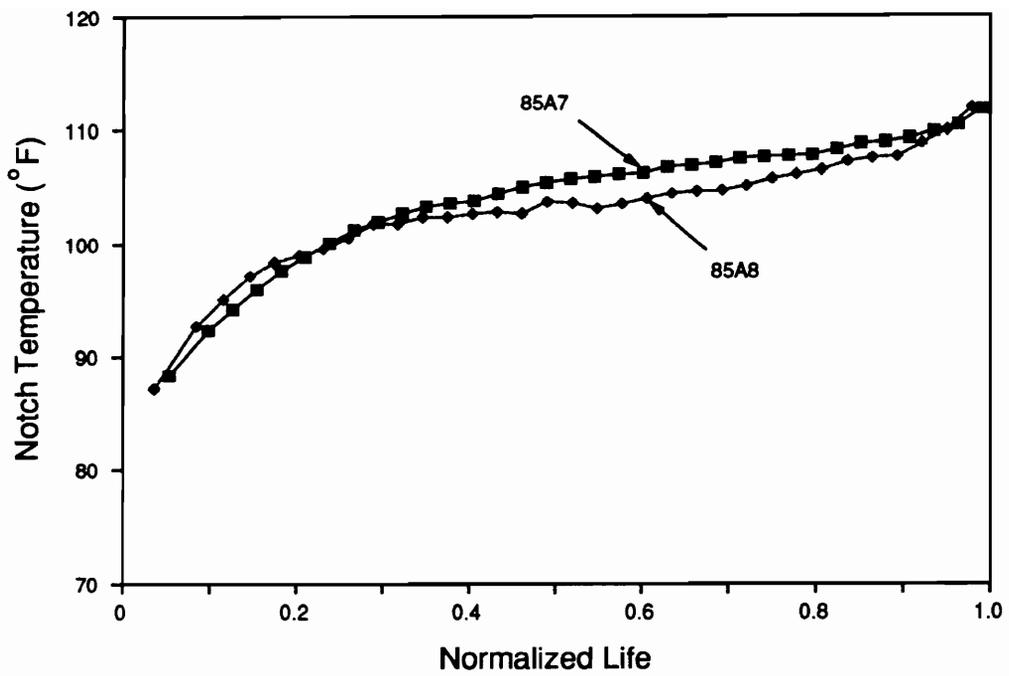
Figure 60. Plot of Notch Temperature versus Normalized Life for Two 85A Specimens; Max. Stress = 75% UCS; R = -1 at 10 Hz.
