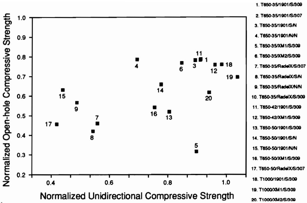
Figure 86. Normalized Open-hole Compressive Strength versus Normalized Unidirectional Compressive Strength; Northrop Materials [39].
