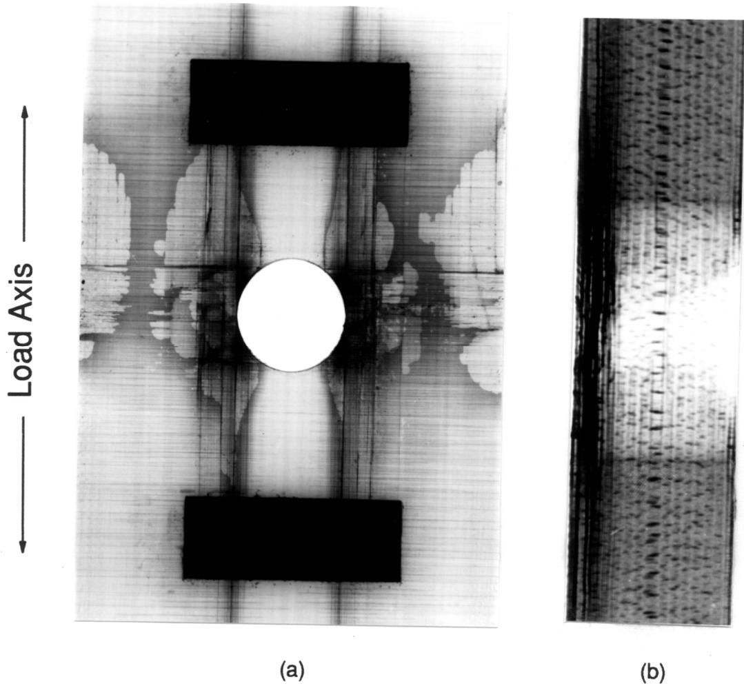
Figure 40. X-ray Radiograph of an 8100 Specimen after 882,500 Cycles; a.) Front View, b.) Edge View.
