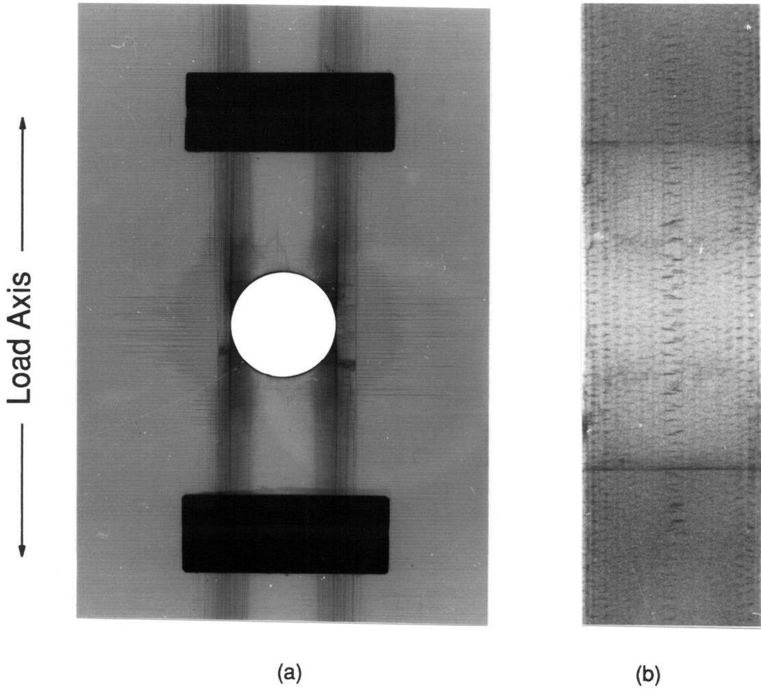
Figure 47. X-ray Radiograph of a 3NN Specimen after 7000 Cycles; a.) Front View, b.) Edge View.
