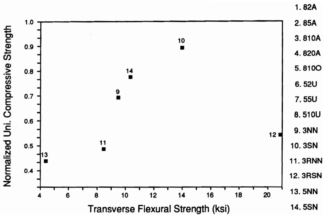
Figure 32. Normalized Unidirectional Compressive Data versus Transverse Flexural Strength of the Northrop Materials [39].
