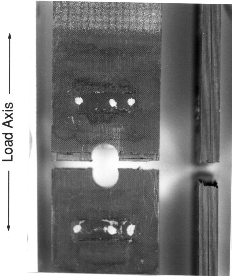
Figure 15. Photograph of Failed 820A Tensile Specimens.
