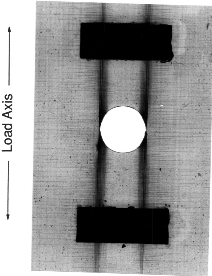
Figure 44. X-ray Radiograph of a 510U Specimen after 136,100 Cycles.
