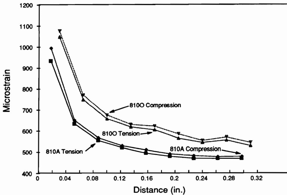
Figure 71. Longitudinal Strain Measurements as a Function of Distance from the Hole; 810A and 810O under 1000 & -1000 lb.
