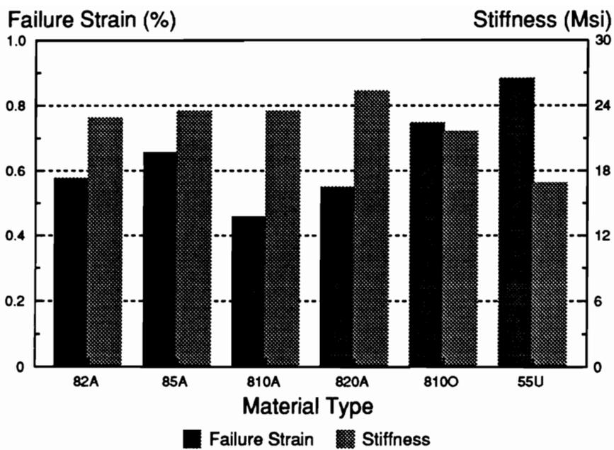
Figure 31. Average Failure Strain and Average Stiffness of the Unidirectional Compressive Specimens from the McAir Materials.
