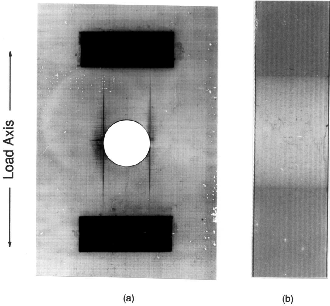
Figure 35. X-ray Radiograph of an 85A Specimen after 2870 Cycles; a.) Front View, b.) Edge View.
