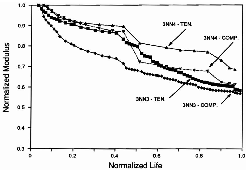
Figure 57. Plot of Normalized Modulus versus Normalized Life for Two 3NN Specimens; Max. Stress = 75% UCS; R = -1 at 10 Hz.
