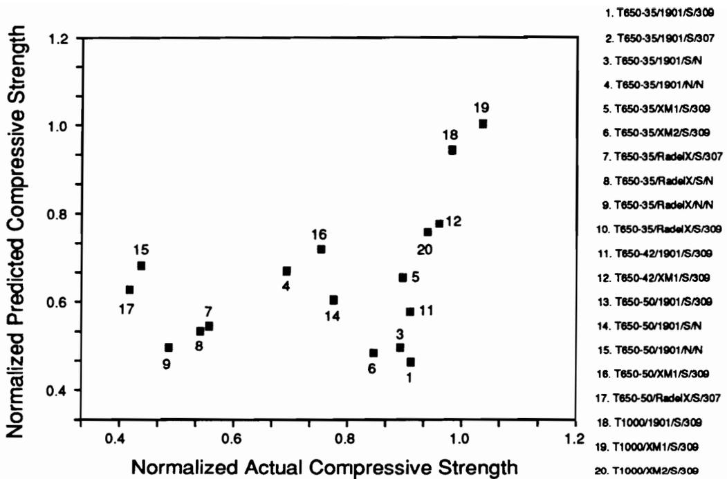
Figure 84. Normalized Unidirectional Compressive Strength; Predicted Values versus Actual Values (Bending Failure Scenario) [39].
