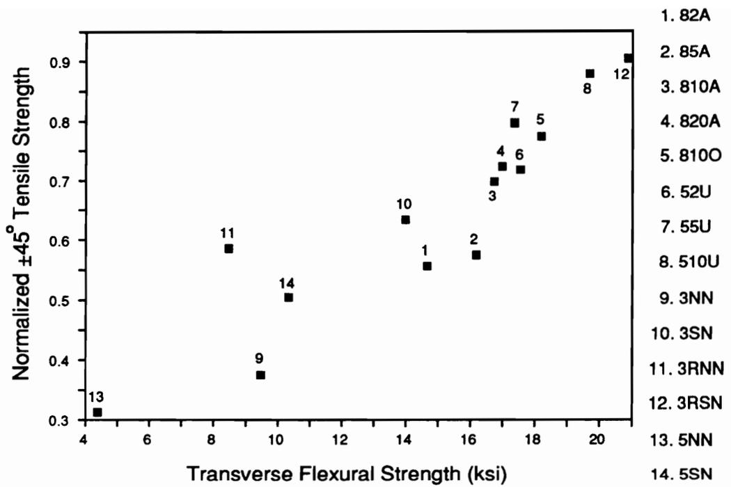
Figure 23. Normalized  $\pm 45^\circ$  Tensile Strength versus Transverse Flexural Strength of the McAir and Northrop Materials [37,39].
