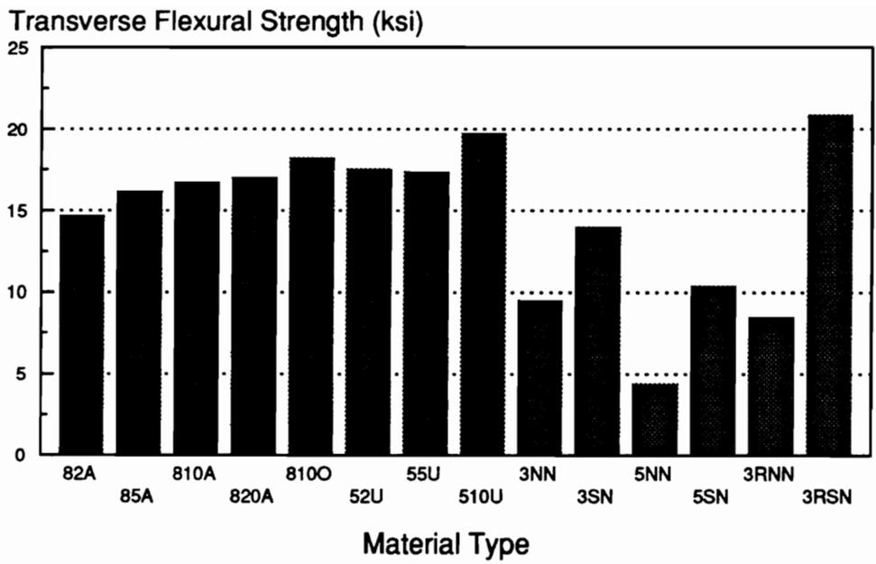
Figure 3. Average Transverse Flexural Strength of the McAir and Northrop Materials.
