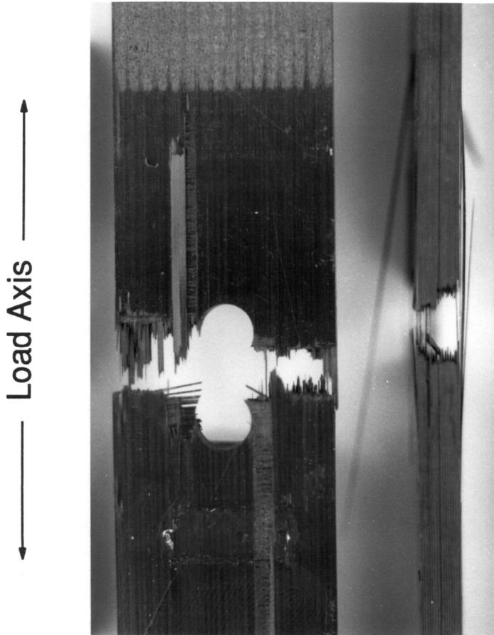
Figure 14. Photograph of Failed 82A Tensile Specimens.
