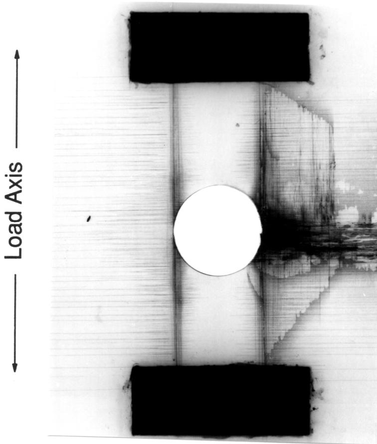
Figure 53. X-ray Radiograph of a 5SN Specimen after 15,200 Cycles.
