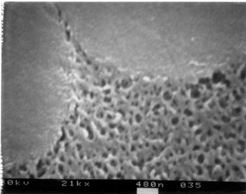
Figure 66. SEM Micrograph of an Etched 810A Specimen (x 21,000).
