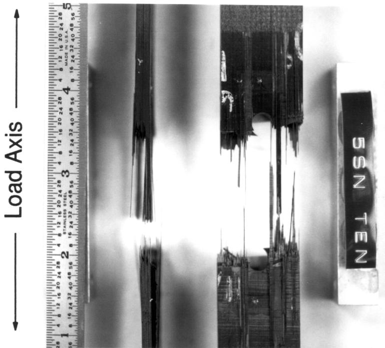
Figure 17. Photograph of Failed 5SN Tensile Specimens.
