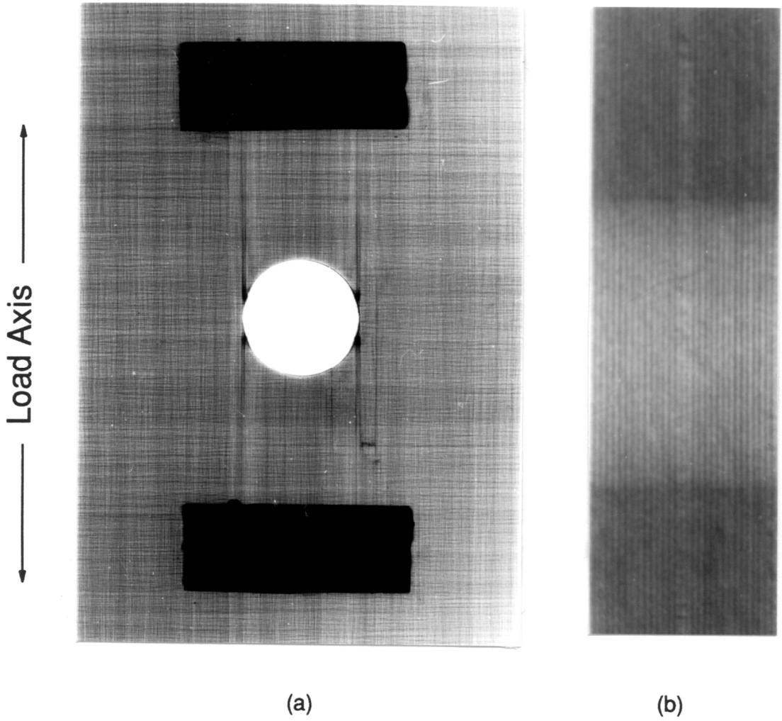
Figure 51. X-ray Radiograph of a 3RSN Specimen after 5500 Cycles; a.) Front View, b.) Edge View.
