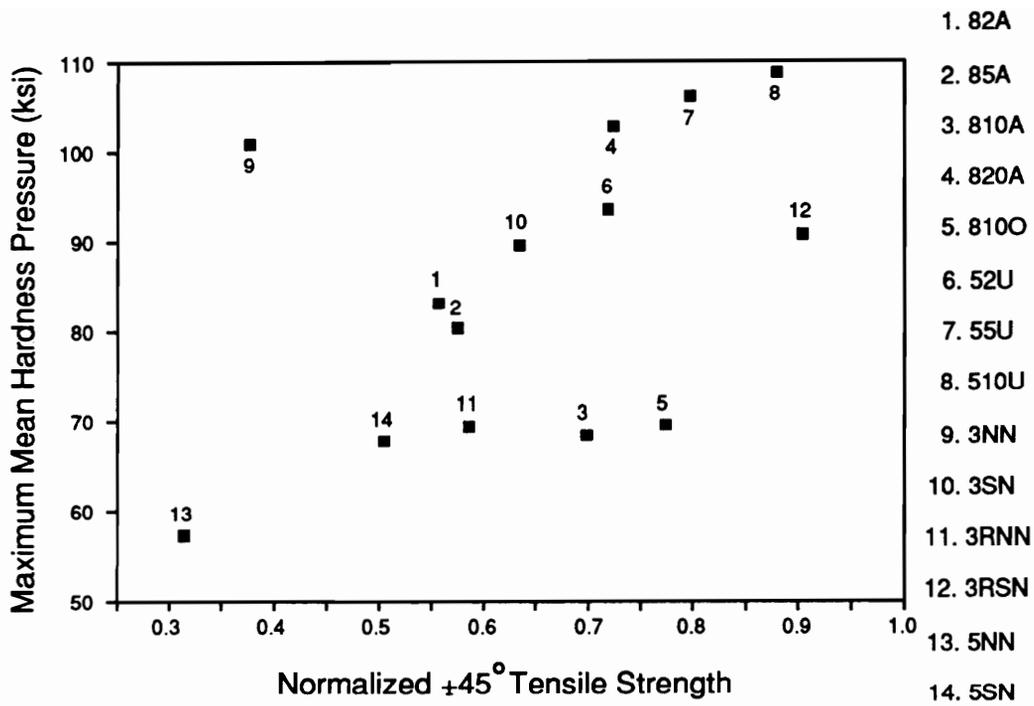
Figure 12. Maximum Mean Hardness Pressure versus Normalized  $\pm 45^\circ$  Tensile Strength of the McAir & Northrop Materials [37,39].
