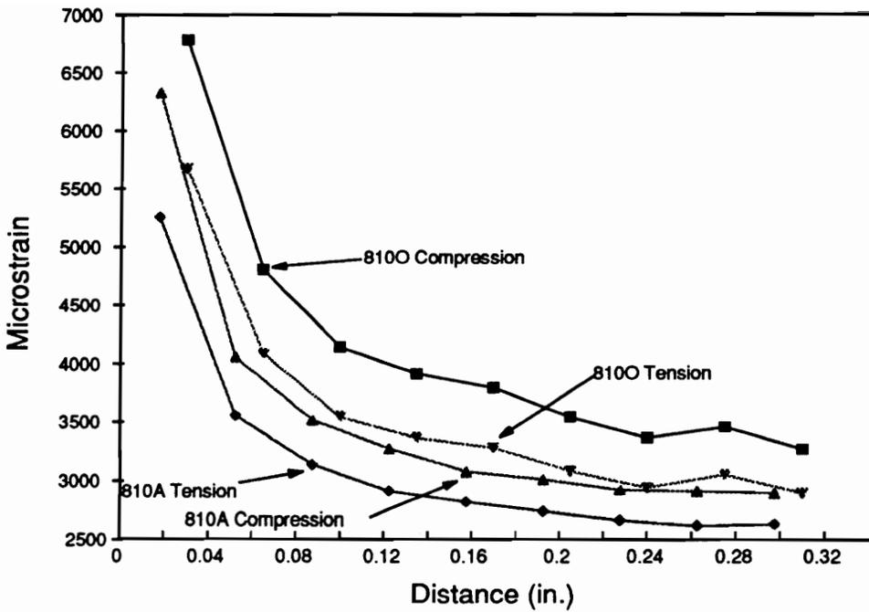
Figure 72. Longitudinal Strain Measurements as a Function of Distance from the Hole; 810A and 810O under 5752 & -5752 lb.
