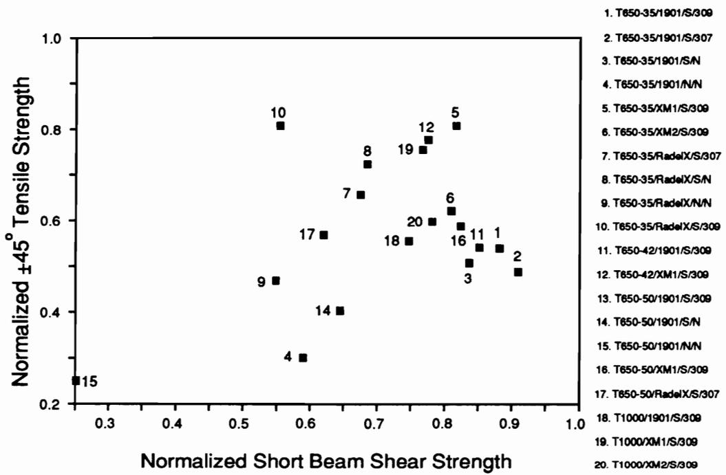
Figure 25. Normalized  $\pm 45^\circ$  Tensile Strength versus Normalized Short Beam Shear Strength of the Northrop Materials [39].
