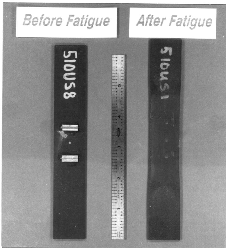
Figure 24. Photograph of Two  $\pm 45^\circ$  Specimens; a.) A Virgin Specimen, b.) A Fatigue Specimen that has Yielded.
