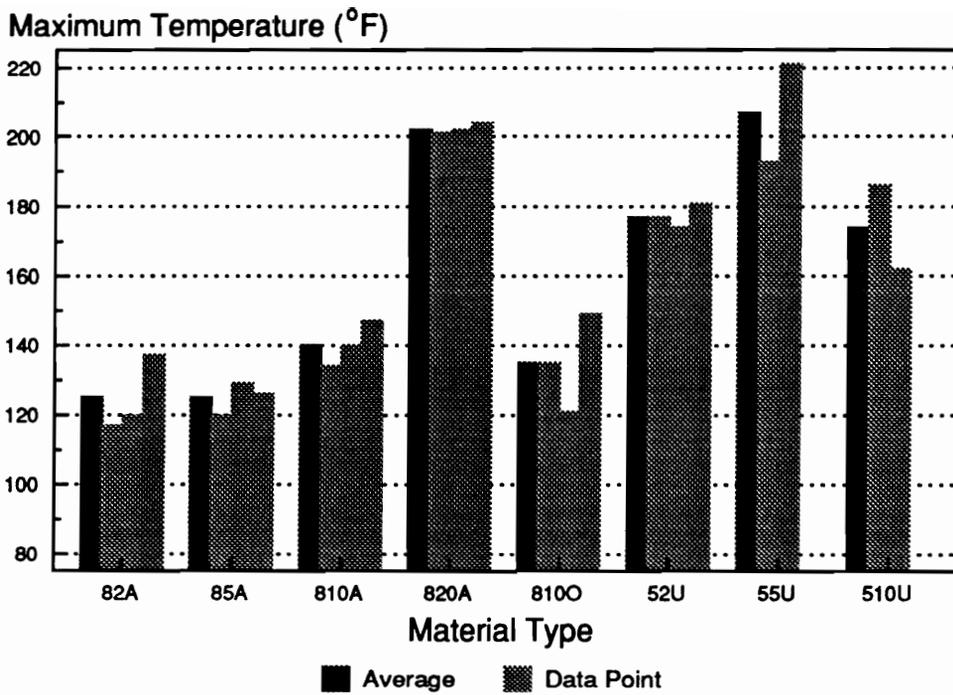
Figure 77. Temperature at Failure of the  $\pm 45^\circ$  McAir Specimens; Max. Stress = 24 ksi; R = 0.1 at 10Hz.
