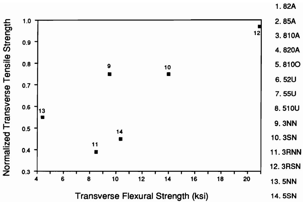
Figure 5. Normalized Transverse Tensile Strength versus Transverse Flexural Strength of the Northrop Materials [39].
