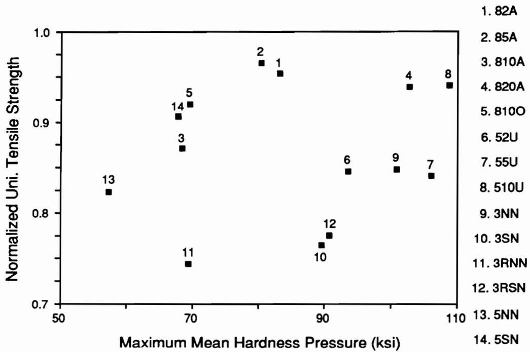
Figure 79. Normalized Unidirectional Tensile Strength versus Max. Mean Hardness Pressure of the McAir and Northrop Materials [37,39].
