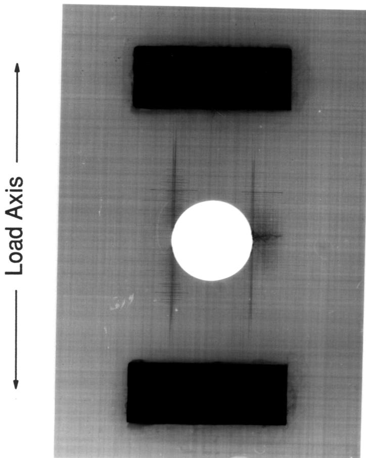
Figure 34. X-ray Radiograph of an 82A Specimen after 2550 Cycles.
