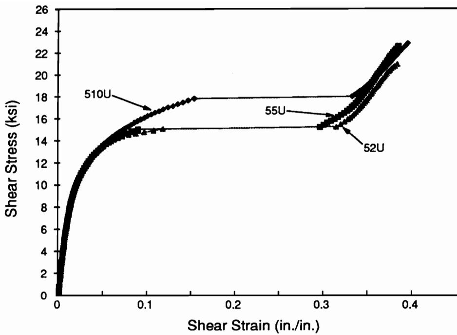
Figure 29. Shear Stress versus Shear Strain for Three Specimens in the 5U Series.
