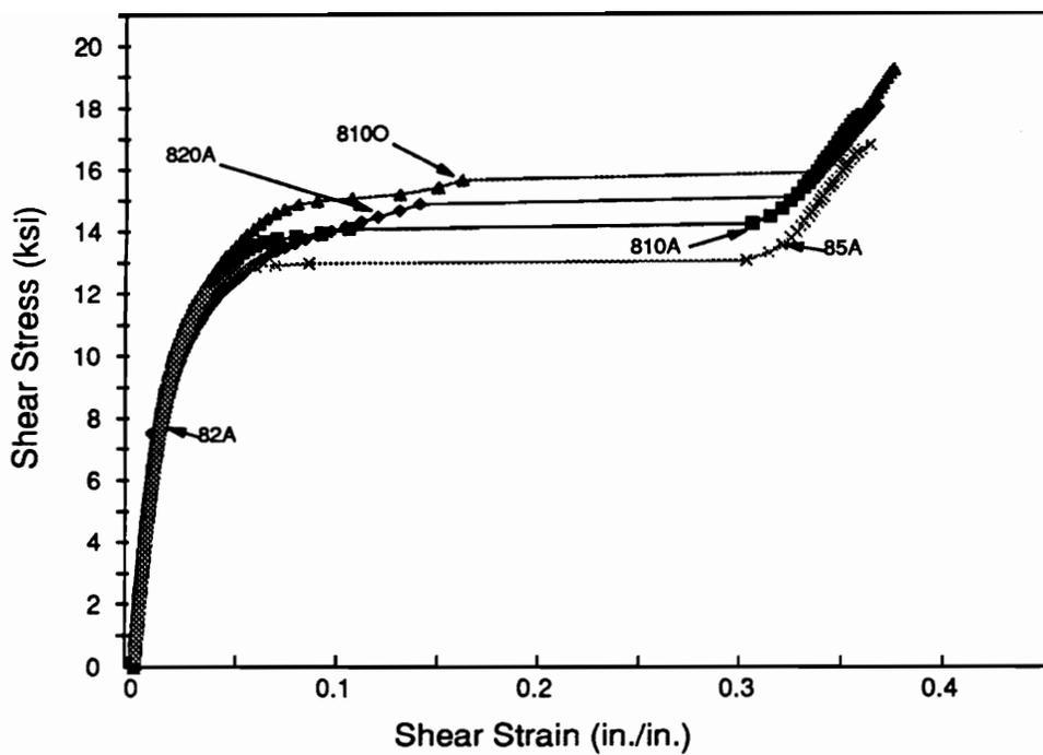
Figure 28. Shear Stress versus Shear Strain for Five Specimens in the 8A&O Series.
