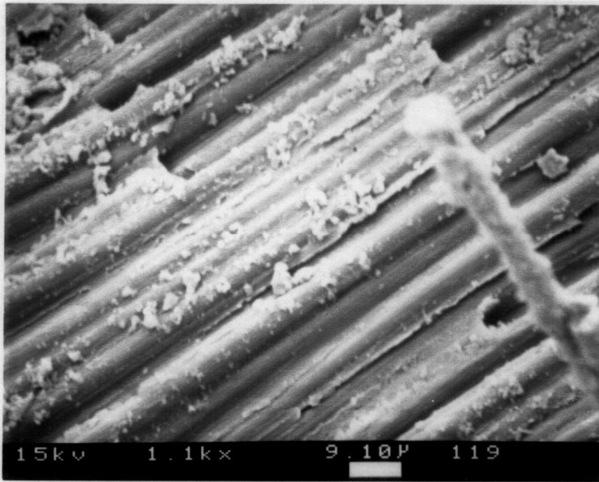
Figure 69. SEM Micrograph of a Failed Notched Cross-plyed 810A Tensile Specimen (x 1100).
