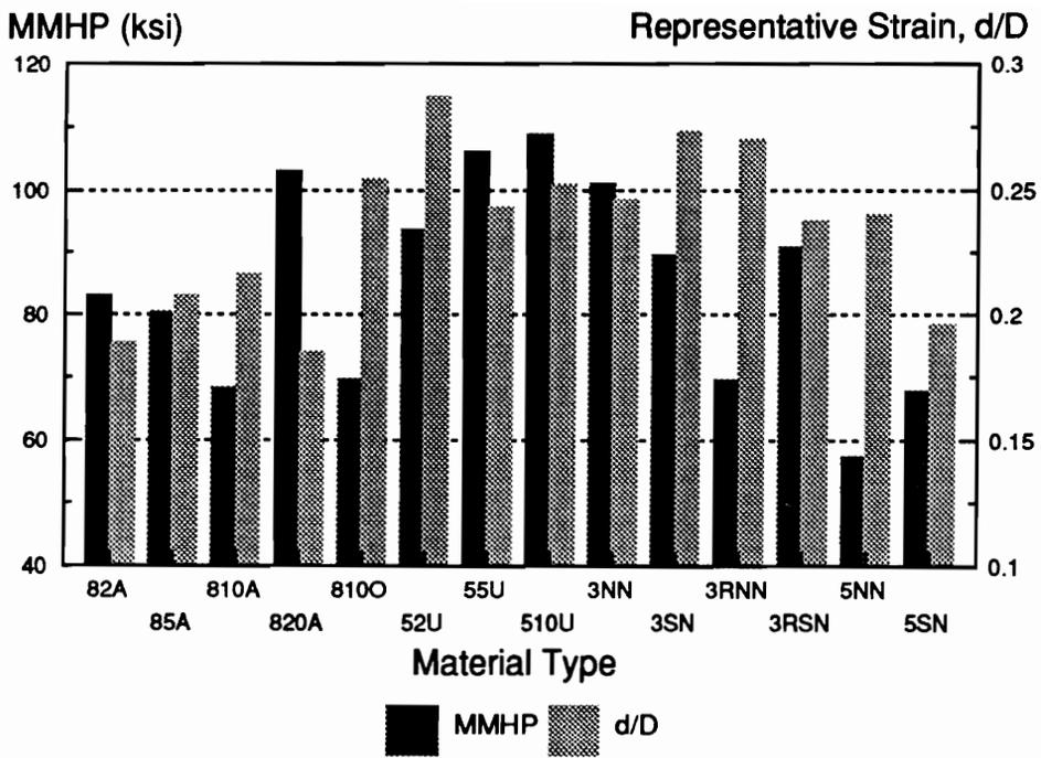
Figure 9. Average Maximum Mean Hardness Pressure and Representative Strain of the McAir and Northrop Materials.
