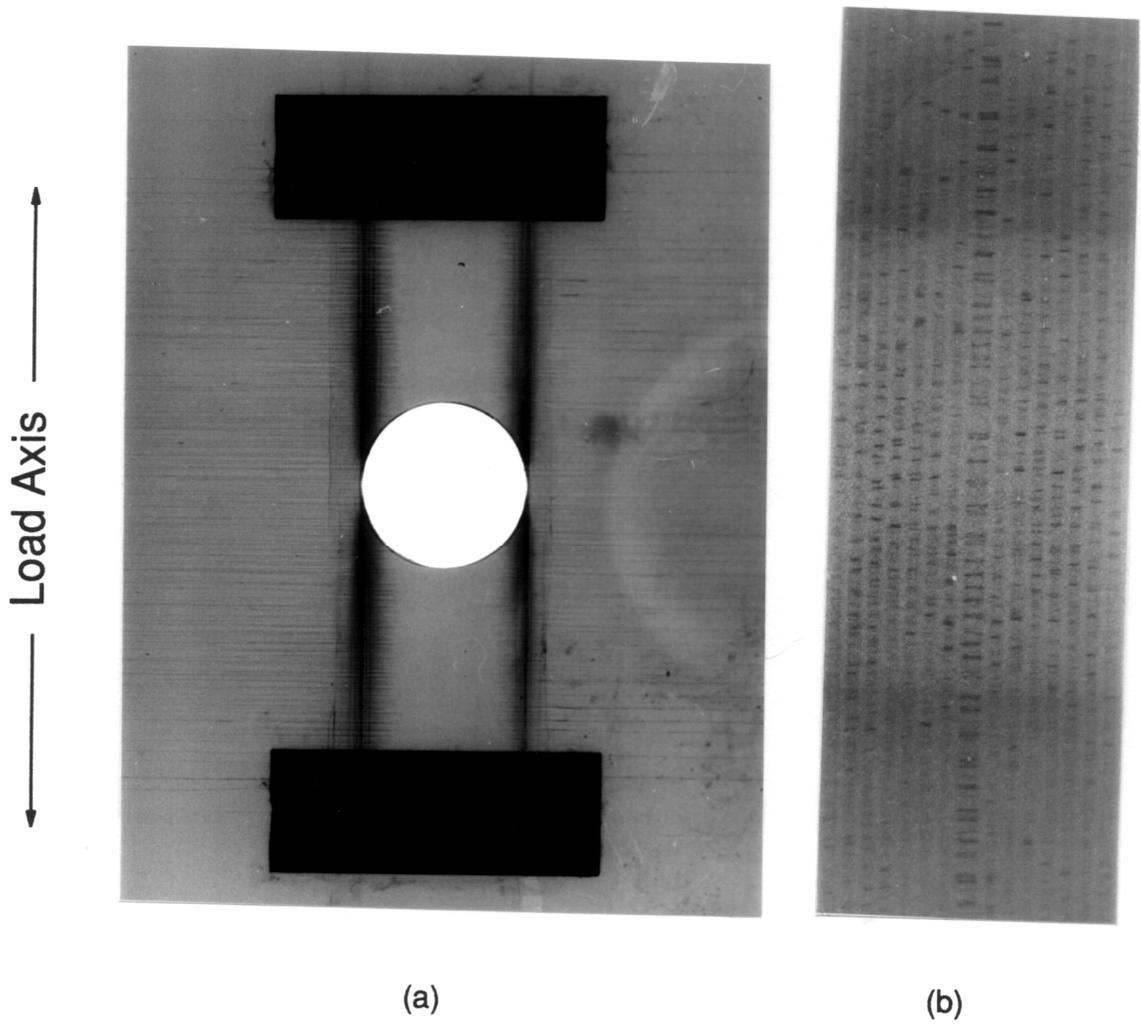
Figure 48. X-ray Radiograph of a 3SN Specimen after 6900 Cycles; a.) Front View, b.) Edge View.
