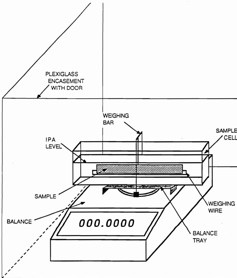
Figure 2. Set-up for Isopropyl Alcohol (IPA) Technique for Measuring Fiber Volume Fraction (taken from [56]).
