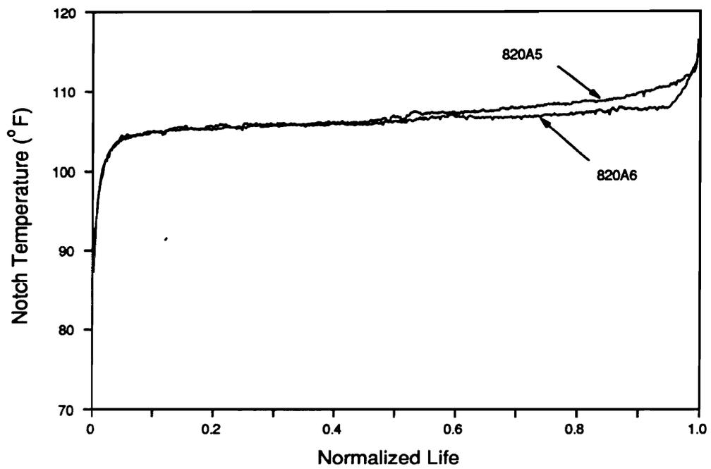
Figure 59. Plot of Notch Temperature versus Normalized Life for Two 820A Specimens; Max. Stress = 75% UCS; R = -1 at 10 Hz.
