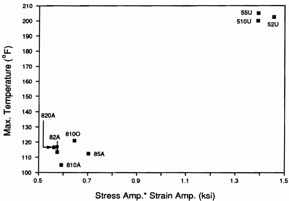
Figure 64. Plot of Maximum Specimen Temperature versus Specific Energy Term for McAir Materials; Max. Stress = 75% UCS; R = -1 at 10 Hz.
