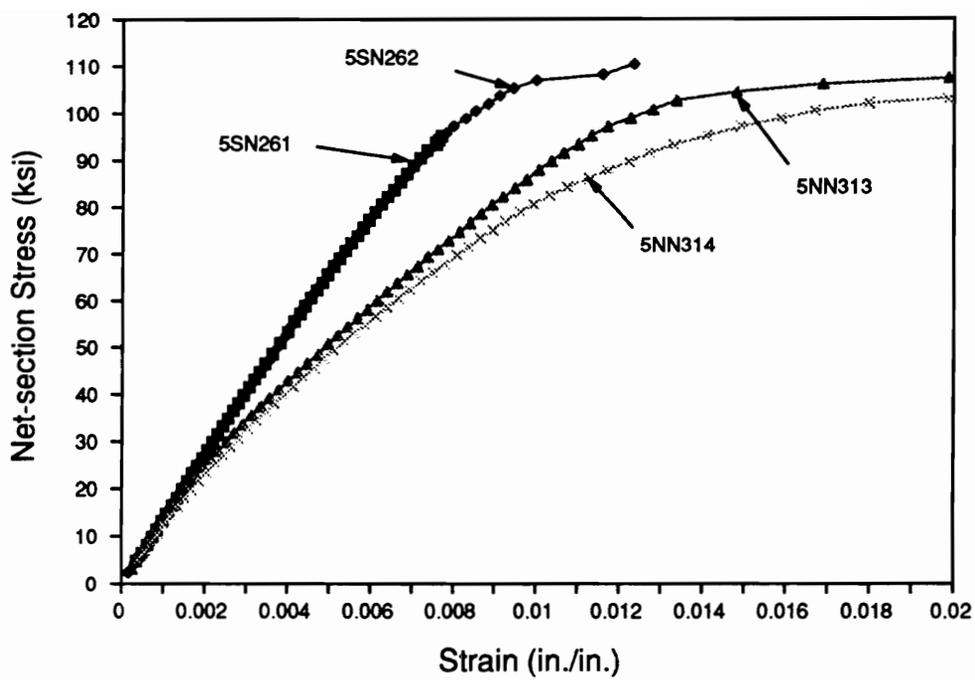
Figure 20. Net-Section Tensile Stress vs. Measured Strain for Two 5NN Specimens and Two 5SN Specimens.
