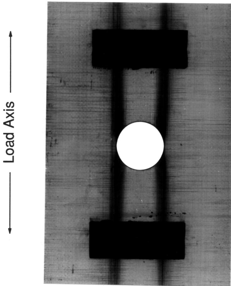
Figure 43. X-ray Radiograph of a 55U Specimen after 100,000 Cycles.
