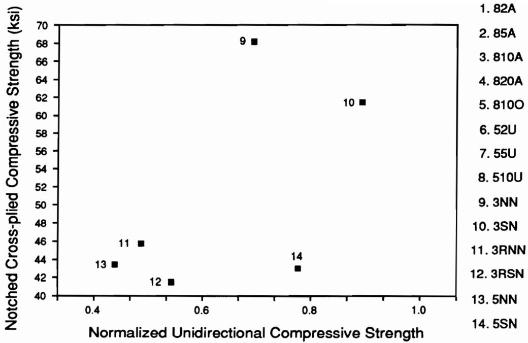
Figure 87. Notched Cross-plyed Compressive Strength versus Normalized Unidirectional Compressive Strength; Northrop Materials [39].
