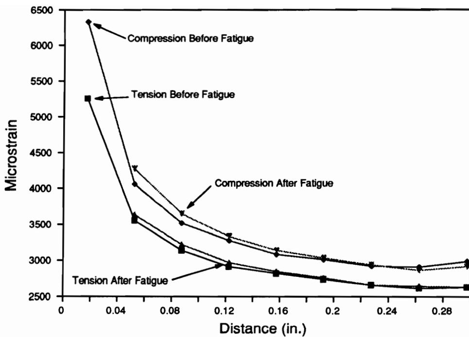
Figure 73. Longitudinal Strain Measurements as a Function of Distance from the Hole; 810A Before and After Fatigue.
