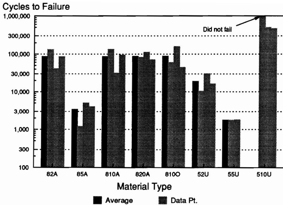
Figure 75. Cycles to Failure of the  $\pm 45^\circ$  McAir Specimens; Max. Stress = 24 ksi; R = 0.1 at 10Hz.
