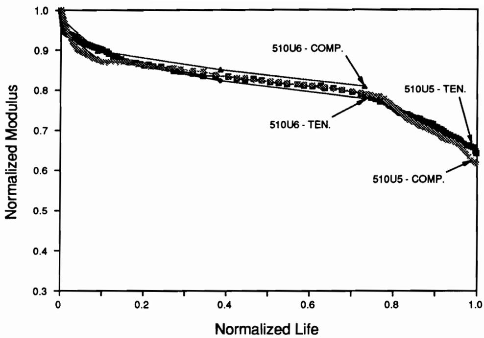
Figure 54. Plot of Normalized Modulus versus Normalized Life for Two 510U Specimens; Max. Stress = 75% UCS; R = -1 at 10 Hz.
